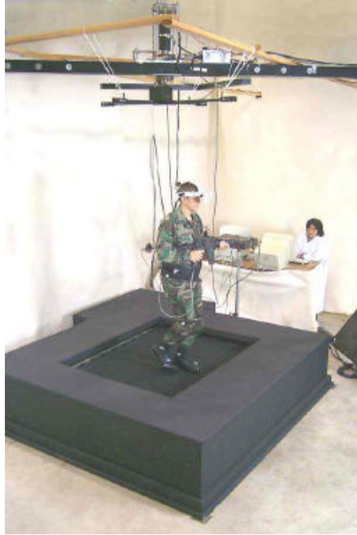
Figure 5. The Omni-Directional Treadmill with the sound enclosure.
