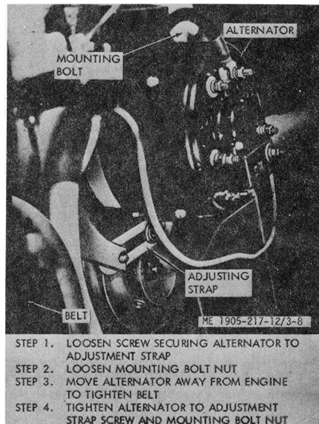
Figure 3-8. Adjusting alternator belts.
