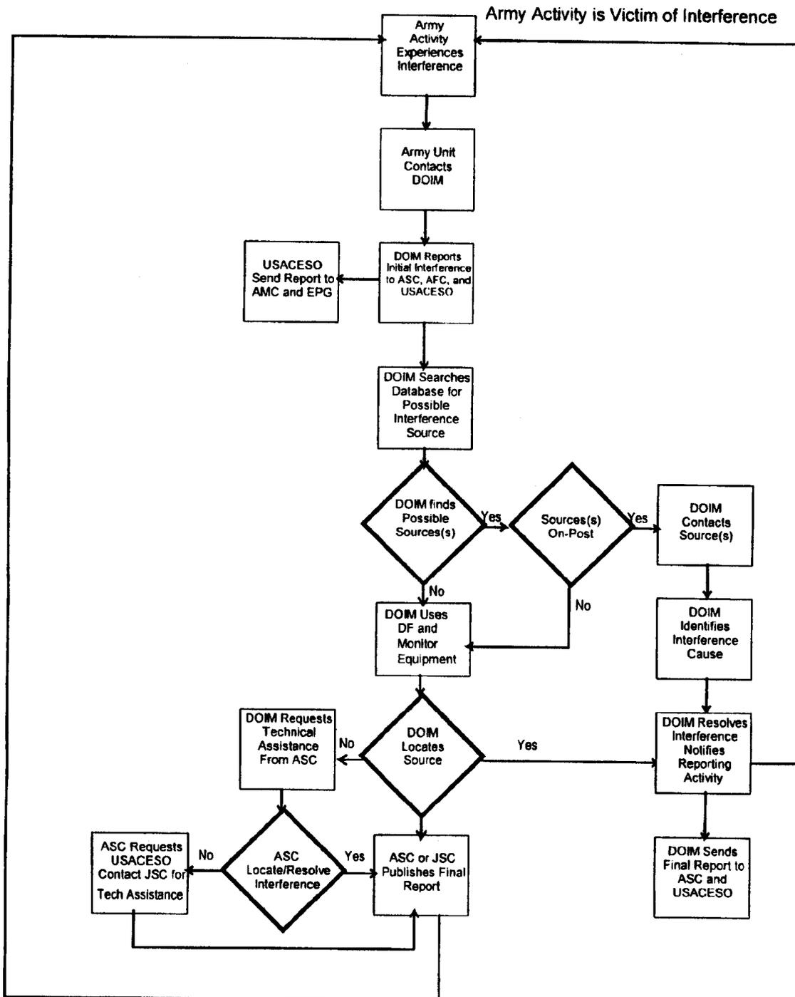
Figure C-4. Interference resolution (sustaining base environment (victim))
