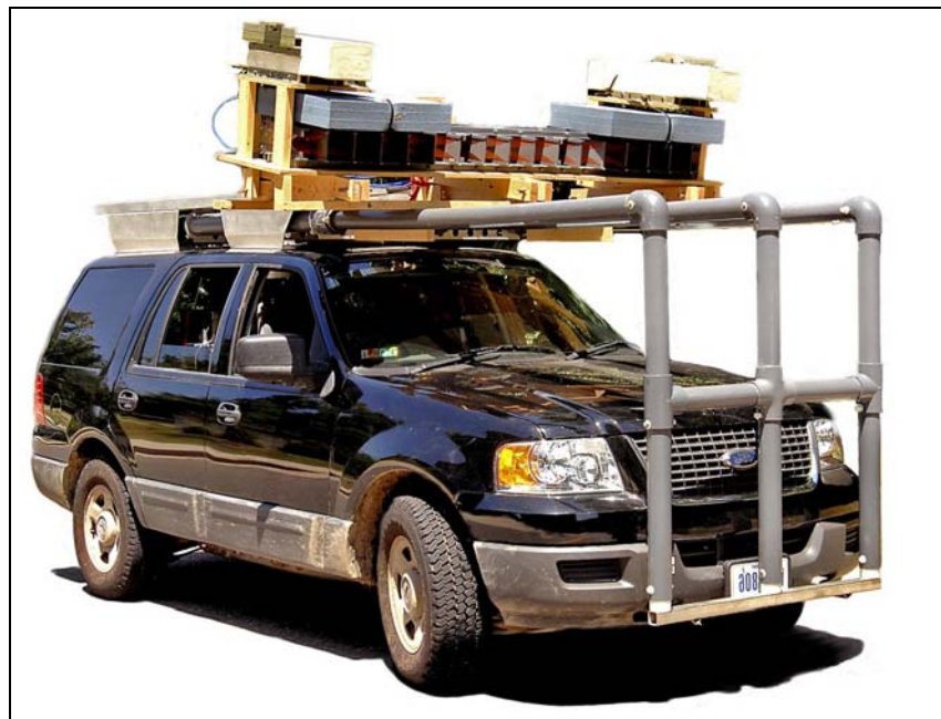
Figure 2. The ARL UWB SIRE radar system integrated onto the Ford Expedition.
