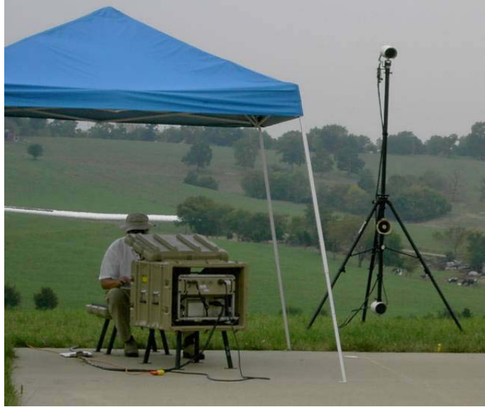
Figure 7. Sweep monitoring system (SMS).
