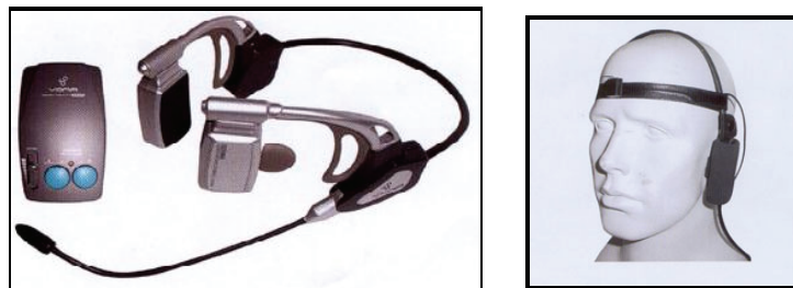
Figure 70. Two bone conduction devices from Duwomi Vonia: the EZ-3000S (left panel) and the BH-70MB (right panel). (The EZ-3000S is a hybrid system with bone conduction vibrators and an air conduction boom microphone, and the BH-70MB is a full bone conduction communication system with the bone conduction microphone located on the side of the head. Downloaded from http://www.vonia.co.za , September 20, 2006.)
