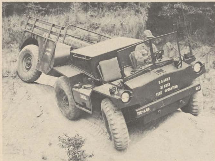
Figure 8—The Army's new 1 \frac{1}{4} -ton truck, the Gama Goat, a forward area tactical vehicle with unusual mobility.
