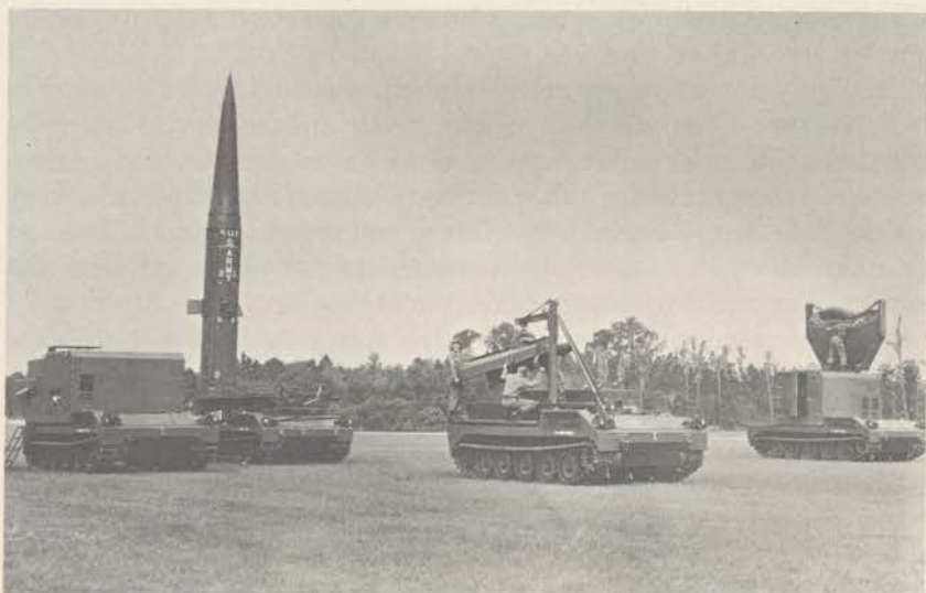
Figure 9. PERSHING missile with emplacement elements. At left, fire control and power supply; center, launch vehicle with aiming devices; and right, communications equipment showing antenna partially inflated.
