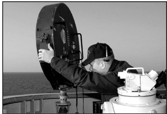
Figure 3. Ship's Serviceman 1st Class Scott D. Amberger aims a Long Range Acoustic Device at an incoming small craft off the starboard bridge wing of amphibious command ship USS Blue Ridge during a small boat attack drill. U.S. Navy photo.
