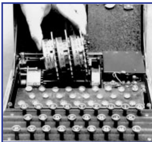
Fig. 5. Putting the rotors in the basket
