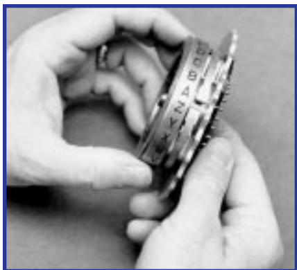
Fig. 3. Setting the notch ring
