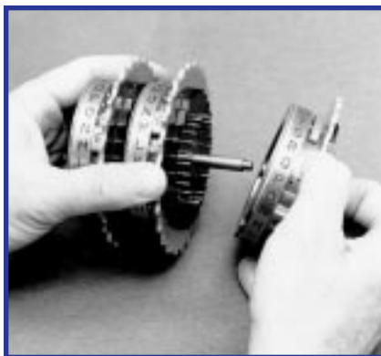
Fig. 4. Assembling the rotor set
