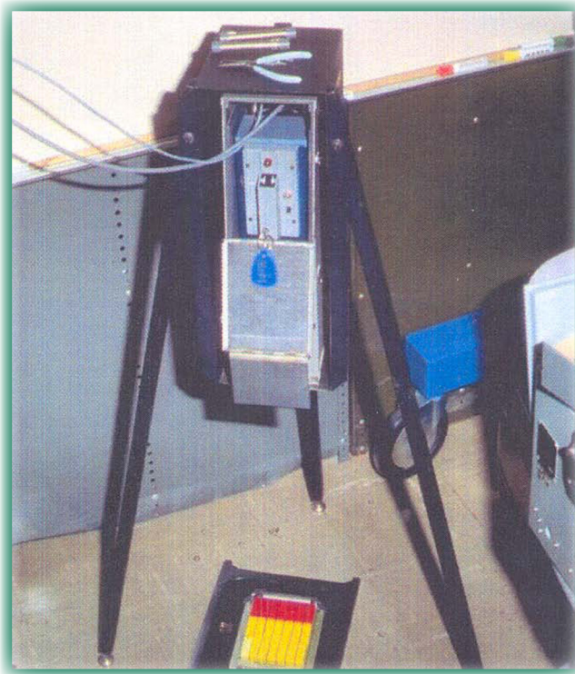
Fig. 2. Primary x-ray machine used in detecting equipment bugs. This was a portable machine about 8 inches deep, 6 inches wide, and 12-15 inches long. It was pointed at the floor when taking an x-ray; a sheet of x-ray film was placed under the item.
