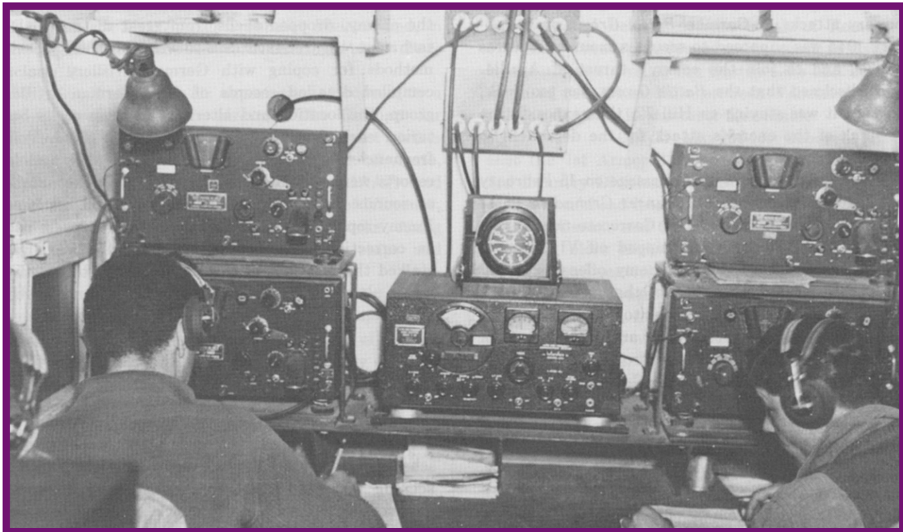
849th SIS Mediterranean Theater (3916th Signal Service Company) intercept van with double bank of receivers (BG 342 and BC 344) and the S-36 (VHF) in the middle (Photograph from the NSA History Collection)
