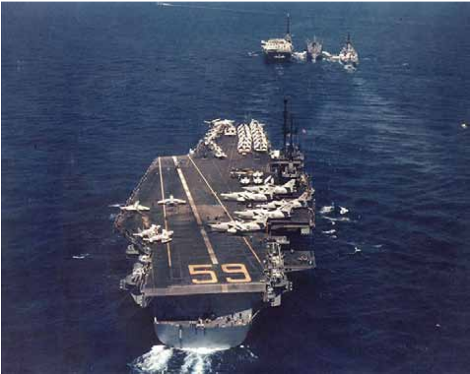
USS Forrestal (CVA-59) in Mediterranean Sea, April 1957. Note the angled deck and large size of the A3D Skywarriors (located on the starboard side of the ship, aft of the island superstructure) relative to the other aircraft.
