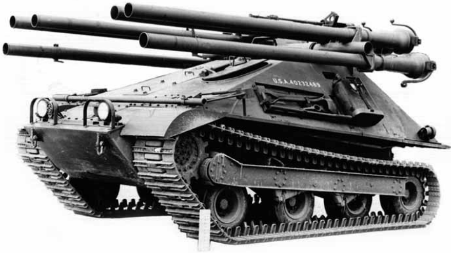
Pilot Ontos test vehicle mounting six 105-mm. recoilless rifles, 1952. (Note: In 1953, Ontos vehicles were modified to mount six 106-mm. recoilless rifles.)
