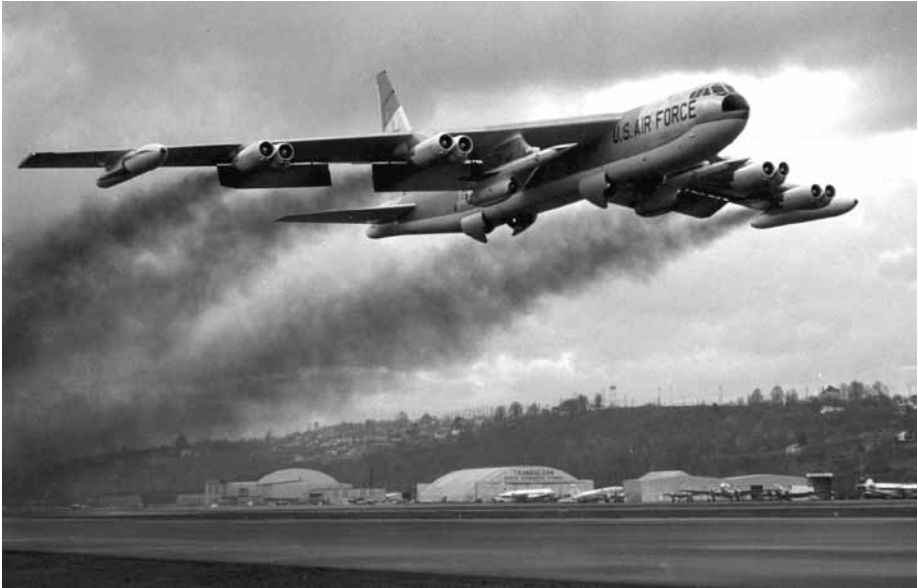
B-52F Stratofortress with Hound Dog air-to-surface missiles loaded on the inboard wing pylons. Courtesy, National Museum of the U.S. Air Force.
