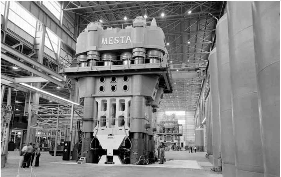
This giant hydraulic forging press—five stories high, weighing 6,000 tons, and capable of exerting 50,000 tons of force—was built by Mesta and housed in a 12-acre facility constructed and operated for the Air Force by Alcoa at its plant in Cleveland, Ohio.
