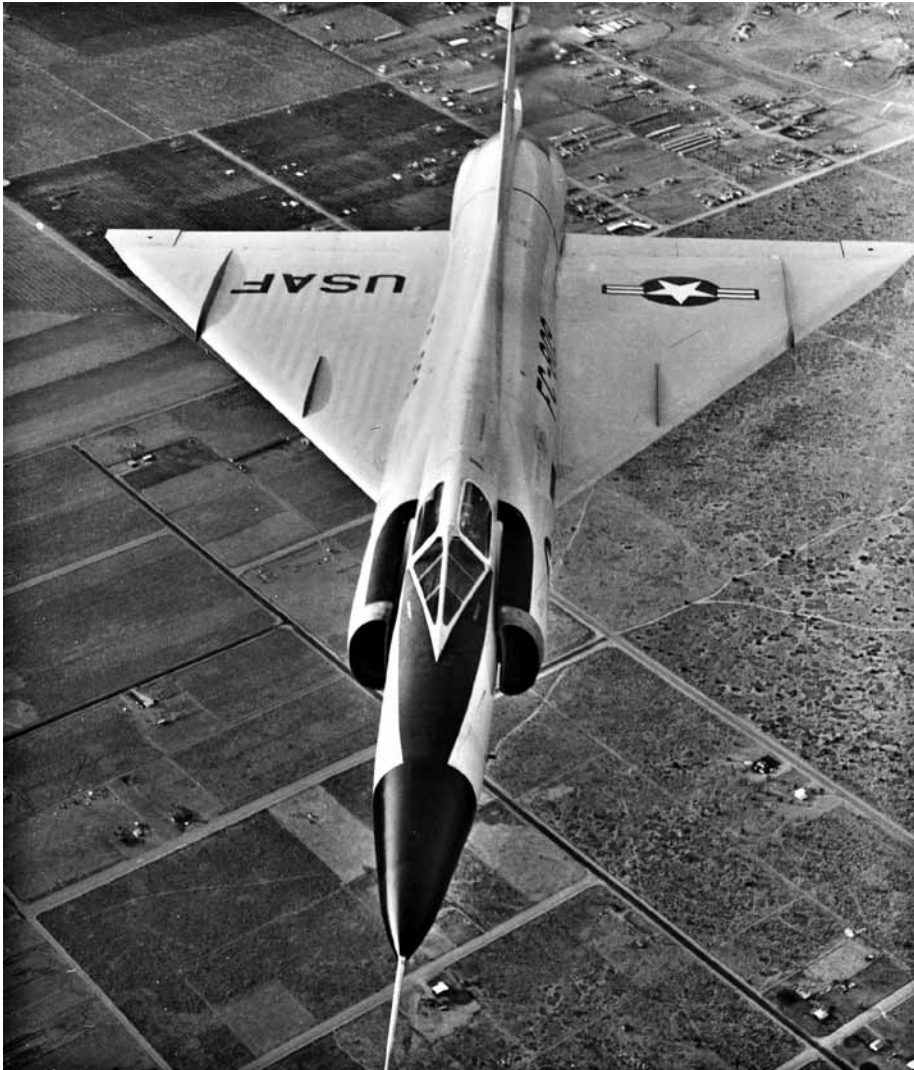
F-102A Delta Dagger in flight. Note indented fuselage.
