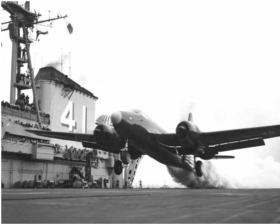
P2V-3C Neptune, with Secretary of Defense Johnson on board, in rocket-assisted take off from the carrier USS Midway (CVB-41), 26 September 1949. Note proximity of the aircraft's right wingtip to the ship's island superstructure.
