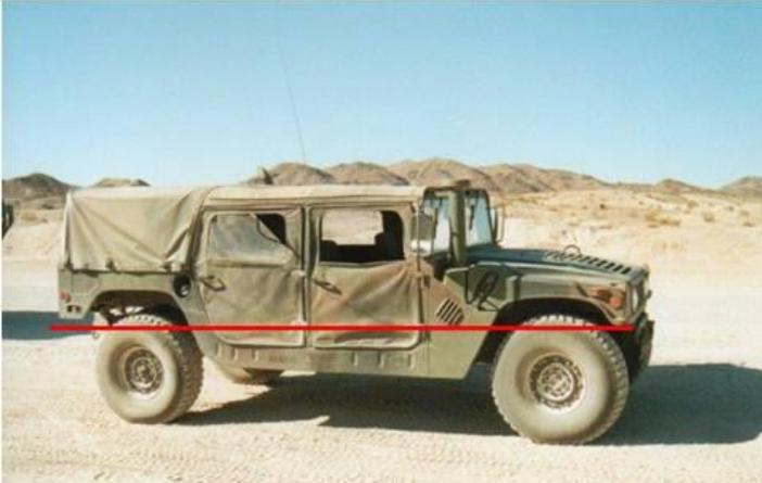
**Maximum fording depth:** 60 inches with deep water fording kit installed.
