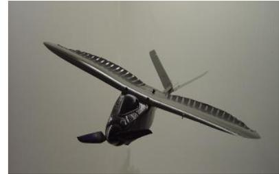
Platoon, squad, and fire team elements employed the TACMAV for real-time reconnaissance and surveillance support. Operational feedback was either neutral or negative. Soldiers complained about the poor image and lack of stability, grid coordinates, and IR capability. Use of the TACMAV is very dependent on weather conditions (wind). Following REF involvement, newer configurations made by ARA included an IR camera and longer flight time.
