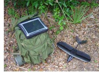
The TACMAV uses flexible wings, which fold around its fuselage, allowing the entire UAV to be stored in a 22-inch long, 5-inch diameter tube and carried in the user’s backpack. The TACMAV uses a payload pod containing two color Charge Couple Device cameras and a video transmitter. The user can select a forward- or side-looking camera. The GCU uses the standard Air Force Portable Flight Planning System interface for mission planning, in-flight updates, and manual control.
