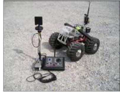
**Background:** Joint Services EOD BomBot is a low-cost, expendable robot for IED neutralization. It is a small, fast, off-road vehicle equipped with a small explosive charge delivery system, and it is remotely controlled using either video feedback or simply LOS radio. In employment, a BomBot is driven to an IED, and a C4 explosive charge is dropped from the vehicle, which is then driven away, if practical, before the charge is remotely detonated.
