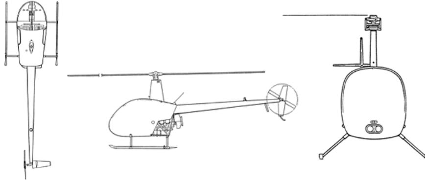
**Background:** Maverick is an unmanned version of the Robinson R22 helicopter. Frontier modified it in 1999 to serve as a testbed for developing the control logic for their DARPA A-160 unmanned aircraft effort. Subsequently, the Navy decided to acquire four Mavericks in 2003.
