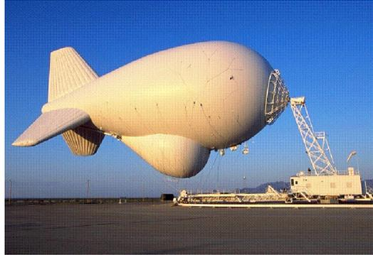
digitized and fed to the various users. Airborne time is generally limited by the weather to 60 percent operational availability; notwithstanding weather, aerostat and equipment availability averages more than 98 percent systemwide. For security and safety reasons, the airspace around Air Force aerostat sites is restricted for a radius of at least two to three statute miles and an altitude up to 15,000 feet.
