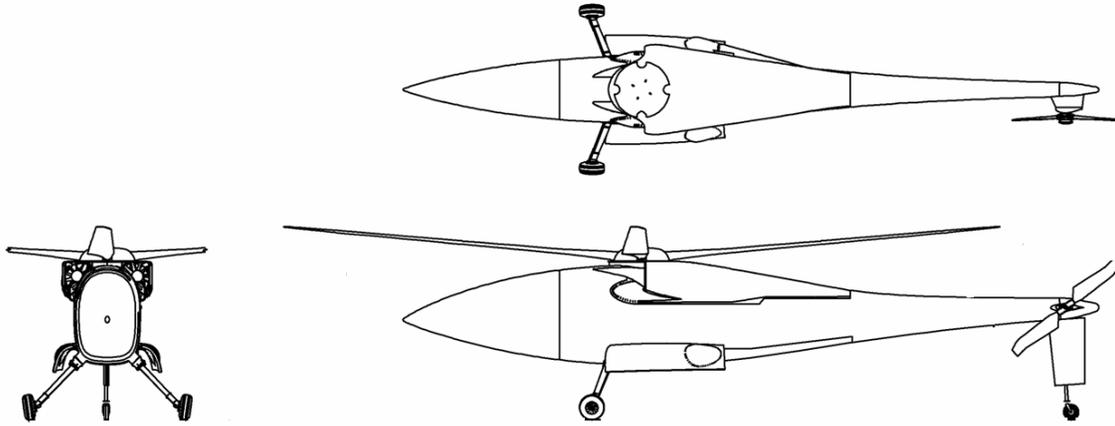
**Background:** A160 Hummingbird is a long endurance VTOL UAV using a revolutionary Optimum Speed Rotor (OSR), low drag configuration, and high fuel fraction to enable much longer endurance than conventional helicopters. In addition, it uses a stiff-in-plane rotor to enable fast reaction to gust loads.
