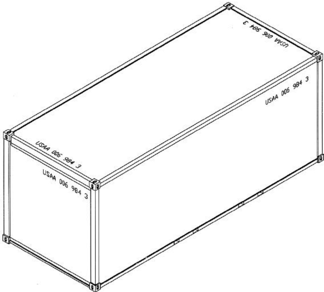
**Figure 603-2. Typical Horizontal Layout of ISO Identification Markings**
