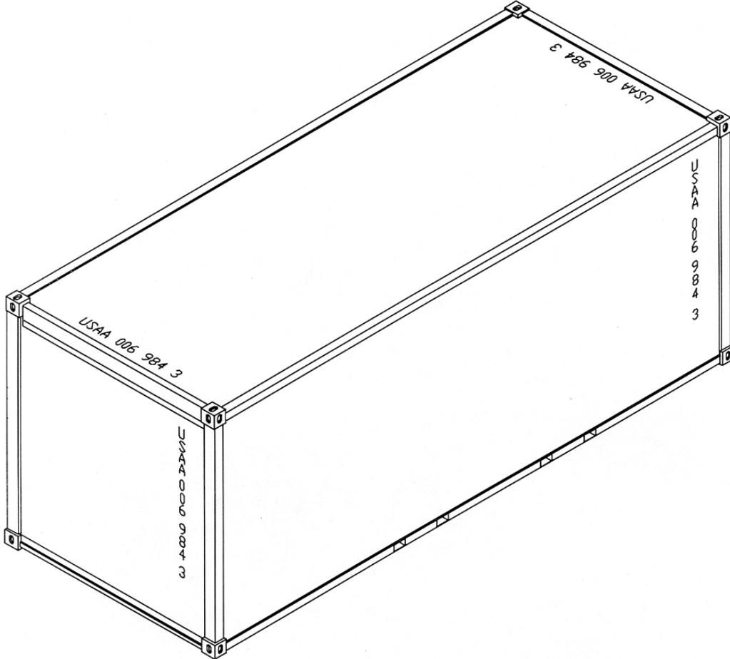
**Figure 603-3. Typical Vertical Layout of ISO Identification Markings**
