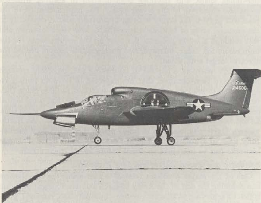
Figure 11. The new XV-5A jet V/STOL aircraft shown in vertical takeoff configuration tests at Edwards AFB, Mass.
