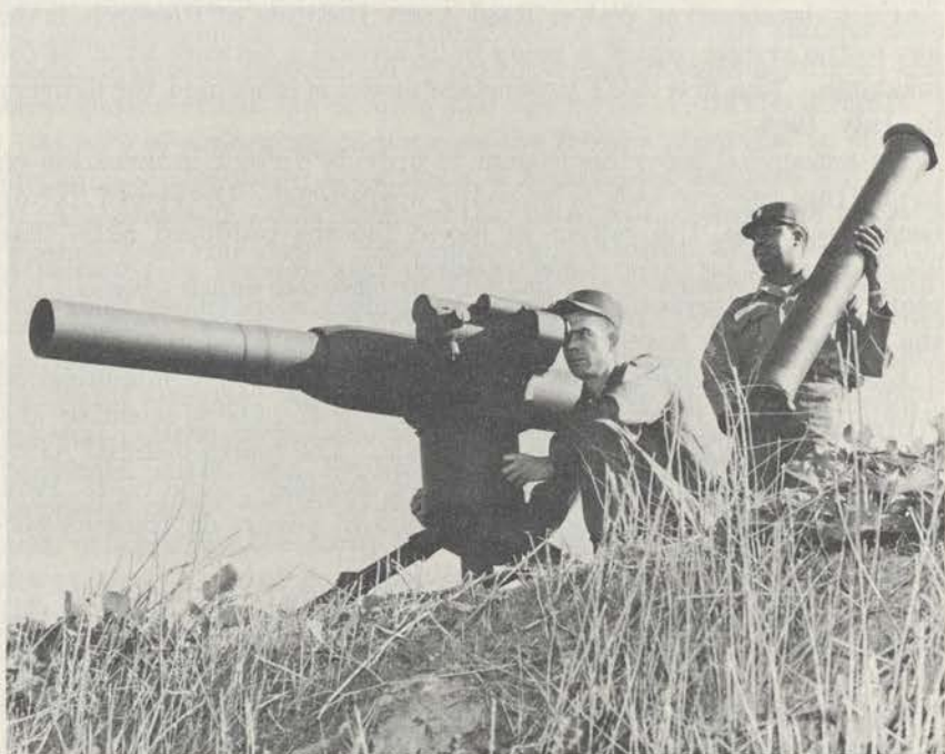
Figure 12. TOW, the lightweight new tank-killer being developed for the Army, has demonstrated an exceptionally high degree of accuracy and good launching characteristics in fully guided test missile firings.
