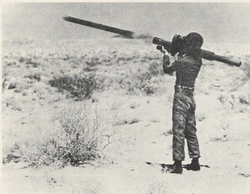
Figure 13. REDEYE, the world's smallest guided missile, is shown here just after clearing the shoulder launcher.
