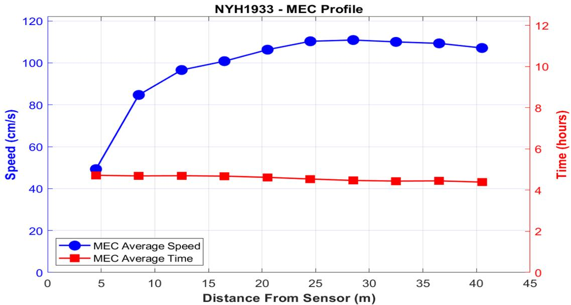
Figure 5-31. NYH1933 MEC timing (GI – red squares) and speed (blue circles) by distance bin.
