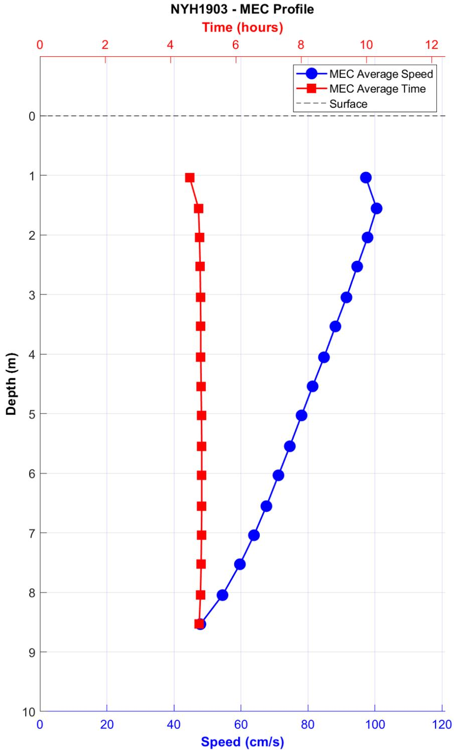
**Figure 5-6** NYH1903 MEC timing (GI – red squares) and speed (blue circles) by depth bin. Bin 1 is the deepest bin observed at approximately 8.5 m below MLLW, and the top-most good bin is bin 16 (1.5 m below MLLW).
