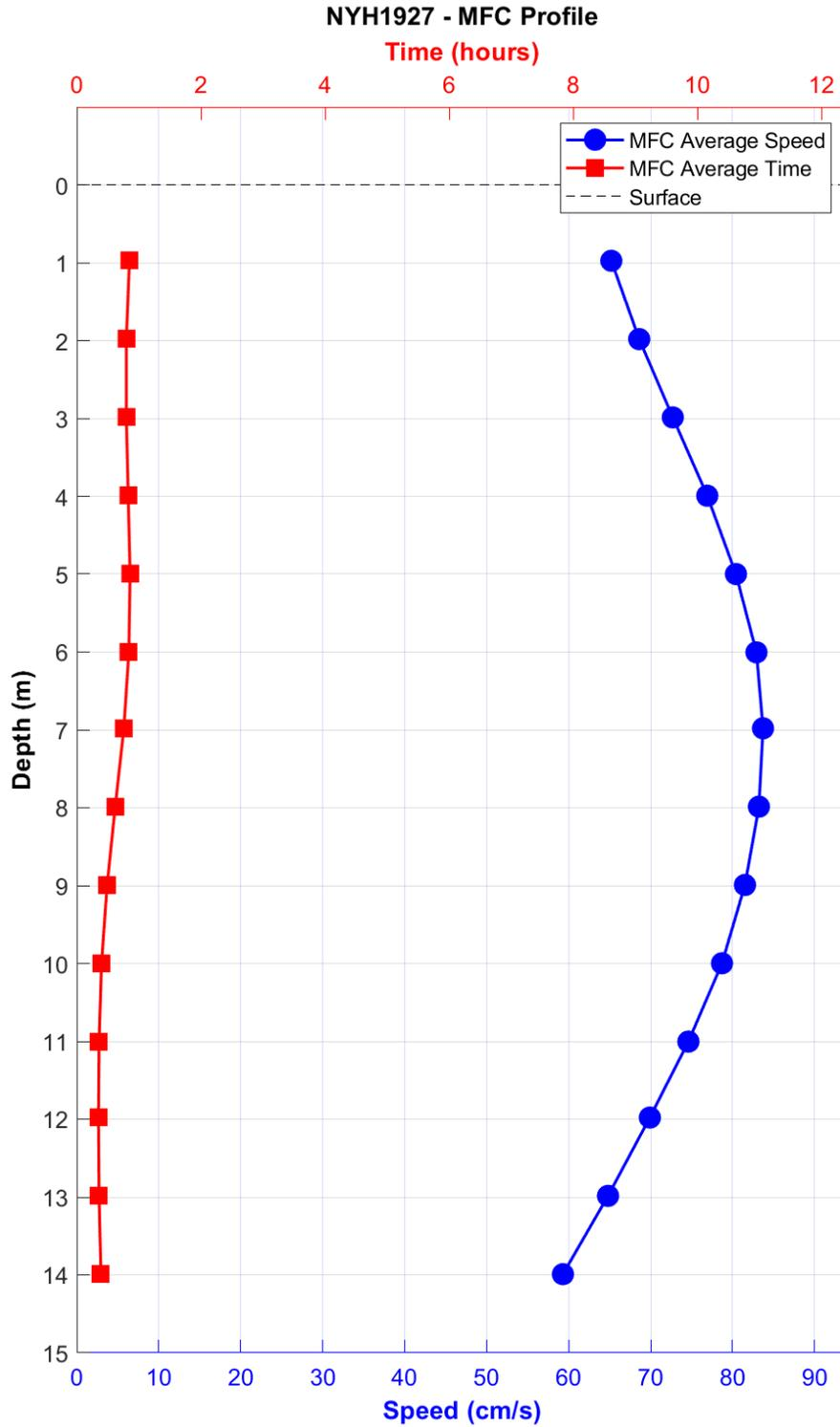
**Figure 5-20.** NYH1927 MFC timing (GI - in red squares) and speed (blue circles) by depth bin. Bin 1 is the deepest bin observed at approximately 13.0 m below MLLW, and the top-most good bin is bin 14 (1.0 m below MLLW).
