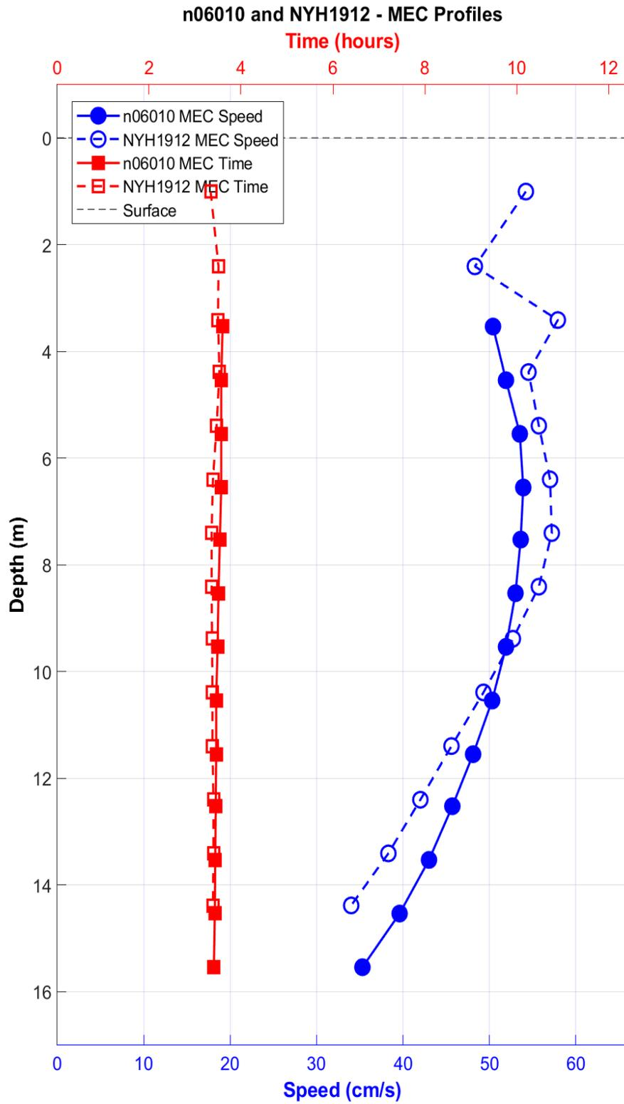
**Figure 5-33.** MEC comparison between stations NYH1912 and n06010 showing similar timing (red squares) but more speed shear for NYH1912.
