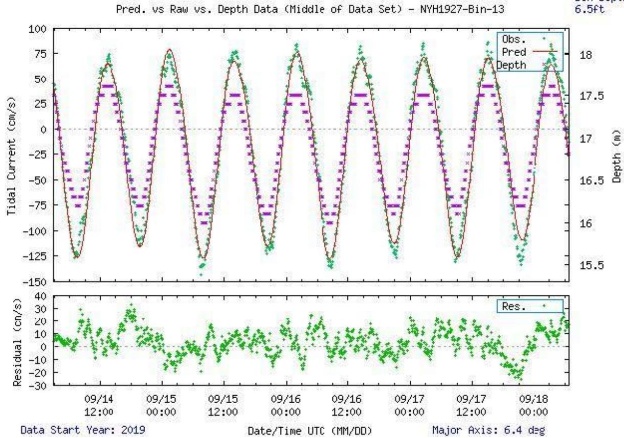
**Figure 5-18.** Comparison of observed major axis velocity data (green points) to predicted tidal velocity along the major axis for station NYH1927. Pressure sensor data is included to show the phase alignment of the tide and current for this location. The lower figure shows the non-tidal residual, the difference between the predicted and observed velocity from the upper panel.
