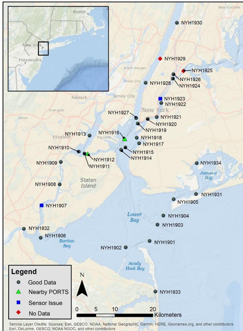
**Figure 1-1.** All stations deployed for the NYH survey of 2019. Stations where no data were collected are indicated by a red diamond. Stations where data were collected but there was an issue with the compass matrix are indicated by a blue square. Stations where a nearby PORTS® station was used in lieu of survey data are indicated by a green triangle. All other stations collected good data and are indicated by a gray dot.
