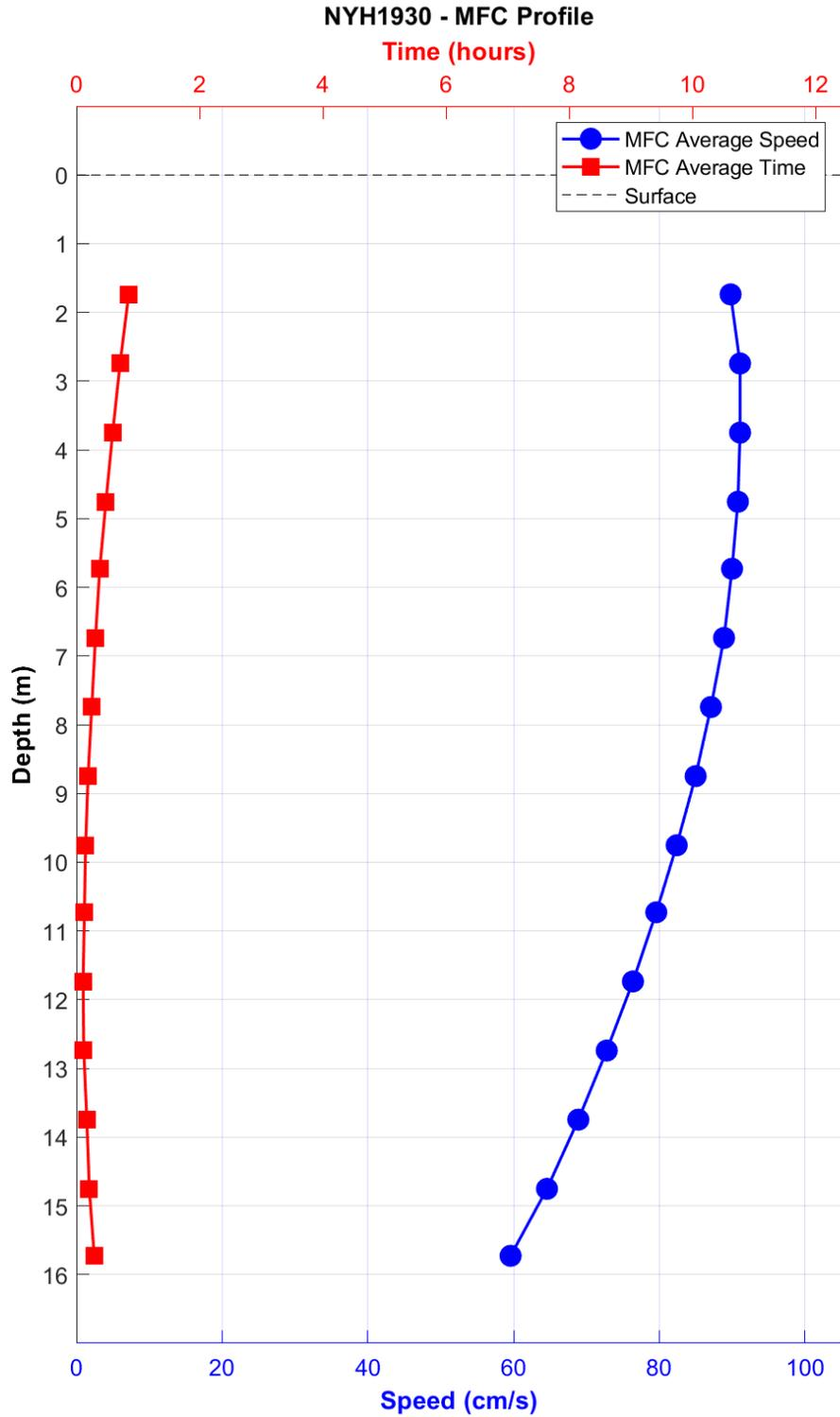
**Figure 5-25.** NYH1930 MFC timing (GI - in red squares) and speed (blue circles) by depth bin. Bin 1 is the deepest bin observed at approximately 15.7 m below MLLW, and the top-most good bin is bin 15 (1.7 m below MLLW).
