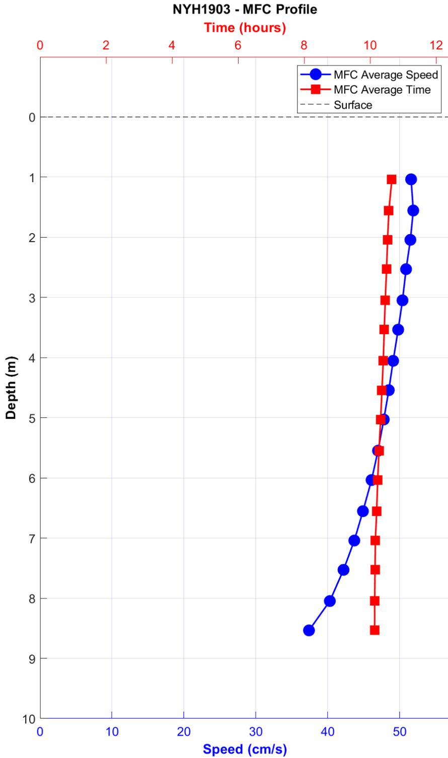
**Figure 5-5.** NYH1903 MFC timing (GI - in red squares) and speed (blue circles) by depth bin. Bin 1 is the deepest bin observed at approximately 8.5 m below MLLW, and the top-most good bin is bin 16 (1.5 m below MLLW).
