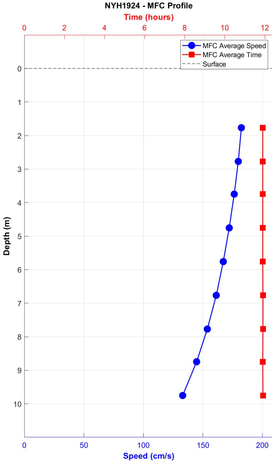
**Figure 5-15.** NYH1924 MFC timing (GI - in red squares) and speed (blue circles) by depth bin. Bin 1 is the deepest bin observed at approximately 9.8 m below MLLW, and the top-most good bin is bin 9 (1.8 m below MLLW).
