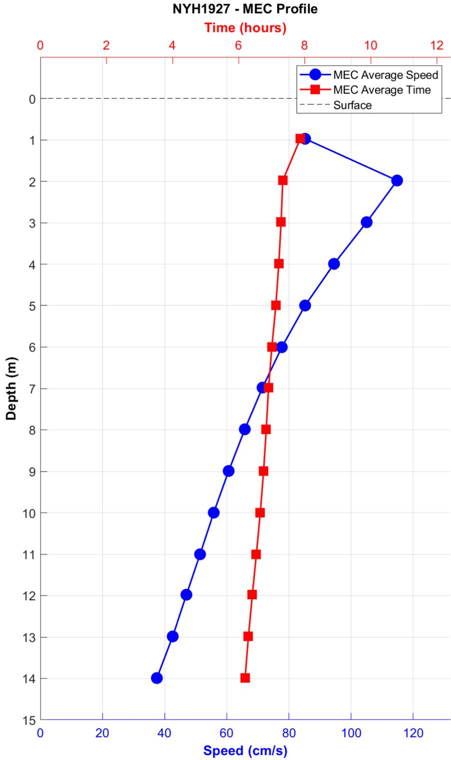
**Figure 5-21.** NYH1927 MEC timing (GI – red squares) and speed (blue circles) by depth bin. Bin 1 is the deepest bin observed at approximately 13.0 m below MLLW, and the top-most good bin is bin 14 (1.0 m below MLLW).
