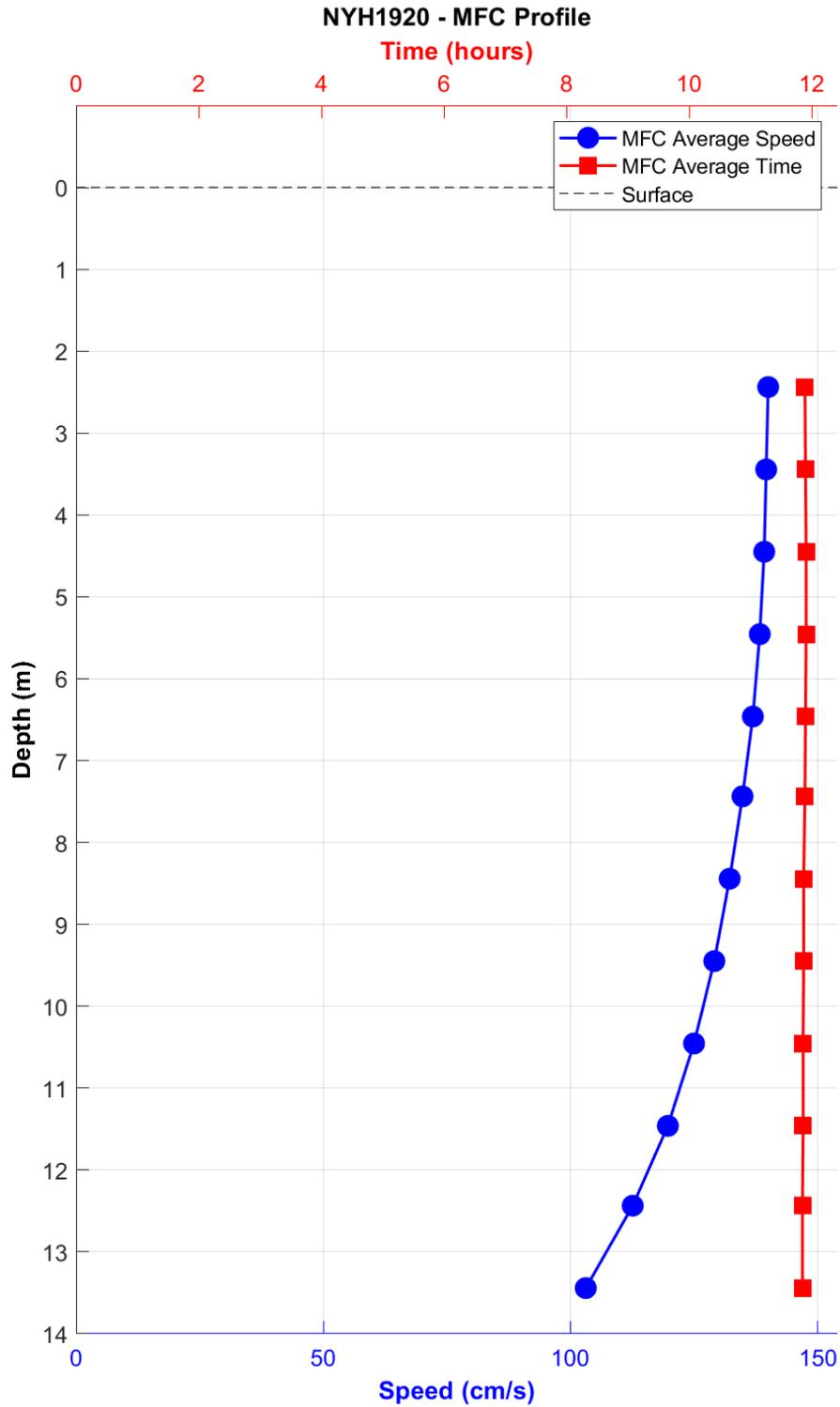
**Figure 5-10.** NYH1920 MFC timing (GI - in red squares) and speed (blue circles) by depth bin. Bin 1 is the deepest bin observed at approximately 13.5 m below MLLW, and the top-most good bin is bin 12 (2.5 m below MLLW).
