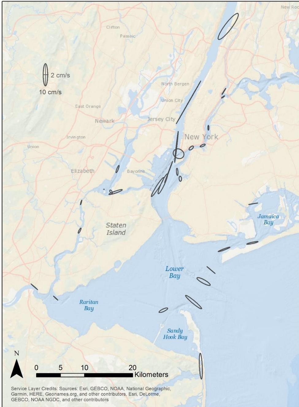
**Figure 6-5.** K<sub>1</sub> tidal ellipses for the entire study region. Note that these are on a different scale than M<sub>2</sub> in order to see the ellipses. These data are at about 1/8 the scale of the M<sub>2</sub> data.
