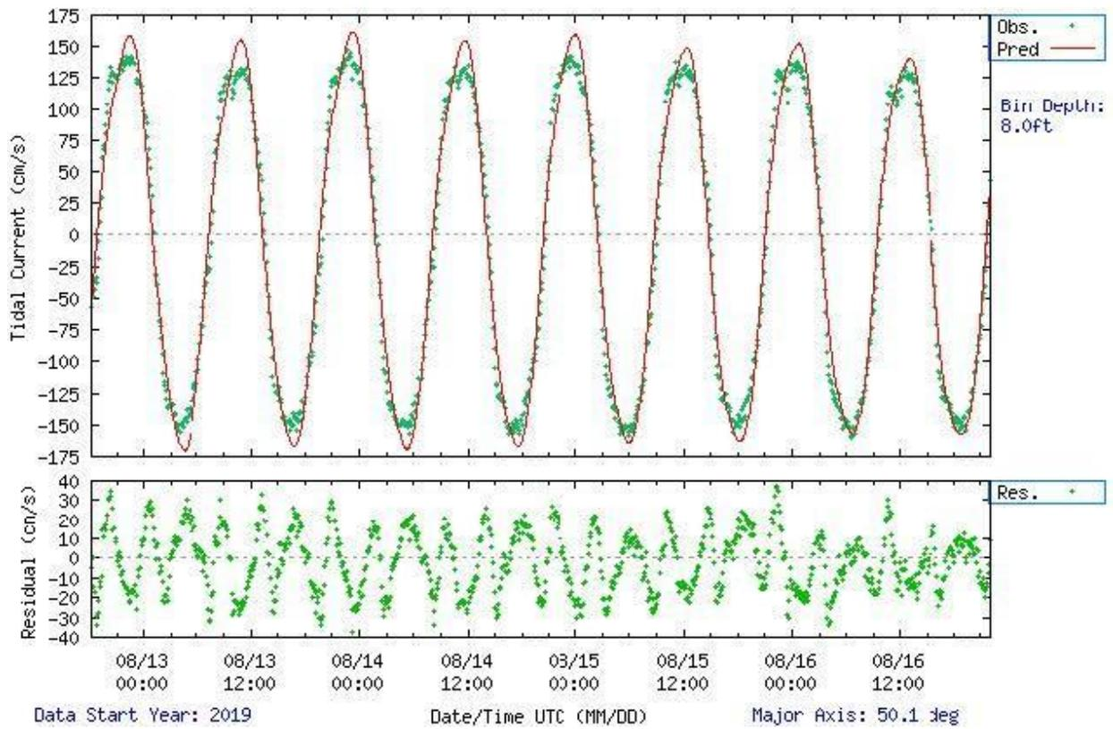
**Figure 5-8.** Comparison of observed major axis velocity data (green points) to predicted tidal velocity along the major axis for station NYH1920. The lower figure shows the non-tidal residual, the difference between the predicted and observed velocity from the upper panel.
