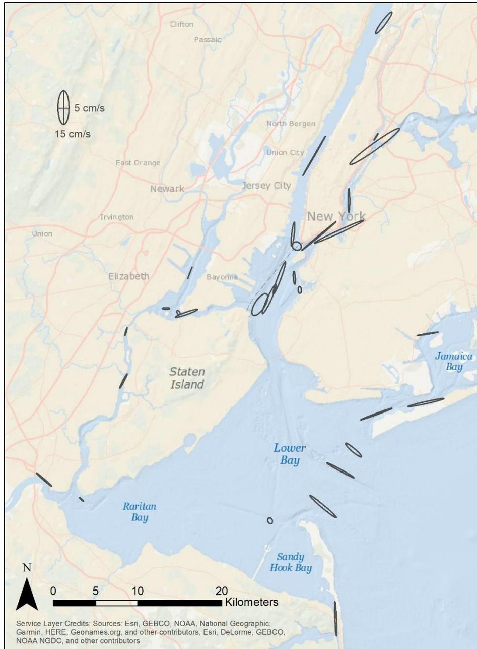
**Figure 6-3.**  $S_2$  tidal ellipses for the entire study region. Note that these are on a different scale than  $M_2$  in order to see the ellipses. These data are at about 1/5 the scale of the  $M_2$  data.
