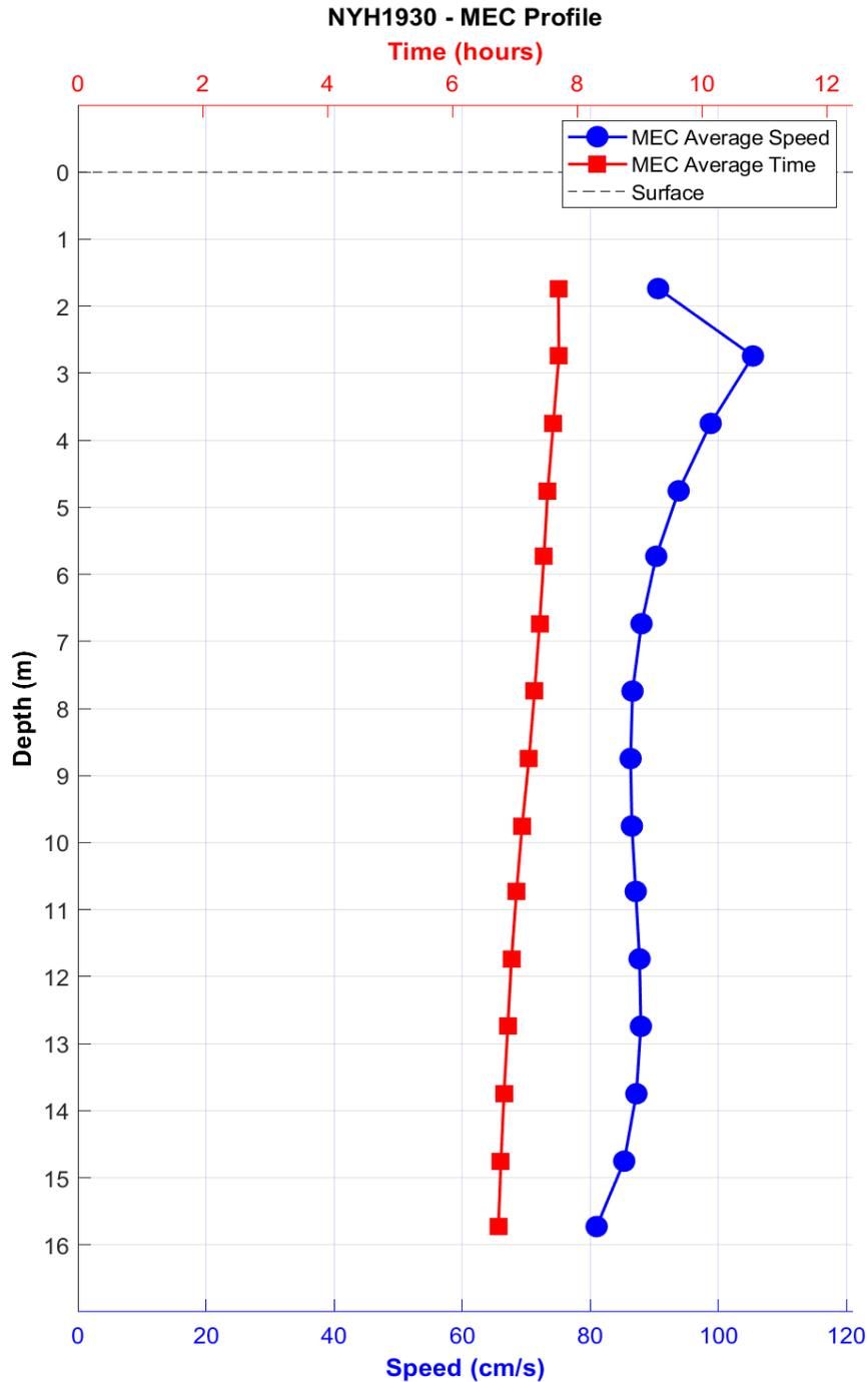
**Figure 5-26.** NYH1930 MEC timing (GI – red squares) and speed (blue circles) by depth bin. Bin 1 is the deepest bin observed at approximately 15.7 m below MLLW, and the top-most good bin is bin 15 (1.7 m below MLLW).
