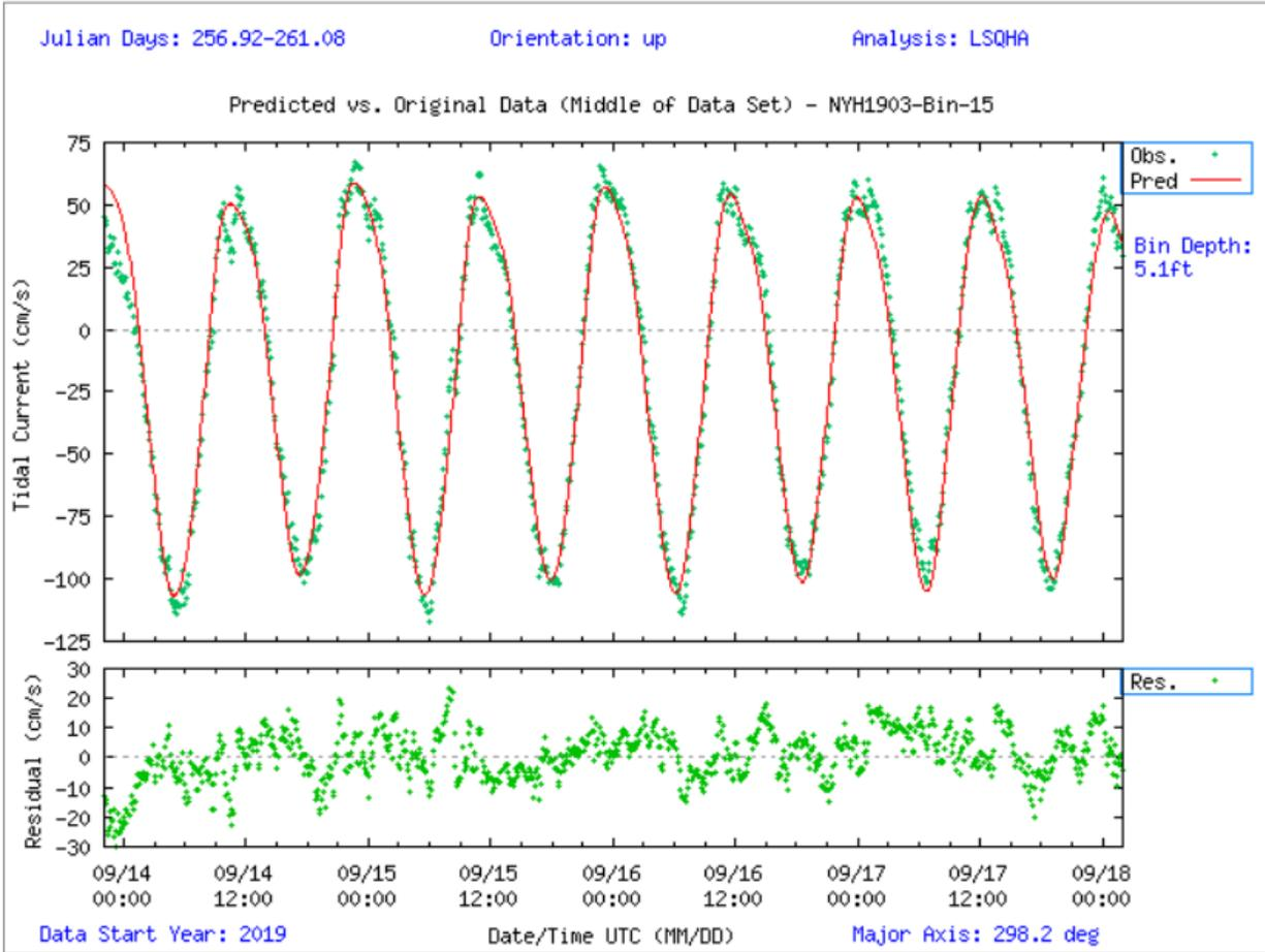
**Figure 5-3.** Comparison of observed major axis velocity data (green points) to predicted tidal velocity along the major axis for station NYH1903. The lower figure shows the non-tidal residual, the difference between the predicted and observed velocity from the upper prediction bin.
