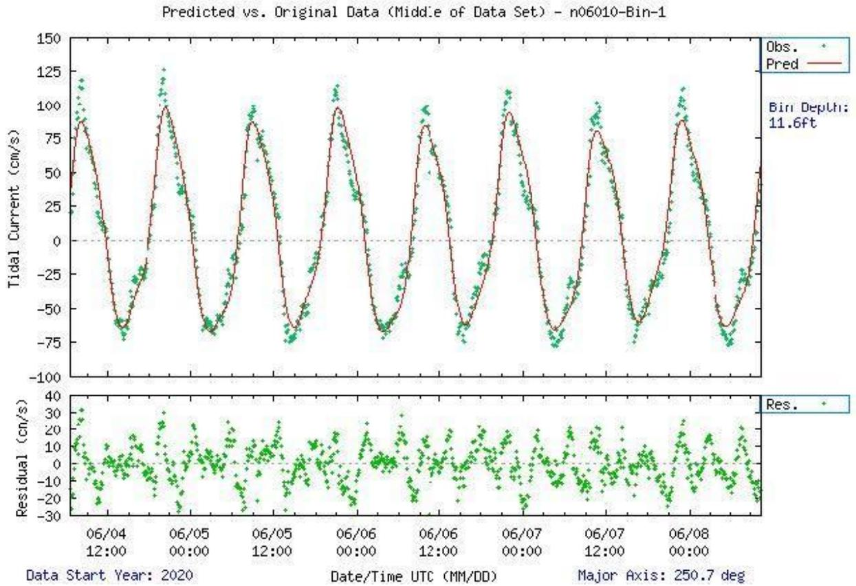
**Figure 5-35.** Comparison of observed major axis velocity data (green points) to predicted tidal velocity along the major axis for station n06010. The lower figure shows the non-tidal residual, the difference between the predicted and observed velocity from the upper panel.
