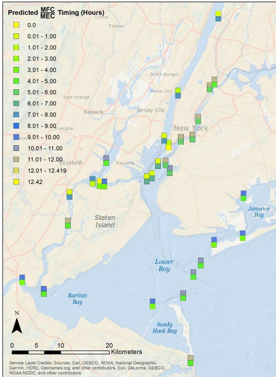
**Figure 6-7** GI timing of maximum flood (top) and ebb (bottom) at all stations in the survey. Note that the colors represent hours from 0 to 12.42 with the end interval limits having the same colors to represent the cyclical tides.
