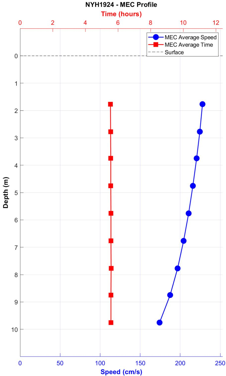
**Figure 5-16.** NYH1924 MEC timing (GI – red squares) and speed (blue circles) by depth bin. Bin 1 is the deepest bin observed at approximately 9.8 m below MLLW, and the top-most good bin is bin 9 (1.8 m below MLLW).
