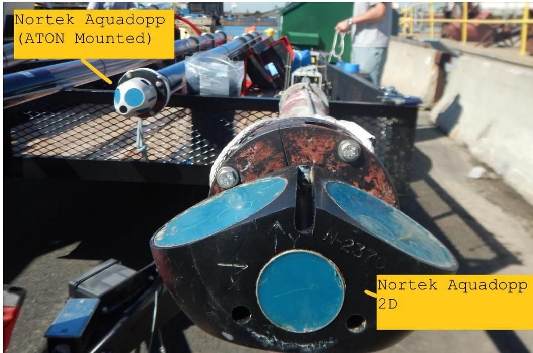
**Figure 3-5.** Bottom of side-looking Nortek AqD 2D ready for installation. View is looking up the pole to the mount. ATON-mounted, downward-facing Aquadopp is pictured to the left of the side-looker, mounted in a tube attached to a Clamparatus and ready for installation.
