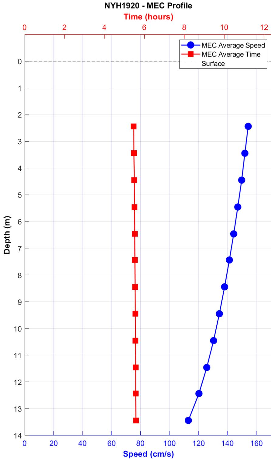
**Figure 5-11.** NYH1920 MEC timing (GI – red squares) and speed (blue circles) by depth bin. Bin 1 is the deepest bin observed at approximately 13.5 m below MLLW, and the top-most good bin is bin 12 (2.5 m below MLLW).
