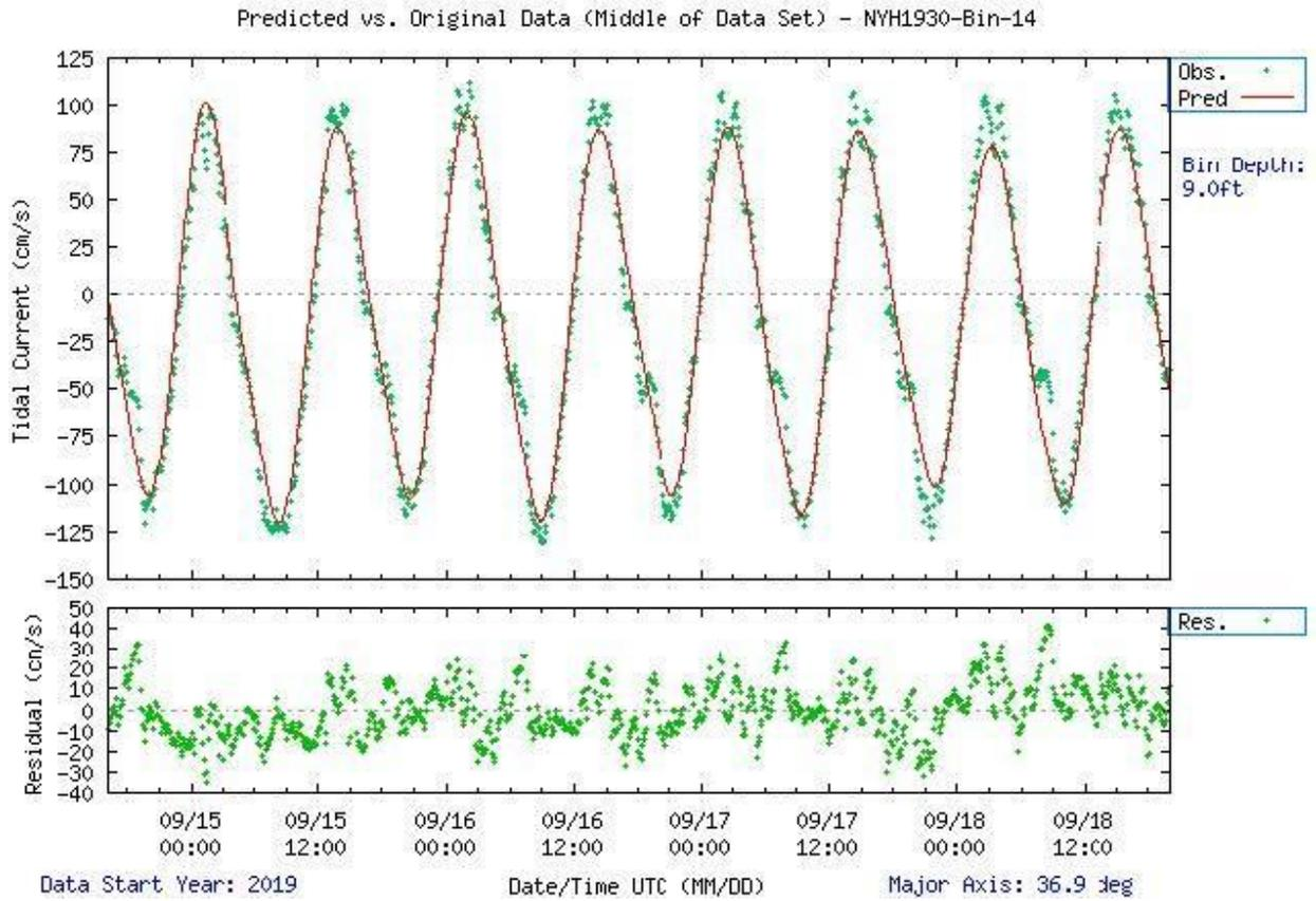
**Figure 5-23.** Comparison of observed major axis velocity data (green points) to predicted tidal velocity along the major axis for station NYH1930. The lower figure shows the non-tidal residual, the difference between the predicted and observed velocity from the upper panel.
