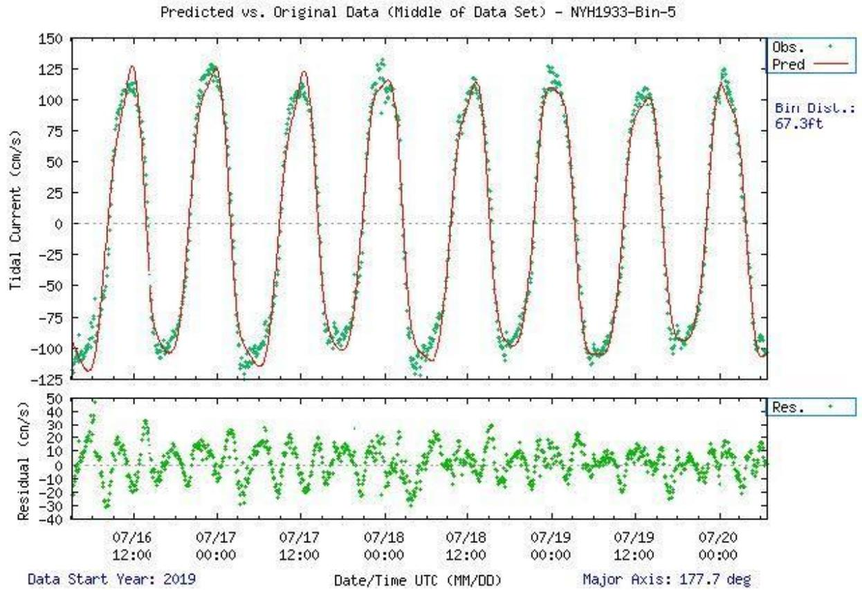
**Figure 5-28.** Comparison of observed major axis velocity data (green points) to predicted tidal velocity along the major axis for station NYH1933. The lower figure shows the non-tidal residual, the difference between the predicted and observed velocity from the upper panel.
