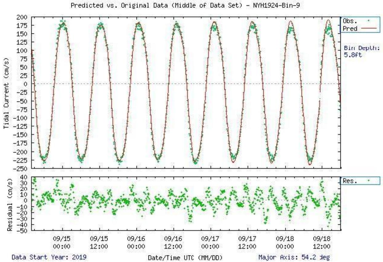
**Figure 5-13.** Comparison of observed major axis velocity data (green points) to predicted tidal velocity along the major axis for station NYH1924. The lower figure shows the non-tidal residual, the difference between the predicted and observed velocity from the upper panel.
