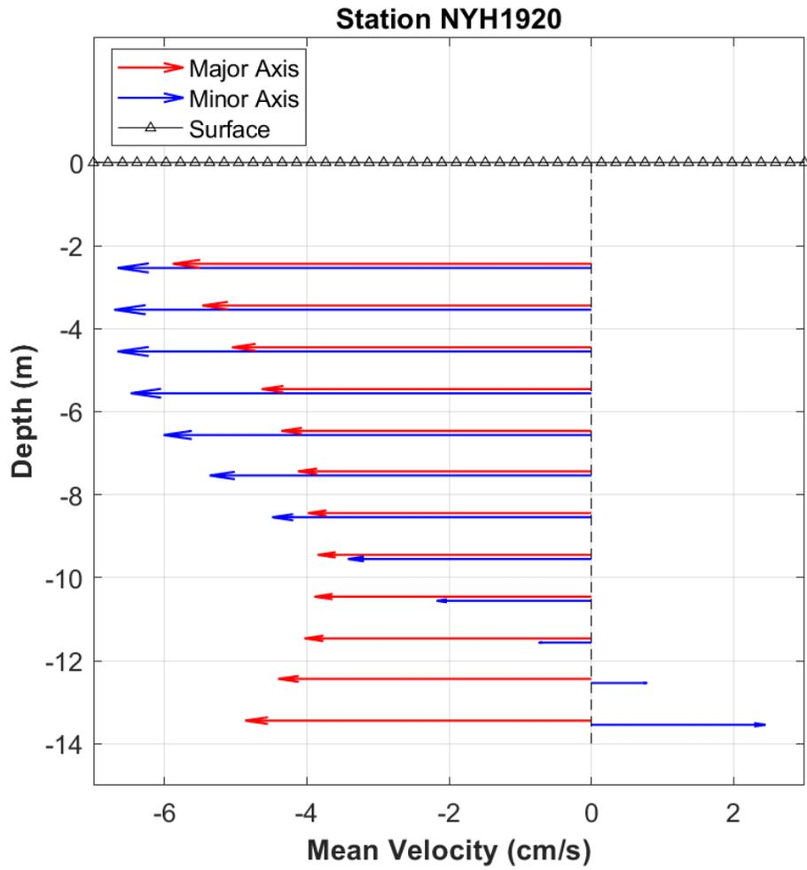
**Figure 5-9.** NYH1920 mean velocity profile by depth. Only depths that passed quality control criteria are shown. This station was configured to collect 1.0 m bins.
