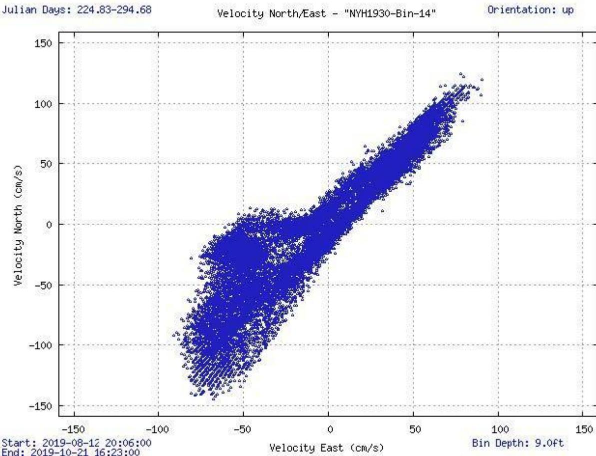
**Figure 5-22** Scatter plot of north-versus-east velocity for station NYH1930 at the near-surface bin, bin 14 at 2.7 m below MLLW. The westward lobe on the ebb is likely the influence of Spuyten Duyvil.
