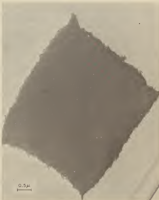
Fig.8 Carbon replica of the surface of a pseudopolyhedral aggregate of polypropylene revealing an apparently intermeshed fibrillar structure. The sides of the aggregate with respect to this electron micrograph coincide in orientation with those of the aggregate shown in Fig. 9.
