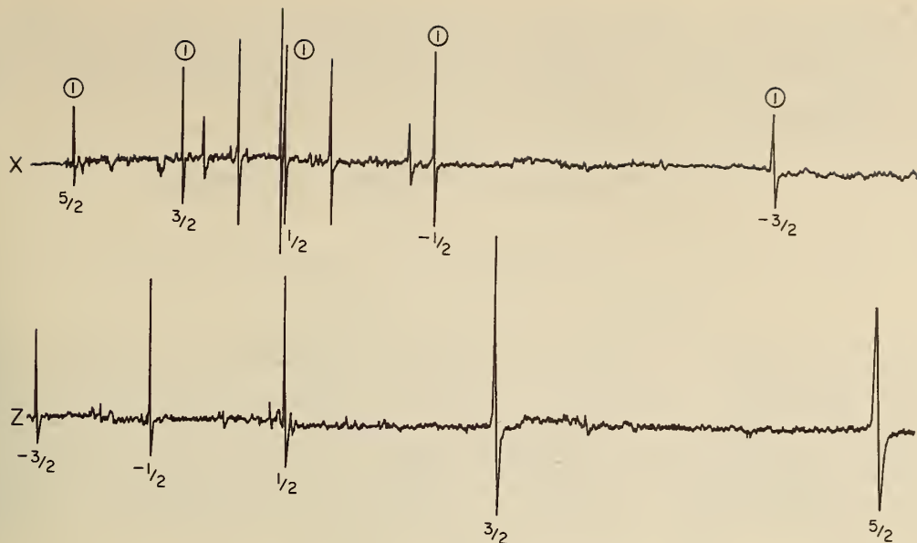
Fig. 26 EPR spectrum of \text{Fe}^{3+} in quartz (synthetic) at K-band and room temperature. Field increases non-linearly from left to right, from about 4500 to 11,300 G. The numbers below the lines indicate the value of M in the transition M \rightarrow M-1 , assuming a positive value for D , the axial field-splitting parameter. The lower trace is the H parallel to the Z axis (optic axis) of the quartz. In this orientation, the spectra of all three sites coincide. When the field is parallel to one of the quartz X axes, it is thereby parallel to the principal axis of one of the three sites; the spectrum of this site is labeled by the circled 1's. At the same time, the field makes equal angles ( 60^\circ ) with the axes of the other two sites, whose spectra coincide to give the other five lines observable at this orientation. The origin of the weak lines which can also be seen in these traces is as yet unknown.
