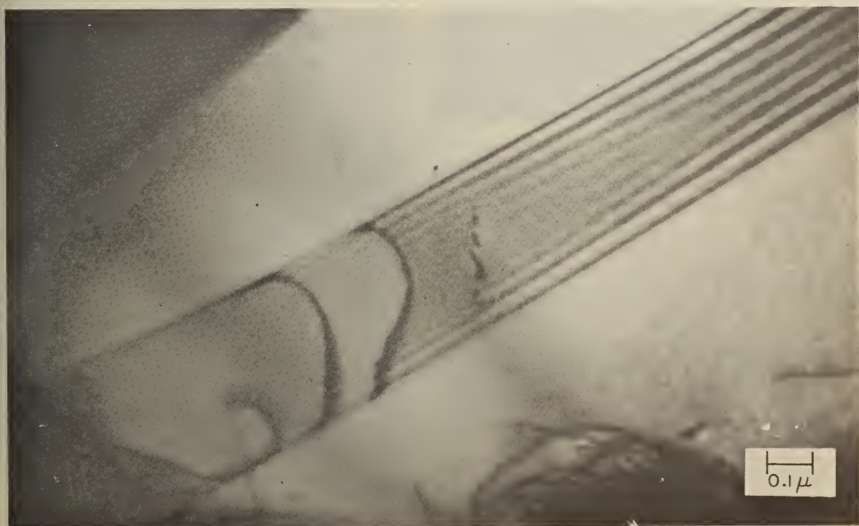
Fig. 16 Transmission electron micrographs of a single-ended Frank-Read source (s) in operation. Sample is 302 stainless-steel foil approximately 2000 Å thick
