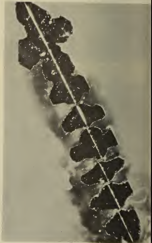
Fig. 17 Section of copper dendrite showing twin boundary
