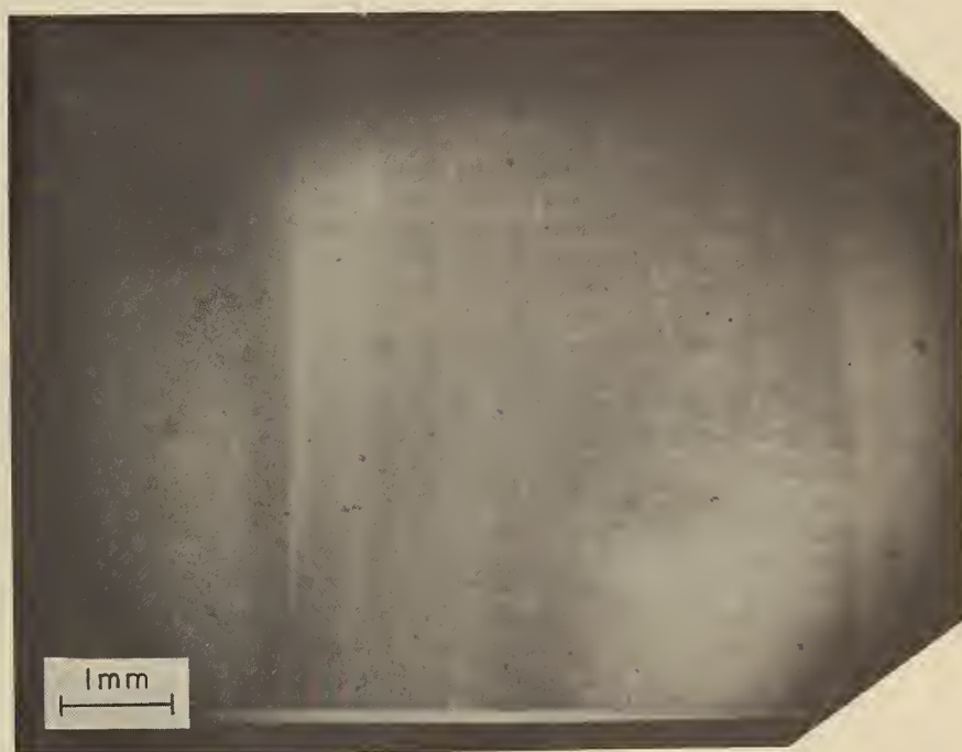
Fig. 23 Diffraction topographs from a pair of ADP (101) crystals. These had been string sawed and chemically polished. The image doubling is due to undispersed alpha doublet. Although the significant long-range strain appears, there are some regions free of the small images which are tentatively identified as emergent dislocations
