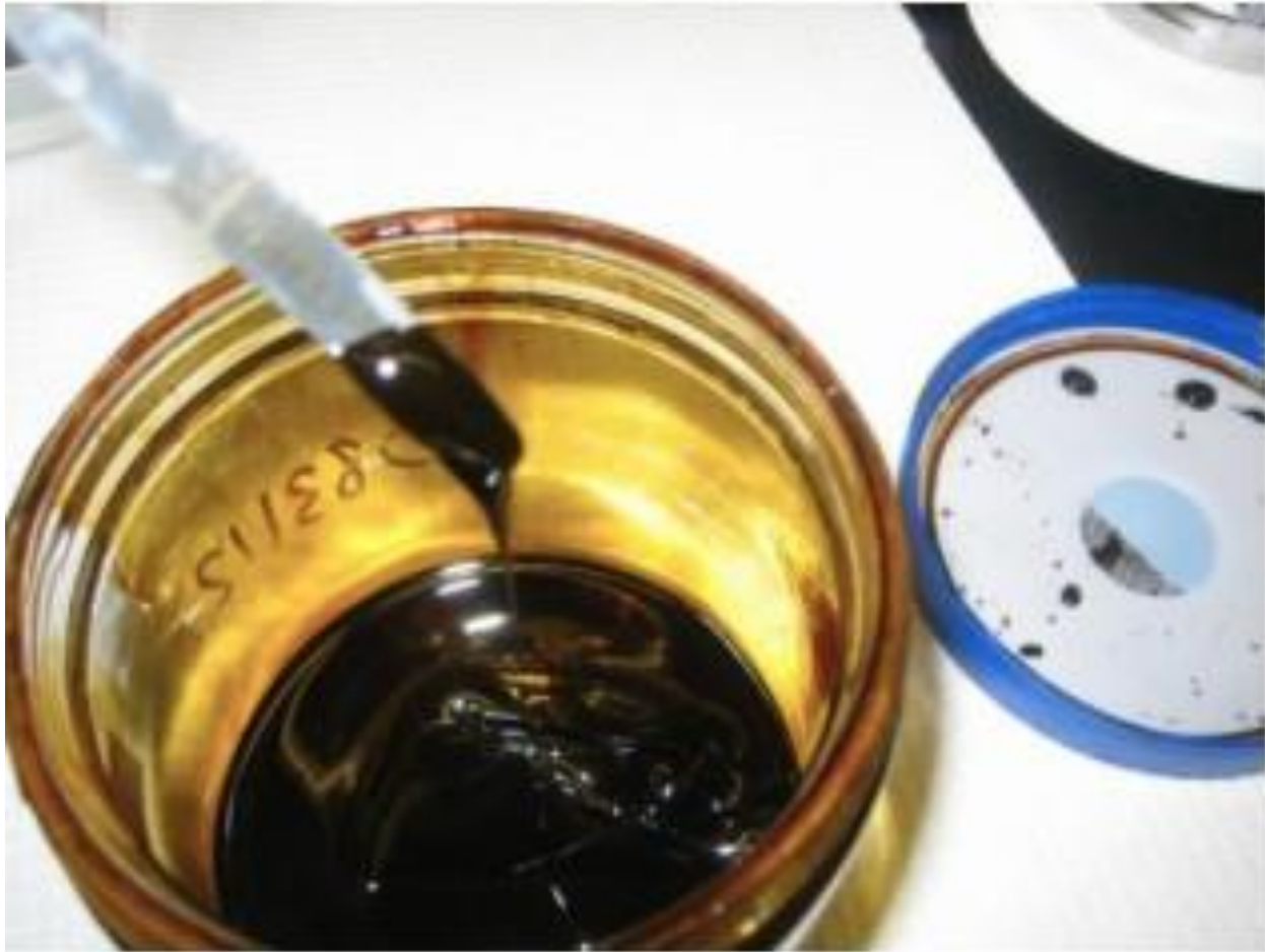
Figure 3. Dark syrupy liquid from the extraction of oiled sand-patties used to prepare candidate SRM 2777.
