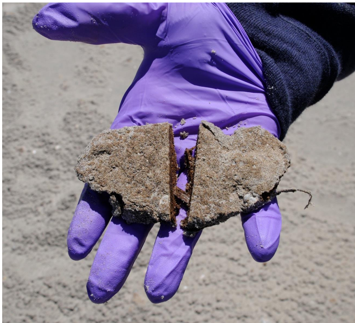
Figure 2. Image of oiled-sand patty typical of those collected for preparing candidate SRM 2777. Approximately 1.7 kg of sand patties were collected from Gulf Shores, Alabama in August 2012 and solvent extracted (with volume fraction 90/10 dichloromethane/methanol). The solvent was removed leaving a dark syrupy liquid (Figure 3). One hundred and twenty grams was sent to the NIST who prepared a solution of 71 mg of extract/gram in toluene, added 1.3 mL and then filled the ampoules with argon prior to sealing.
