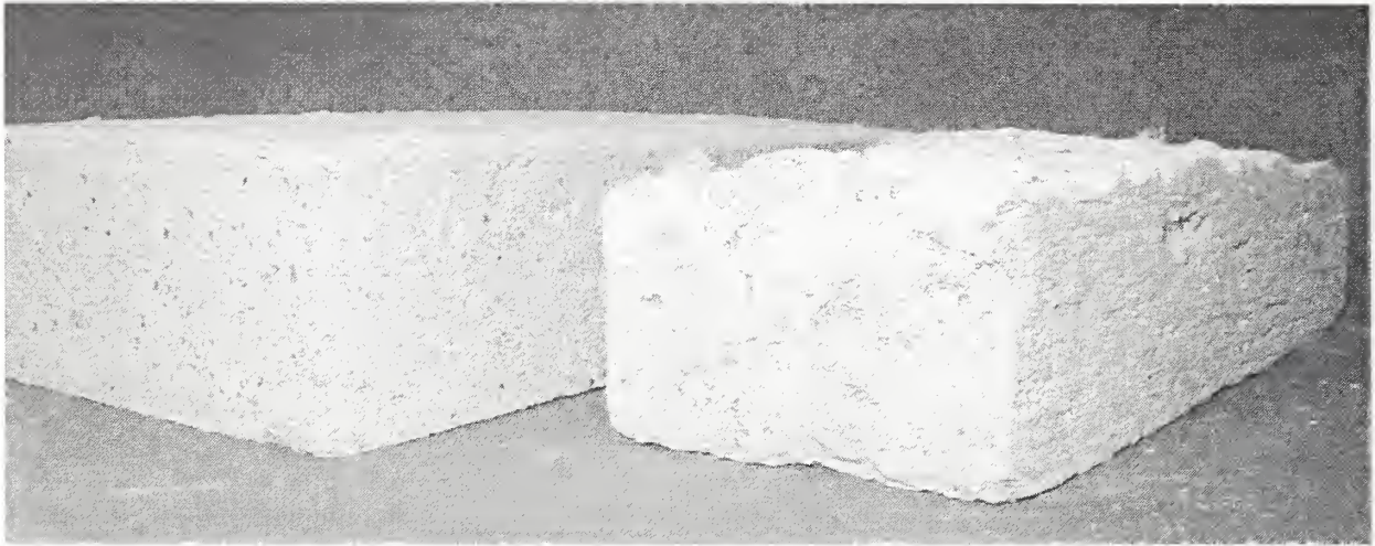
Figure 1–1. Examples of sprayed fire-resistive materials: (left) material based on gypsum and vermiculite aggregate; (right) material based on mineral fibers and cementitious binder.
