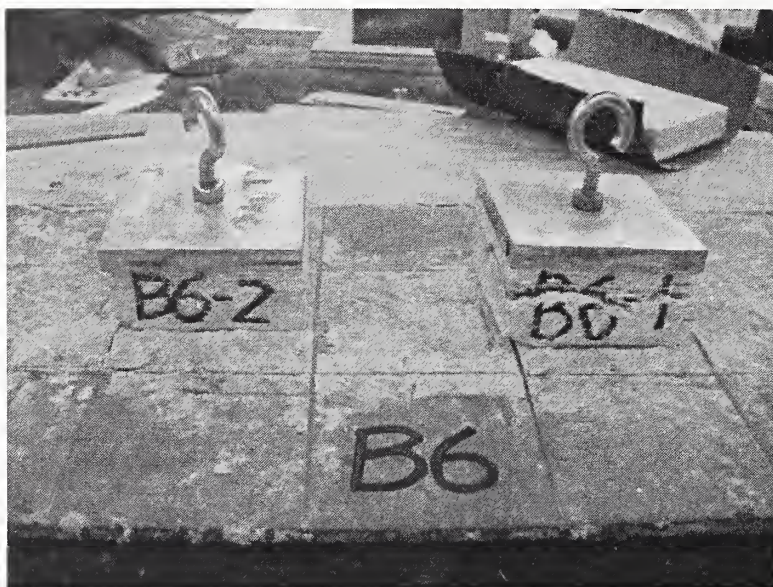
Figure 7–15. Results of second tests after repair: specimen on left had adhesive failure and specimen on right had cohesive failure.
