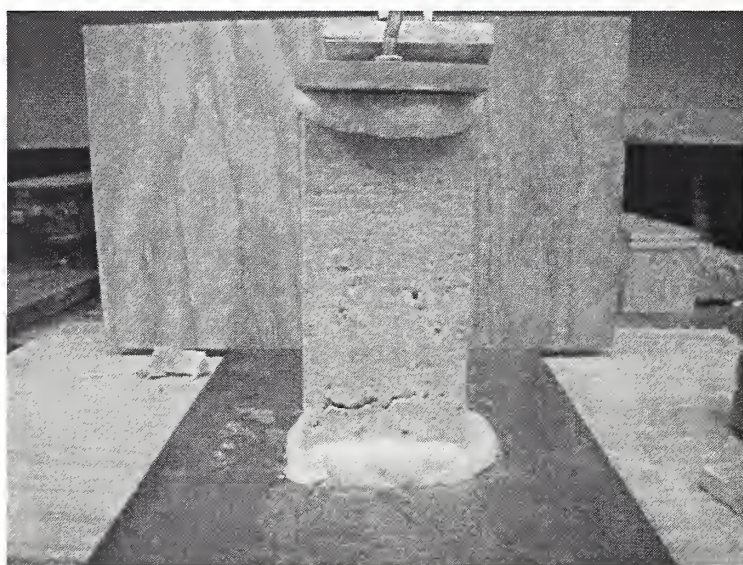
Figure 7–16. SFRM specimen after measuring in-plane cohesive strength.
