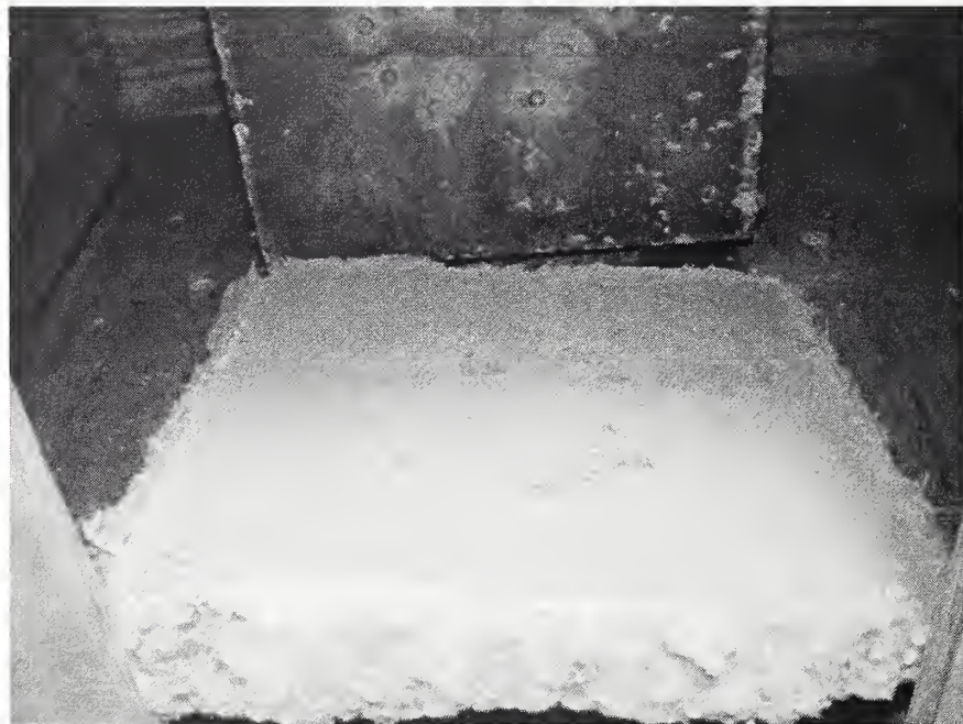
Figure C-4. Photograph showing damage to the SFRM after a ballistic impact at 0 degree. The SFRM layer completely separated from the steel plate.
