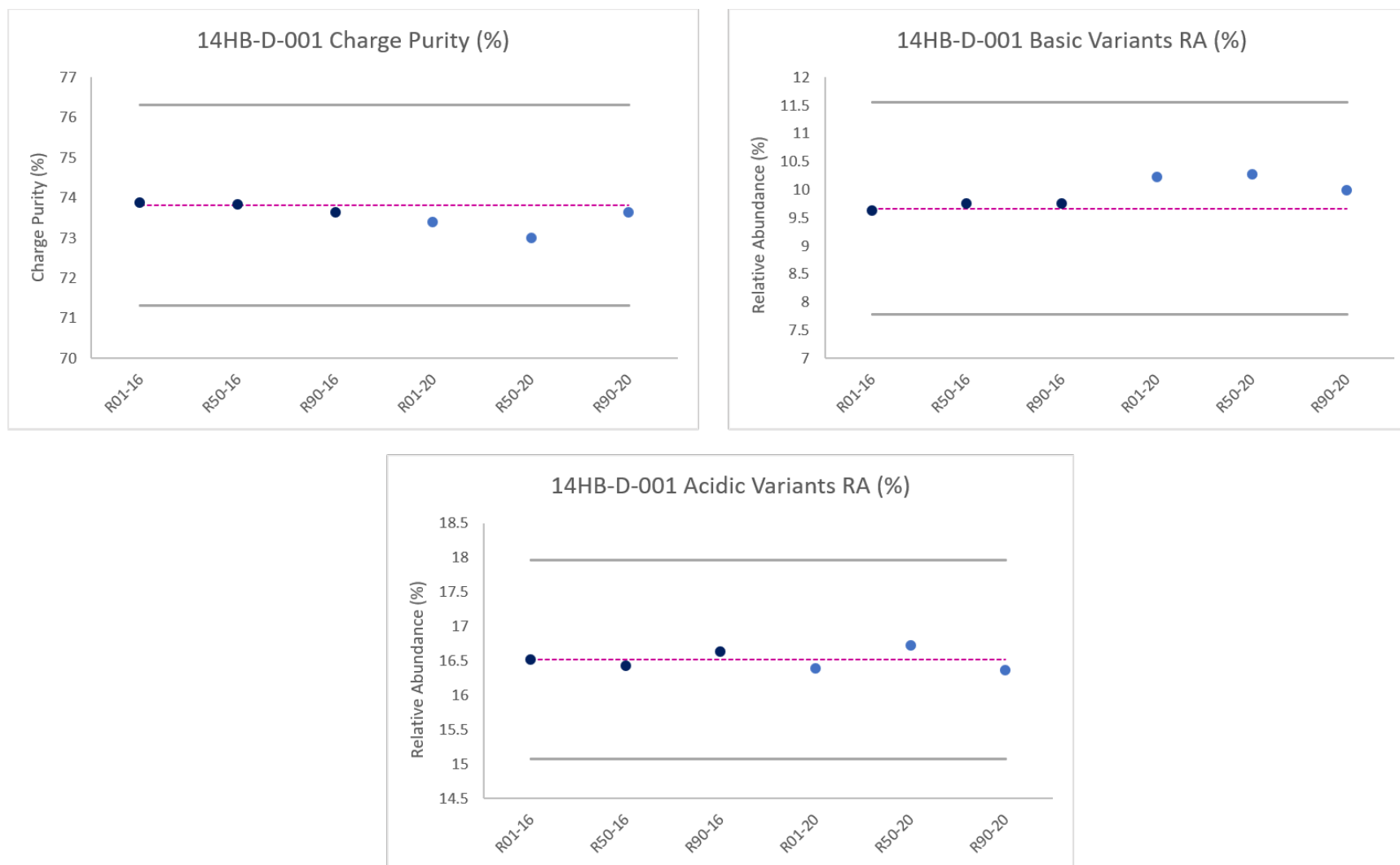
Figure 15. Charge heterogeneity control charts using capillary zone electrophoresis for lot 14HB-D-001. Initial certification (0y) data is shown in dark blue and 5YSV (5y) in light blue. Pink dotted line corresponds to the non-certified value assigned in the original 2016 certification. Control limits set at \pm 3\sigma_c (grey bars)
