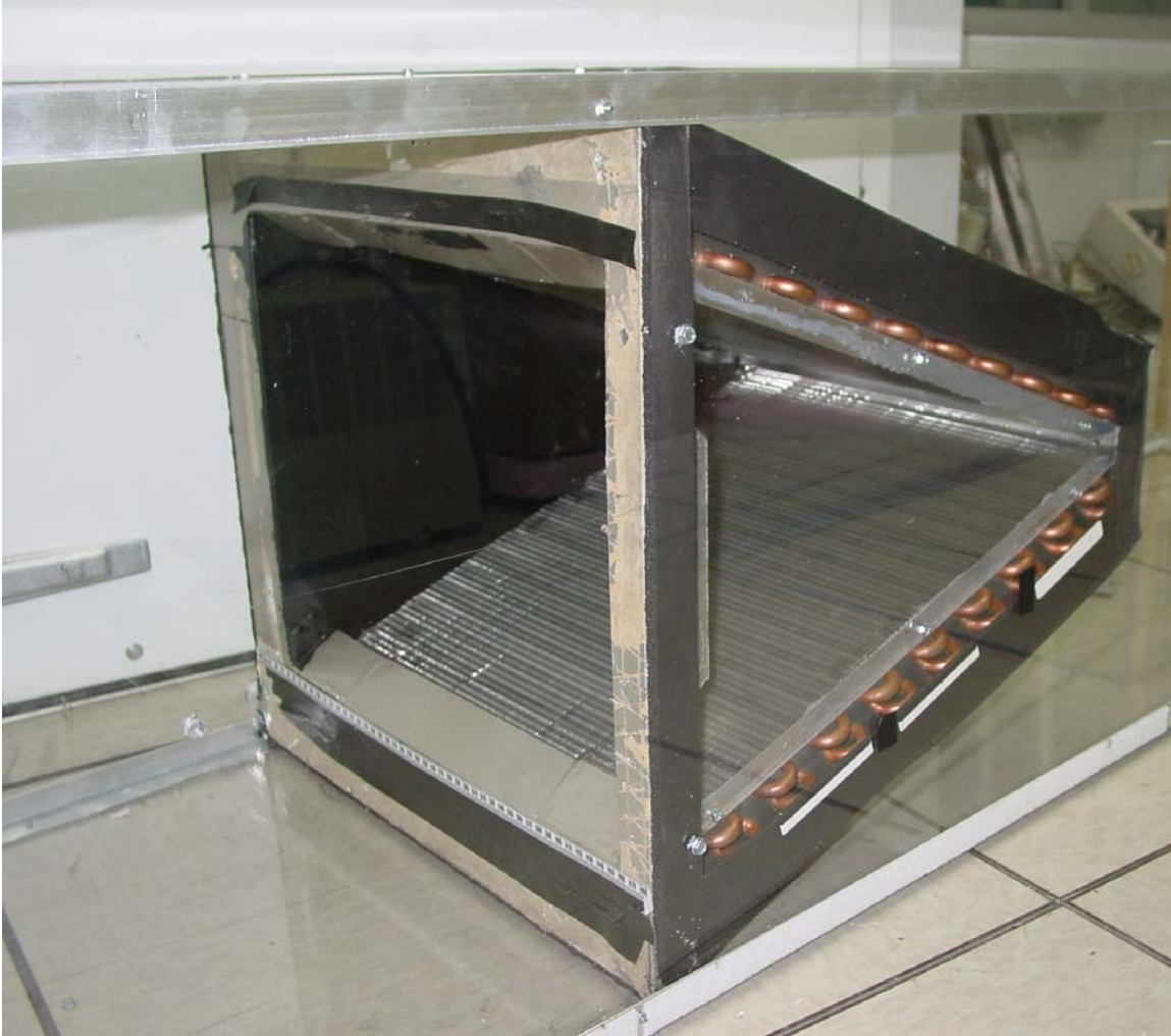
Figure 5.3.1 A-Shaped Coil Test Section
