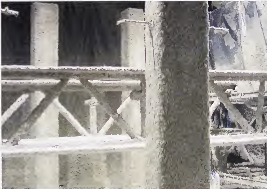
Figure 6–42. SFRM-coated steel components prior to a test.
