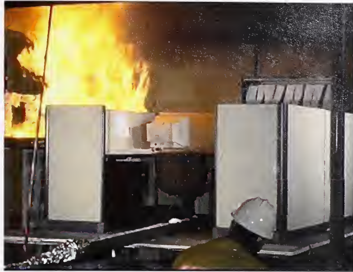
Figure 6–31. Fire test of a single workstation.
