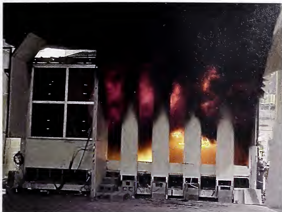
Figure 6–34. Three-workstation fire test, 2 min after the start.
