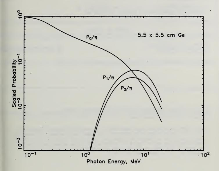
Figure 1. Peak probabilities for total absorption,  $P_0$ , single-annihilation escape,  $P_1$ , and double-annihilation escape,  $P_2$ , for the 5.5  $\times$  5.5 cm Ge detector irradiated by broad beams of gamma rays incident with energy  $E_0$ . The results have been scaled by the detection efficiency n to remove dependence on the angle of incidence.
