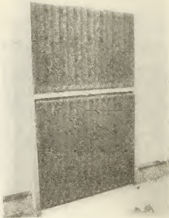
Figure 30. Photograph of collector-storage water wall installed in test frame
