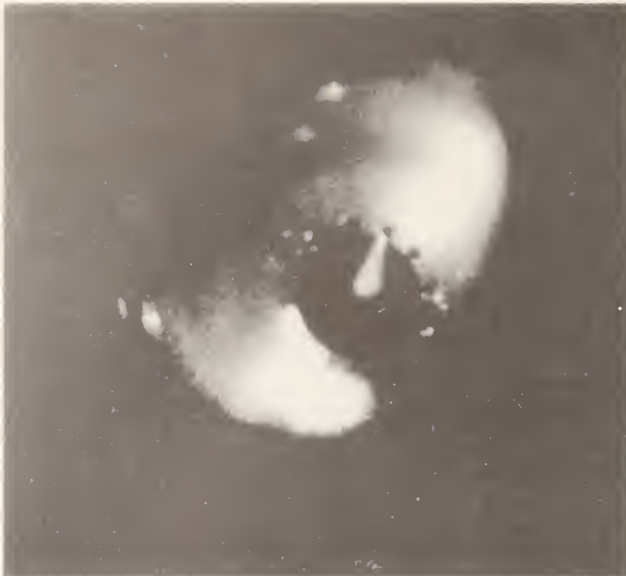
Stopping sodium atoms with light. A beam of sodium atoms approaching the camera from the upper right at speeds exceeding 1000 m/sec is brought to a virtual standstill by a laser beam aimed in the opposite direction. In this experiment at NBS, Gaithersburg, the atoms travel down the axis of a solenoid (whose opening appears as the dark circle at the center of the photograph) and spread out as they come to a virtual halt near the opening. 18
