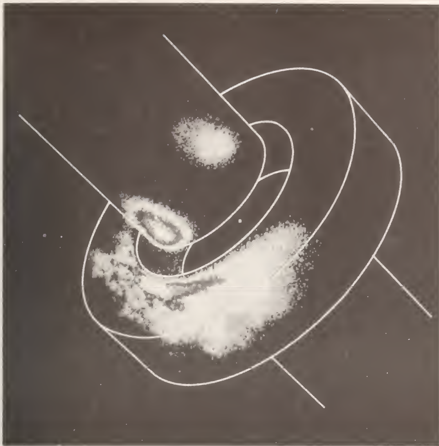
Single ion of mercury. The white dot at the center of this false-color image is a laser-cooled \text{Hg}^+ ion in an electromagnetic trap. This image was made with a photon-counting imaging tube sensitive to the 194-nm fluorescence light scattered from the ion and trap electrodes. The white overlay shows the position of the electrodes of the ion trap. The circular ring electrode has an inner diameter of about 0.9 mm. To photograph such an ion requires a minimum exposure time of about 50 \mu\text{sec} . The effective temperature of the ion was approximately 2 mK. The computerized imaging system used here was developed by Charles Manney and John Bollinger at the National Bureau of Standards. The first photographic images of single ions were reported in reference 15.
