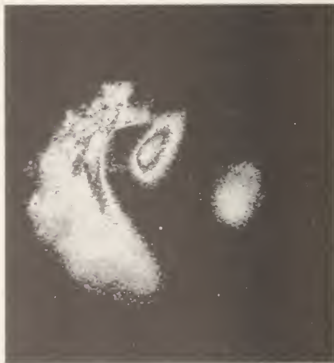
Fig. 3. False color image of a single \text{Hg}^+ ion (small isolated dot slightly below the center) stored in an rf trap. The other shapes are due to light reflected from the trap electrodes, whose orientation is the same as in Fig. 2. The largest reflection is from the front surface of the ring electrode. The two smaller reflections are from the edges of one of the endcap electrodes. Computerized imaging system developed by C. Manney and J. J. Bollinger (NBS). [Adapted from (43) with permission from the American Institute of Physics]
