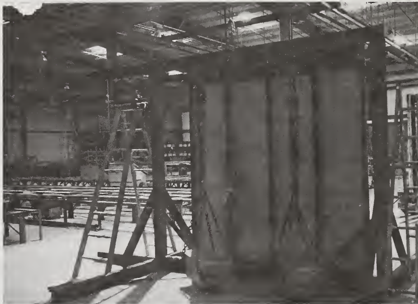
Figure 3: Structural testing of 8 ft. x 8 ft. sample of load-bearing sidewall.
