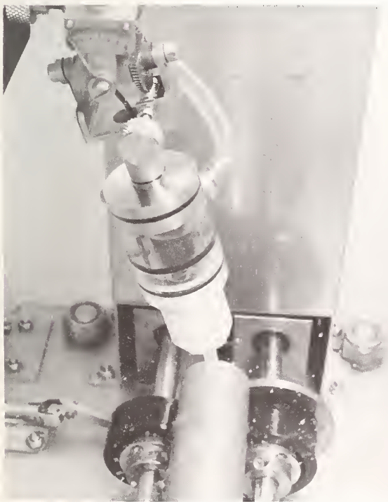
This laboratory set-up ultrasonically monitors the surface condition on a rotating part by means of sound echoed from the part surface.
