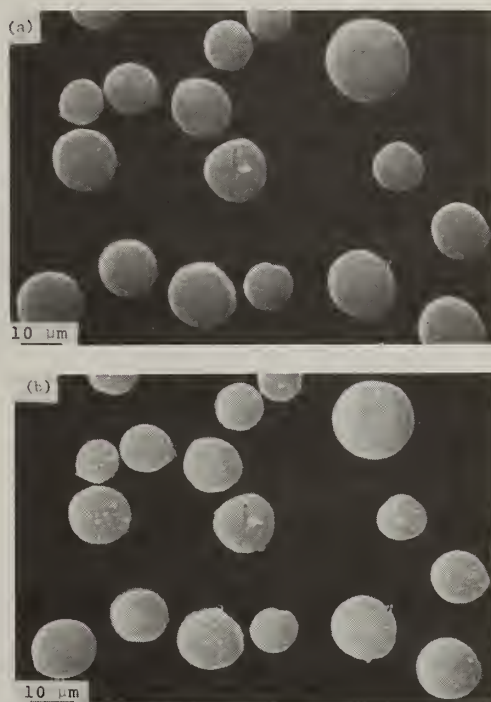
Figure 12. Microstructures of emulsified droplets of Sn-5%Pb: (a) Rapidly cooled to -25°C, (b) Rapidly cooled and then held one month at room temperature 1000X.
