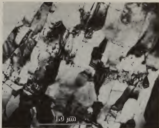
Figure 4. Longitudinal and transverse TEM views in RSPD Ni superalloy.
