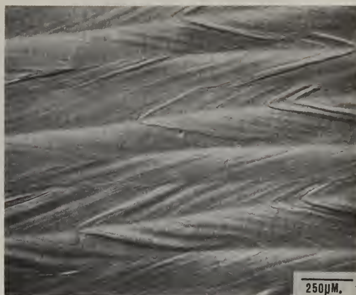
Fig. 2. Actual view of the surface of 52150 bearing steel formed by an oscillating beam ( f=62.5 hertz).
