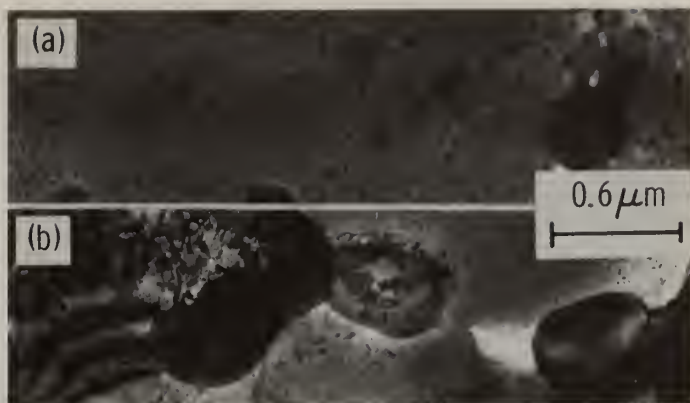
Figure 8. Microstructure of (a) X7091 (slightly overaged); and (b) X7090 T6511 showing greater number of, and somewhat larger, \text{Co}_2\text{Al}_9 particles in the X7090.
