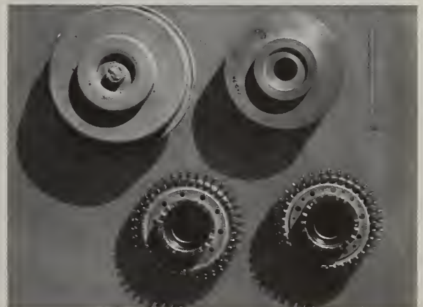
Figure 9. P/M Rene 95 Turbine Disks. (Top left-as-HIP shape, Top right-machined sonic shape, Bottom left-final machined 1st stage disk, Bottom right-final machined 2nd stage disk.)
