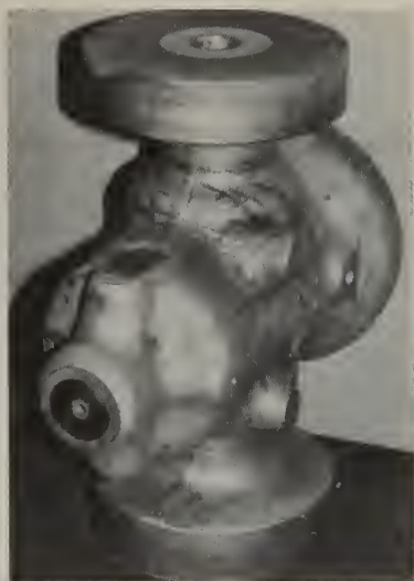
Figure 12. Alloy Steel Valve Body Clad on the Inside with Alloy 625 Powder using Hot-Isostatic-Pressing.
