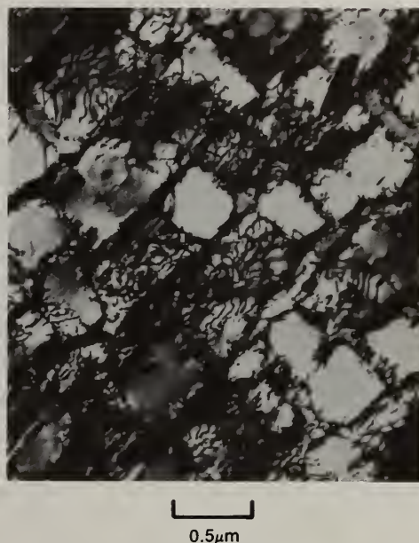
Figure 9: Bright-field TEM photomicrograph showing interfacial dislocations in NiAlMo alloy after solution heat treatment for two hours at 1316^{\circ}\text{C} ( 2400^{\circ}\text{F} ) followed by 10 hours at 816^{\circ}\text{C} ( 1500^{\circ}\text{F} ).
