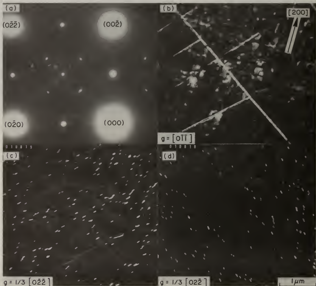
Figure 2 (a) One quadrant of [100] zone with (0\bar{1}\bar{1}) satellites (b) D.F. using (0\bar{1}\bar{1}) and satellite spots (c) D.F. using 1/3 (022) (d) D.F. using 1/3 (022)
