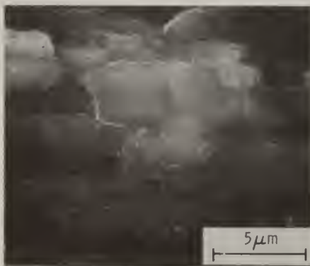
Figure 25. Fracture of X7091 under liquid gallium is intergranular.
