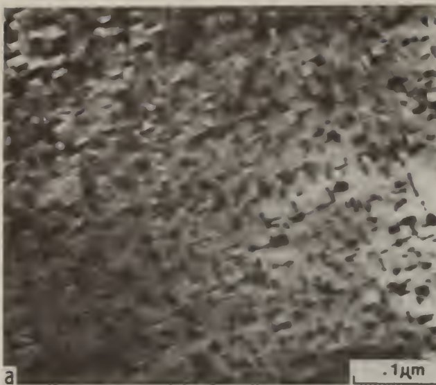
Figure 1. TEM micrographs showing fine, uniformly distributed precipitates typical of most age hardening alloys.
