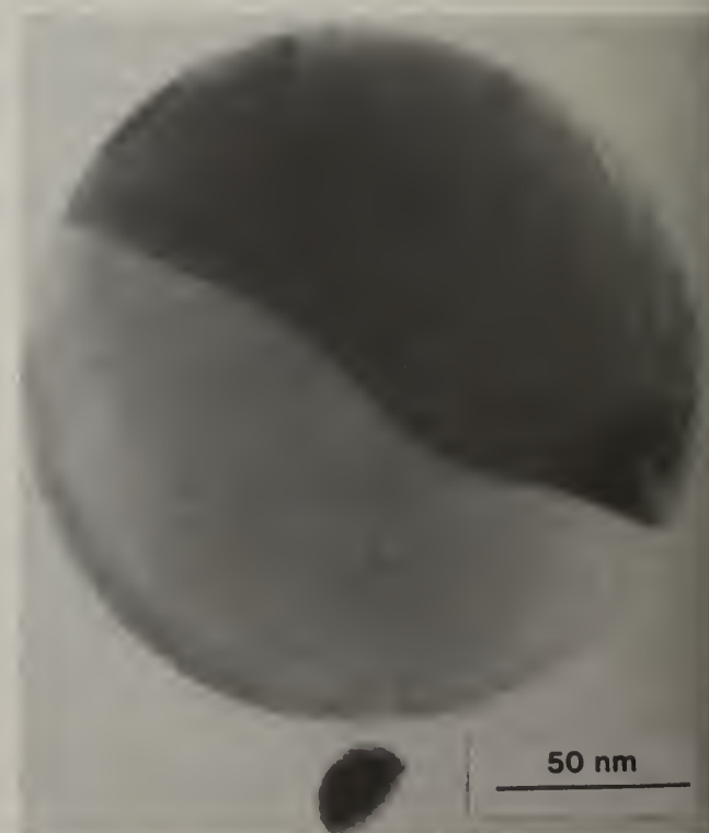
Figure 2. Examples of a bicrystal in Al-Ge eutectic powders.
