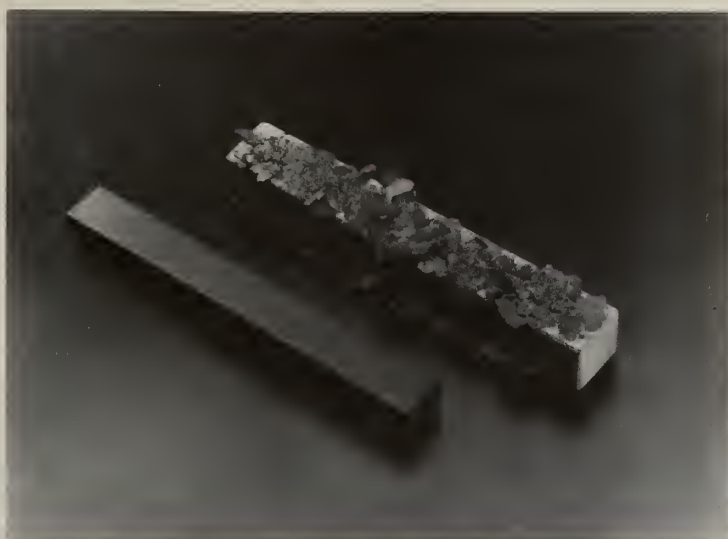
FIGURE 14 STATIC OXIDATION BEHAVIOR OF UNCOATED ALLOY-185 AND ALLOY PWA 1120 Cycle 2100° F/1 Hr/AC
