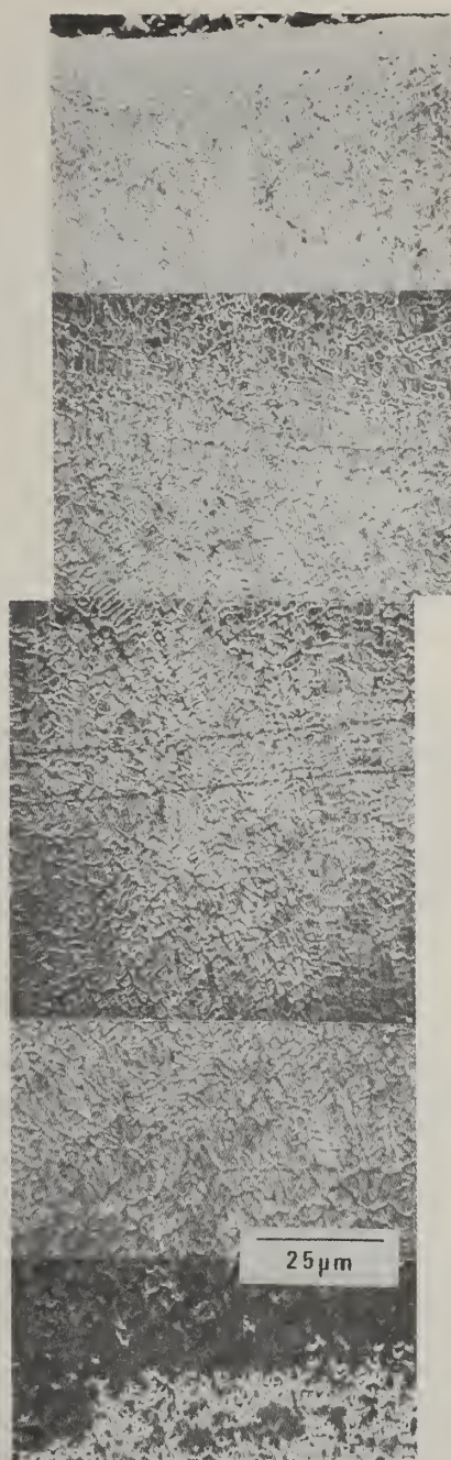
Fig.5. Shows a homogenous cellular solidification structure in the rapidly solidified M2 high speed steel.
