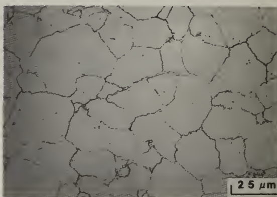
Figure 2 Typical as-deposited microstructures of RSPD Hastelloy Alloy X; (etched).
