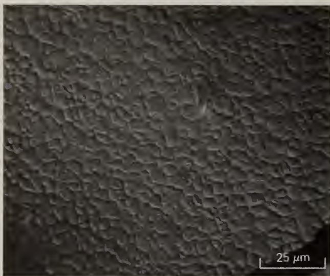
Figure 2. Microstructure of JBK-75 (a) IGA Powder (b) CA Powder
