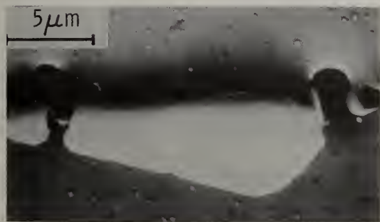
Figure 21. SCC initiation at constituent particle in 7075.
