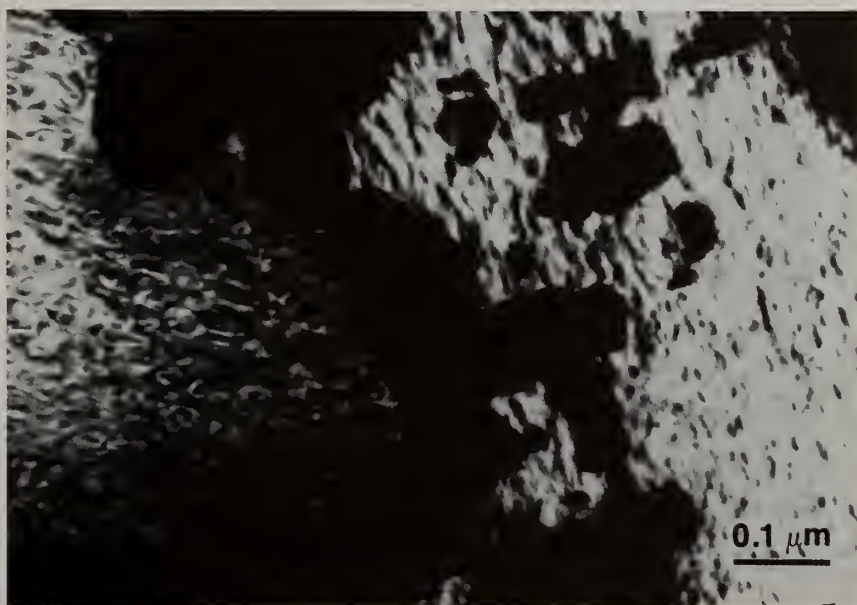
Fig. 6 Microstructure in the superalloy ribbon containing 0.75 w/o boron, annealed at 760°C for 24 hours.
