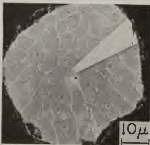
Fig. 6 Solidification microstructure developed in Al-9 w/o Fe droplets.
