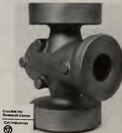
Figure 11. Alloy 625 Valve Made from Hot- Isostatically- Pressed Powder (Top-as-HIP Part, Bottom-Machined Part).
