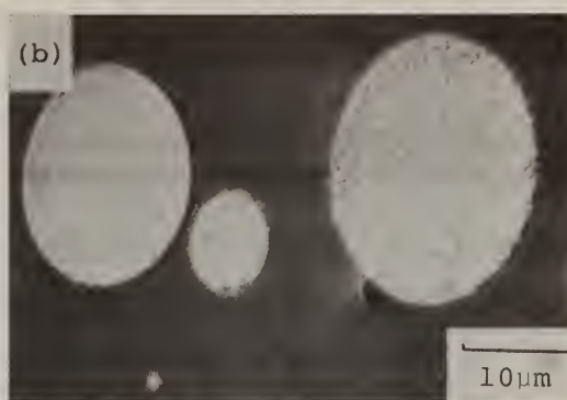
Figure 10. (a) Optical micrograph of cross-sectioned and etched 316 BCC and FCC particles after undercooling. Fcc particles are light in color. (b) Backscattered electron micrograph of the same particles, from MacIsaac [44].
