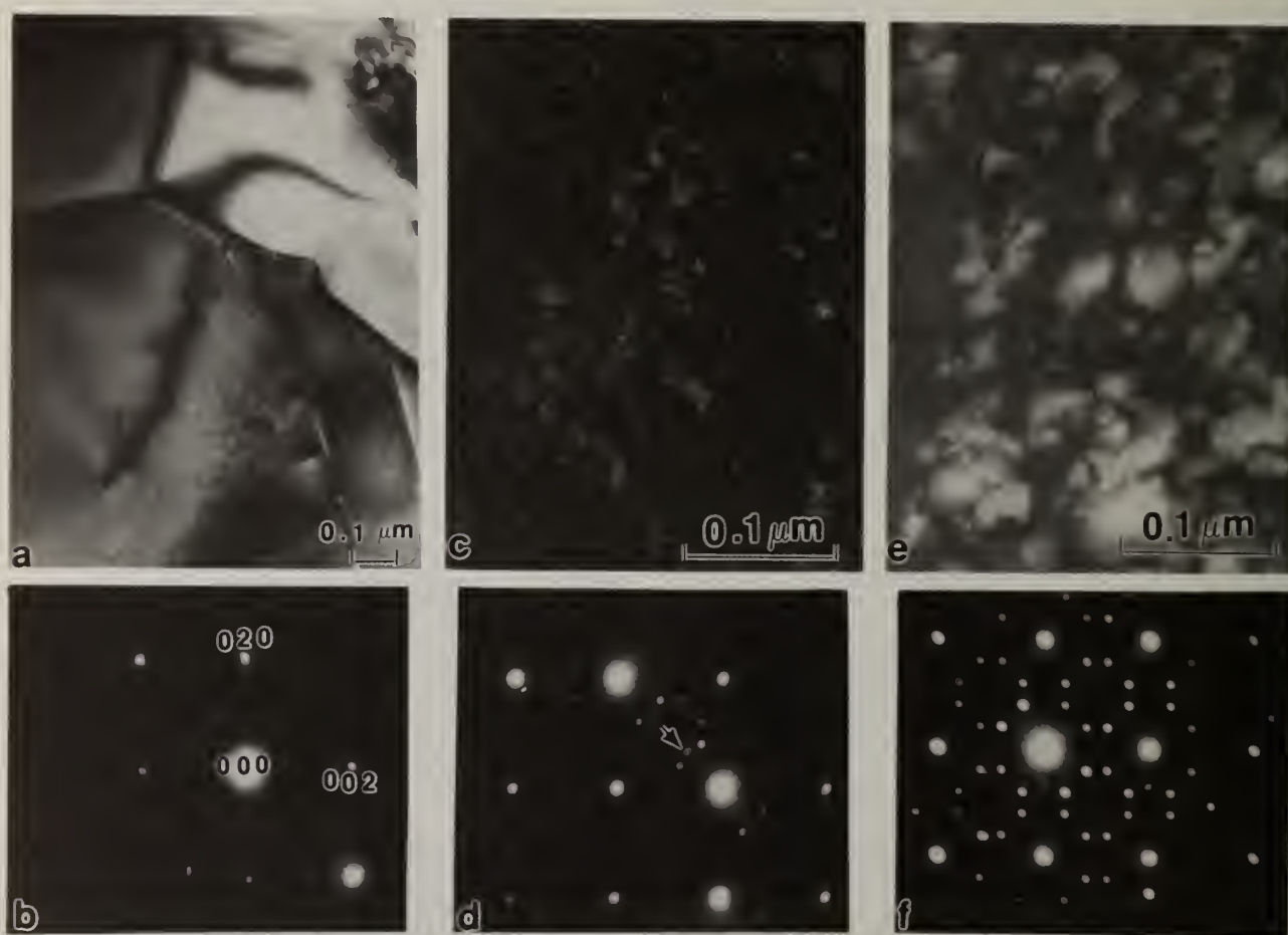
Fig. 3 Effect of heat treatment on microstructure of (a) - (d) Ni 60 Mo 30 B 10 alloy and (e) - (f) Ni 49 Mo 31 B 20 alloy. (a) Bright field TEM of sample quenched in iced brine from 1100°C, (b) [100] SAD of matrix in (a), (c) Dark field using a Ni 4 Mo spot in (d) from a sample aged at 700°C for 20h, (d) [100] SAD of matrix in (c), (e) Dark field of Ni 4 Mo spot in (f) from a sample aged at 700°C for 50h, (f) [100] SAD of matrix in (e).
