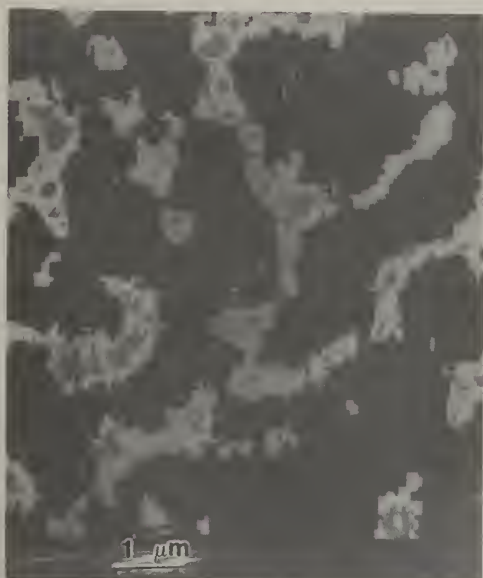
FIGURE 5(a): Microstructure of alloy with 5 wt. pct. Si showing cellular microstructure.
