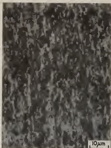
Fig. 20. Microstructure of extruded product through streamlined die of 3-in. length.
