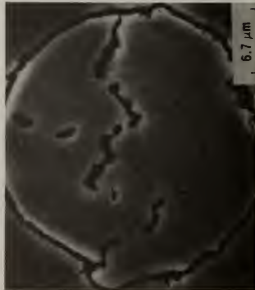
Figure 4: Microstructure of as received "Virgin" powders. a) Fe-20 wt% Mn, b) René 80 and c) Hastelloy X.
