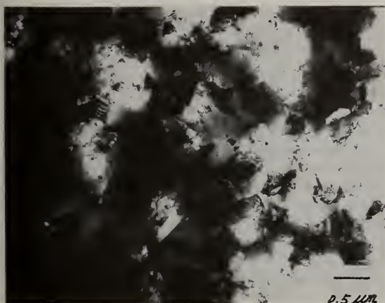
Fig. 3. TEM micrograph of alloy N-5; as extruded, longitudinal view.
