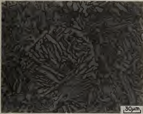
Fig. 24. REP Ti 6-4 alloy after HIPing and heat treatment.
