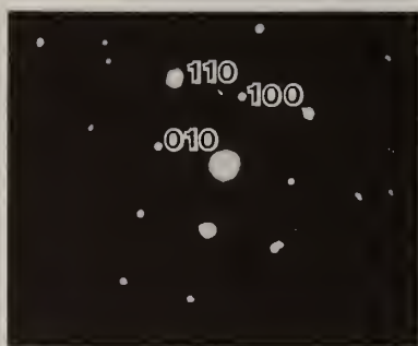
Figure 8: Selected area diffraction (SAD) pattern of a columnar grain.
