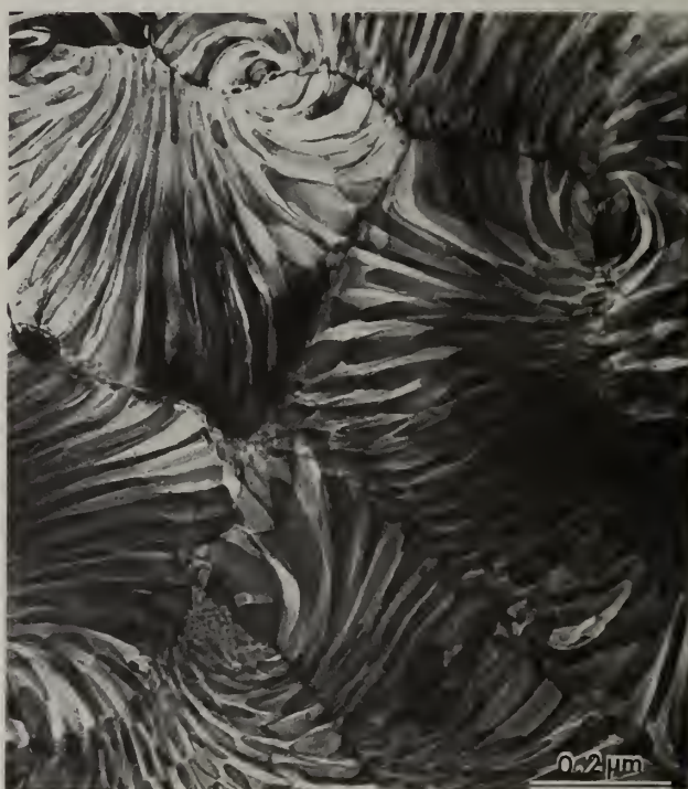
Figure 6: Region of foil consisting primarily of eutectic (TEM).
