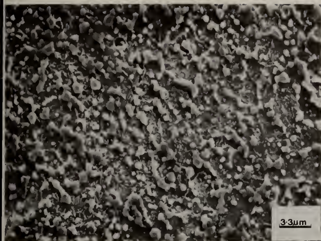
Figure 4: HIPed material (H1) from 250-840 \mu m screen fraction. Etch: Kalling's reagent. SEM.
