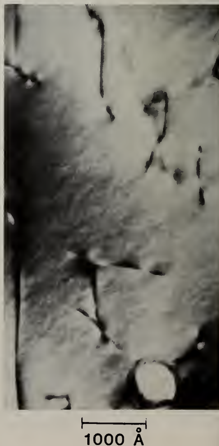
Figure 2 - TEM micrograph showing the interference thickness fringes and change of contrast for voids in stainless steel specimen # B28 processed at 800°C.
