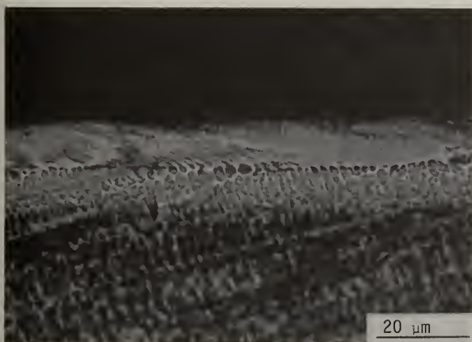
Figure 14. Mixing patterns in a rapidly laser-surface melted layer of FeMoC alloy
