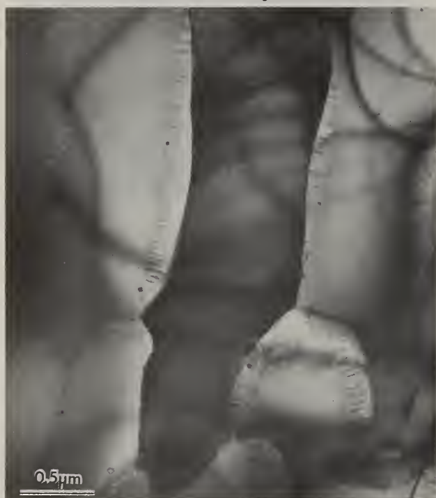
Figure 5: Region of foil consisting primarily of columnar grains (TEM).
