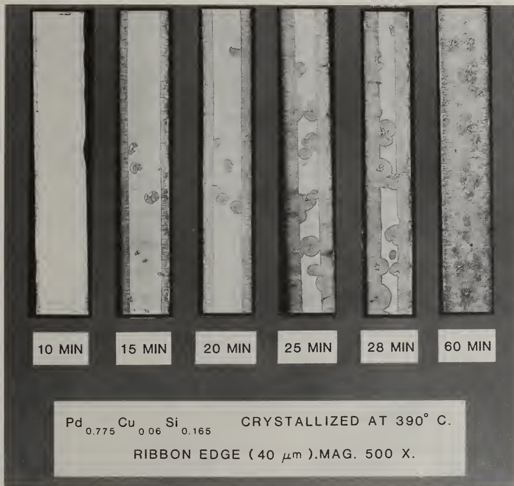
Fig. 3 Crystallization sequence of amorphous PdCuSi as a function of time at a constant temperature, by optical metallography.
