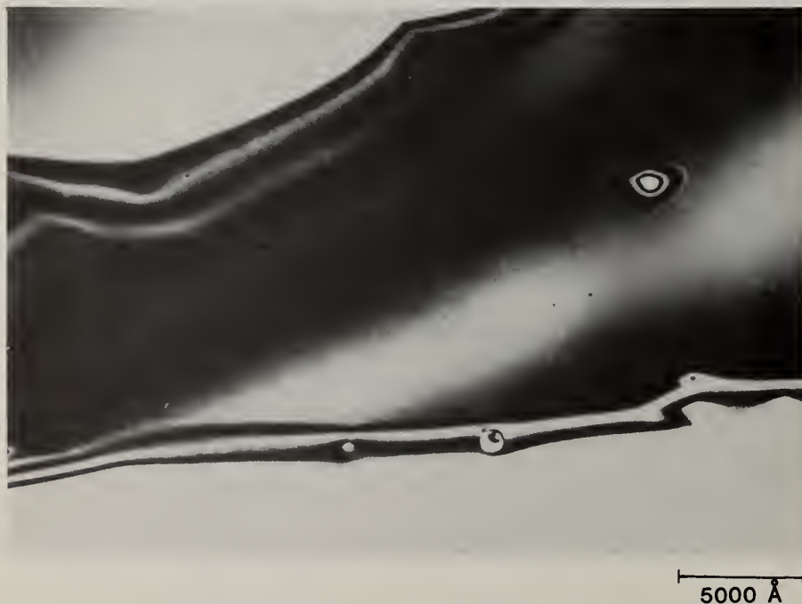
Figure 2 - TEM micrograph showing the interference thickness fringes and change of contrast for voids in stainless steel specimen # B28 processed at 800°C.
