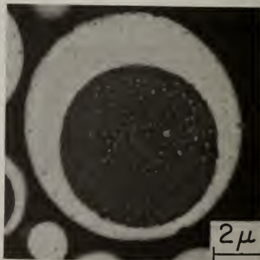
Fig. 7 Microstructure developed in Pb-40 w/o Cd droplets in which phase separation preceded solidification.
