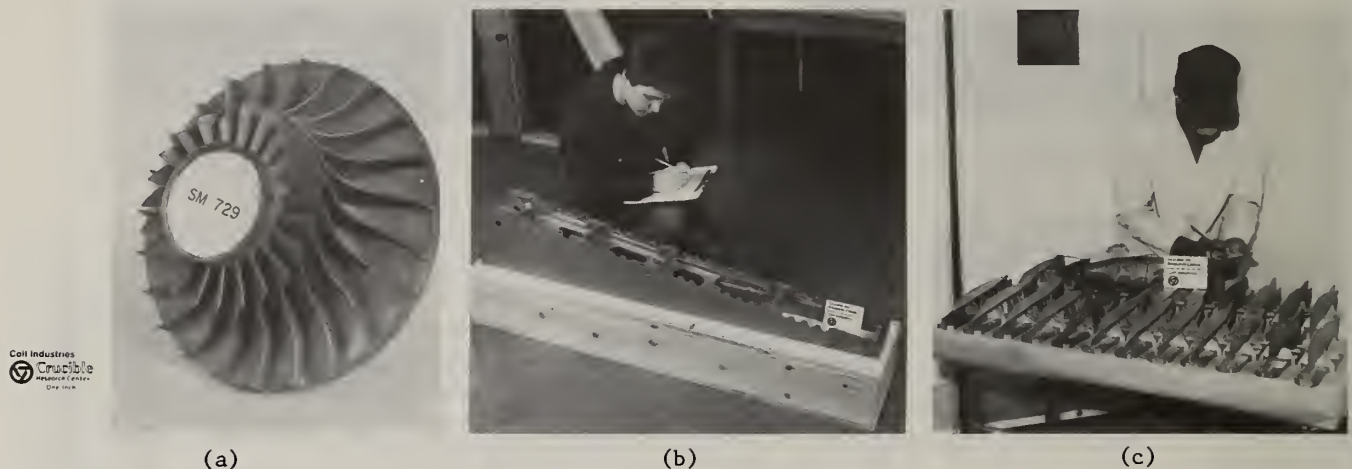
Figure 5. Hardware Produced Using Titanium Alloy Powder and Crucible's Ceramic Mold Process. (a) Compressor Rotor, (b) Arrestor Hook Support Fitting, and (c) Fuselage Braces.
