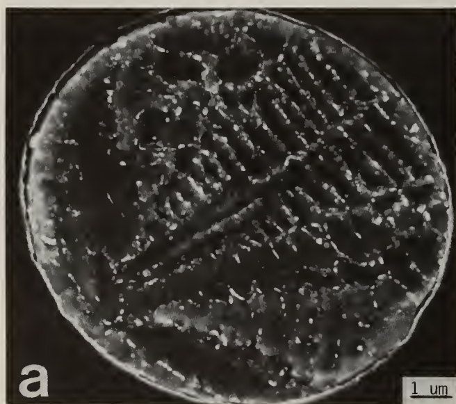
Fig. 4. Two 12 \mu\text{m} -diameter argon atomized C101 powder particles exhibiting (a) dendritic and (b) microcrystalline microstructures.
