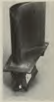
FIGURE 10 BLOCKLETS TO BE BONDED TO PRODUCE THE FULL AIRFOIL CROSS SECTION
