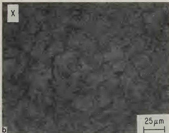
Fig. 9. Hot-rolled RSPD Rene' 80, reduced 50% in thickness at 1230°C, appeared to have undergone dynamic recrystallization as equiaxed grains 10 μm in diameter resulted. Micrographs taken (a) of the rolling plane and (b) perpendicular to the rolling plane.
