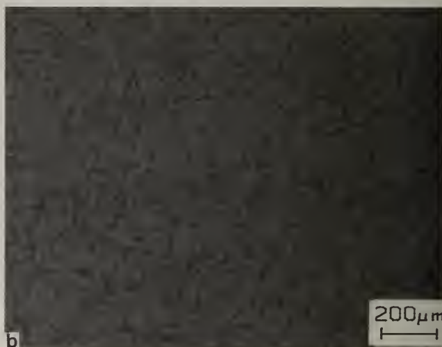
Fig. 6. Typical grain sizes developed in RSPD experimental alloy C4 following (a) 1 hr. at 1220°C were 25 μm while those resulting from (b) critically straining 4% (reduction in thickness) before annealing averaged 150 μm.
