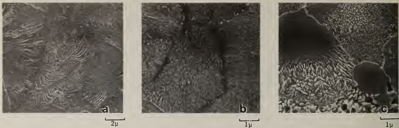
FIGURE 4: Typical microstructures of as-hot-pressed alloys: a = Al-5.7Fe-6.2Co; b = Al-5.7Fe-6.1Ni; c = Al-7.4Fe-3.4Ce.
