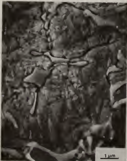
Figure 1: Atomized powder particle cross-section (SEM) from 550-700µm screen fraction. Etch: Kalling's reagent + HCl/Picral.
