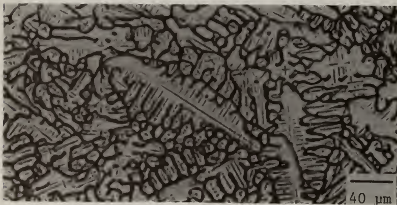
Figure 1. The dendritic morphology etched to reveal fine "primary" dendrites within the dendritic arms. The sample was supercooled 175 K before quenching in molten lead.
