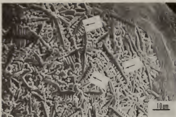
Figure 1(a). Atomized powder; 119 to 213 \mu\text{m} size screen. Arrows point to austenite dendrites. SEM.
