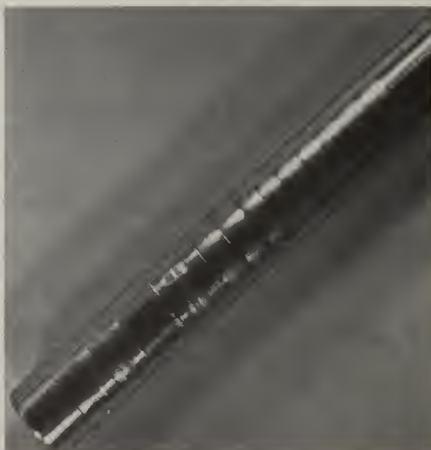
Fig.3. A cylindrical bar (M-42 tool steel) was treated using electromagnetically oscillated beam generated by unit shown in fig.2.
