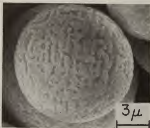
Fig. 4 Solidification microstructures developed in Pb-17.7 a/o Sb alloys at different undercooling levels. A transition from eutectic (a) [ \Delta T=19^\circ\text{C} ] to a dendritic surface morphology (b) [ \Delta T=130^\circ\text{C} ] is illustrated.
