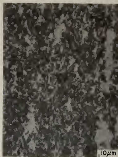
Fig. 21. Microstructure of extruded product through streamlined die of 2-in. length.
