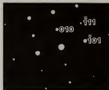
Figure 9: Diffraction pattern taken from a columnar grain and its surrounding eutectic.
