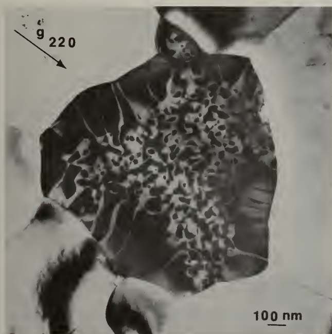
Fig. 4. Bright-field electron micrograph of a Ni 3 Al sample containing 1000-ppm B; the APB structure in small grain. Foil normal and electron-beam direction near [114].
