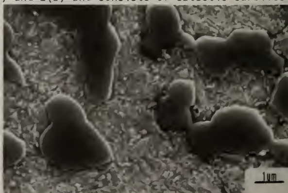
Figure 2(b). HIPed and heat-treated material; \leq 44 \mu\text{m} size screen. SEM.
