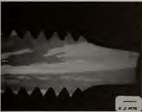
Fig. 9. The grain structure of N-5 test bar after ZAP treatment (7.6 cm/h at 1260°C) plus heat treatment.
