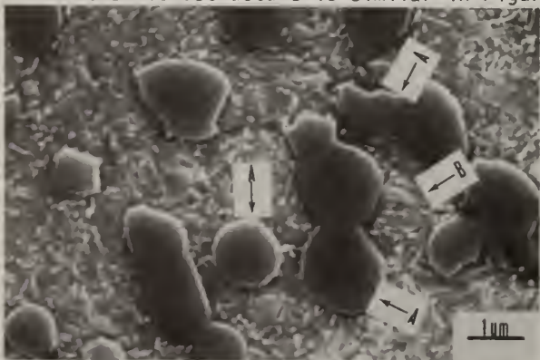
Figure 2(a). HIPed and heat-treated material; 119 to 213 \mu\text{m} size screen. A = eutectic carbides, B = area showing secondary carbides in tempered martensite. SEM.
