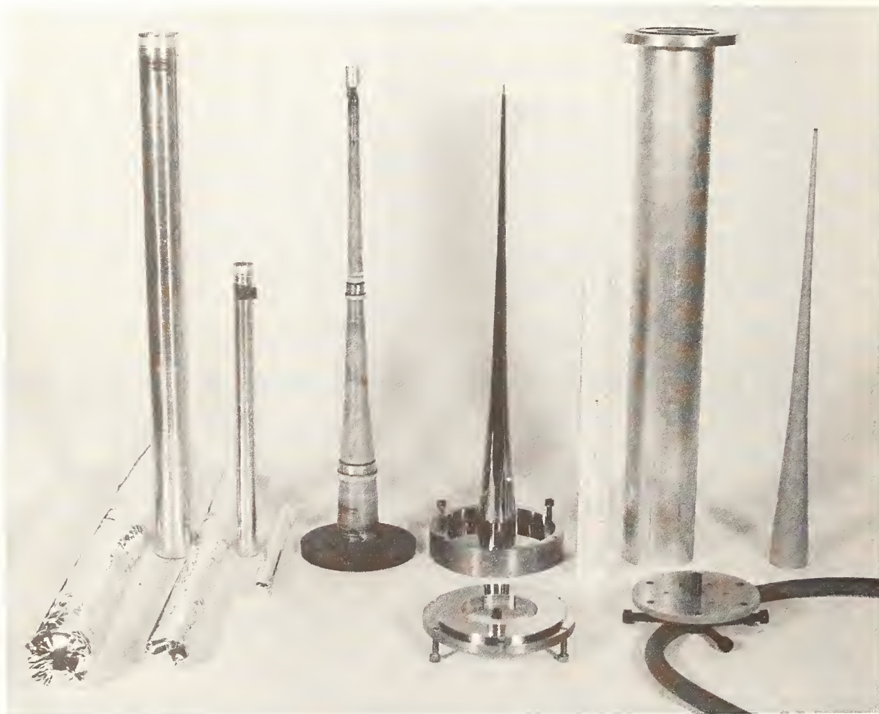
Fig. 8. From left to right: Superinsulation packs and radiation shields, glass fibre epoxy sleeve, brass cone with flange mould and cover, 30 cm scale, wax/sand mould with flange, glass powder/epoxy displacer.
