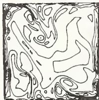
Figure 2B. Vorticity contours corresponding to Figure 2A. \Delta\omega = 0.75/\text{sec} . \omega maximum at the wall is 12.9.
