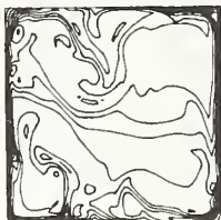
Figure 2C. Isotherms corresponding to Figure 2A. \Delta T = 0.5^\circ\text{F} .
