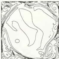
Figure 3B. Vorticity contours corresponding to Figure 3A. \Delta\omega = 10.0/\text{sec} . \omega maximum at the wall is 145.4.
