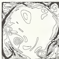
Figure 3C. Isotherms corresponding to Figure 3A. \Delta T = 0.5^\circ\text{F} .
