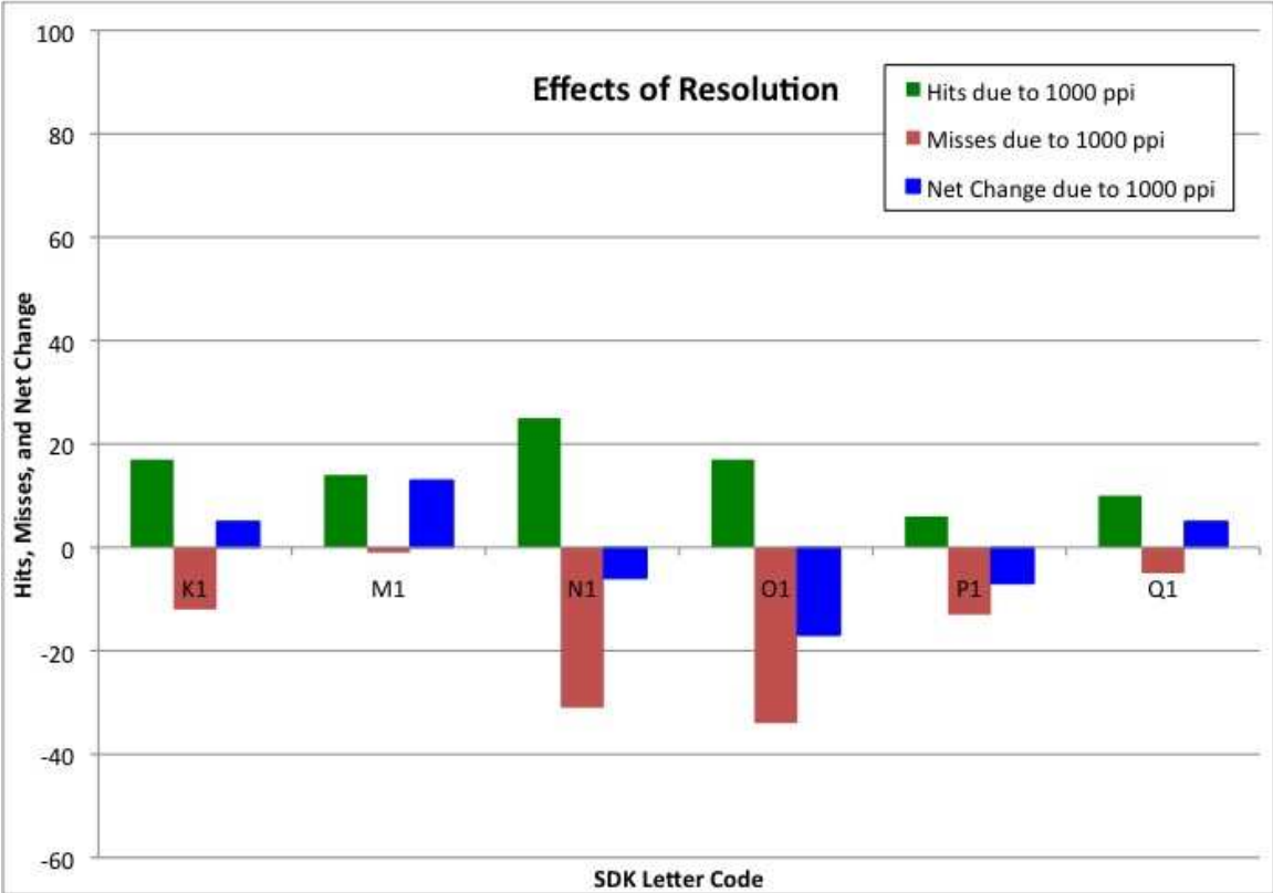
Figure 12: Effect of latent resolution on Rank 50 detection rate; searches of 1000 and 500 ppi latents against gallery of size 5K
