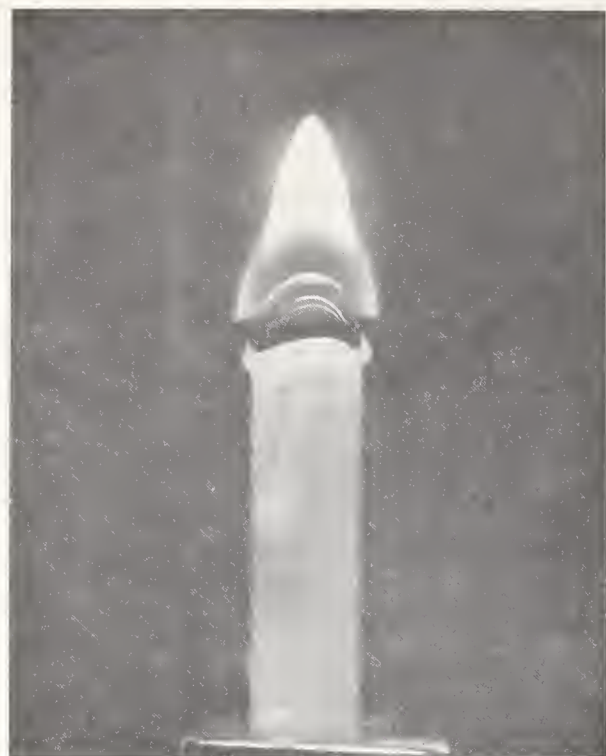
FIGURE 1. Polyethylene burning close to extinction limit at 1 atm.
