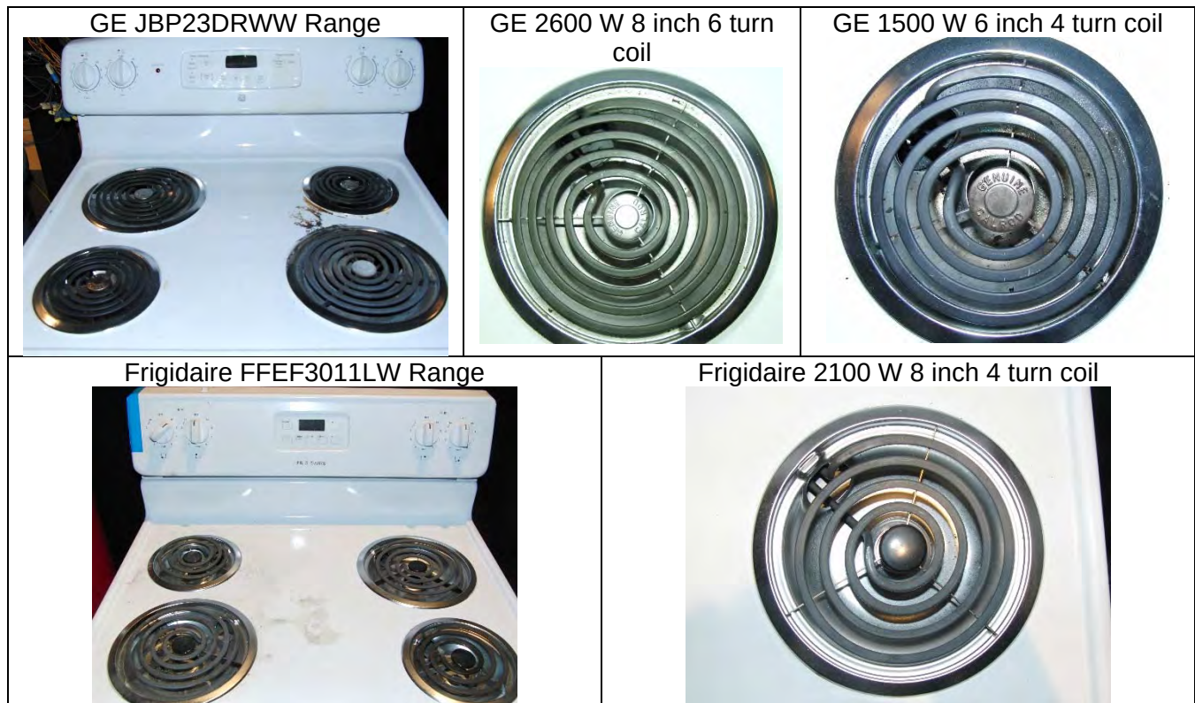
Figure 6 – Range tops and burners used during testing.
