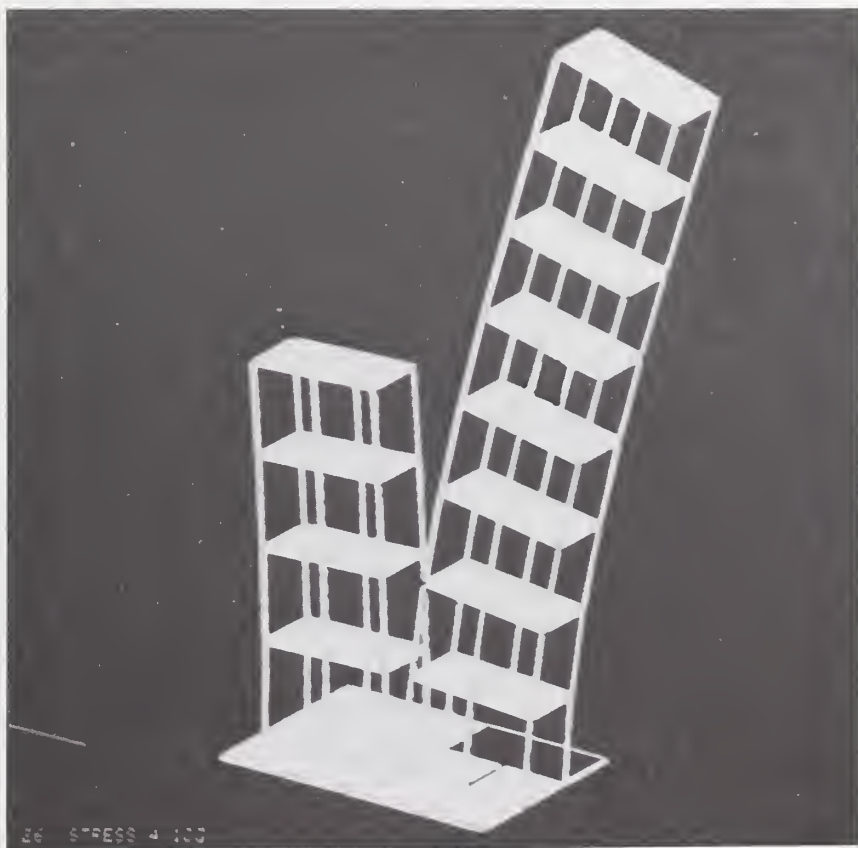
Figure 5.57. Computer simulation showing the pounding phenomenon when two buildings of unequal height vibrate out of phase.
