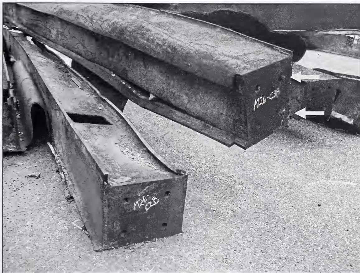
Figure 3–42. Photographic example of Type 1 failure mode for end plate connections, bolt failure. Column on right (M26-C3B) has two failed bolts remaining (arrows). Sample shown is M-26 (A130: 90-93). Damage of this type may be due to any one of the extreme loading events.
