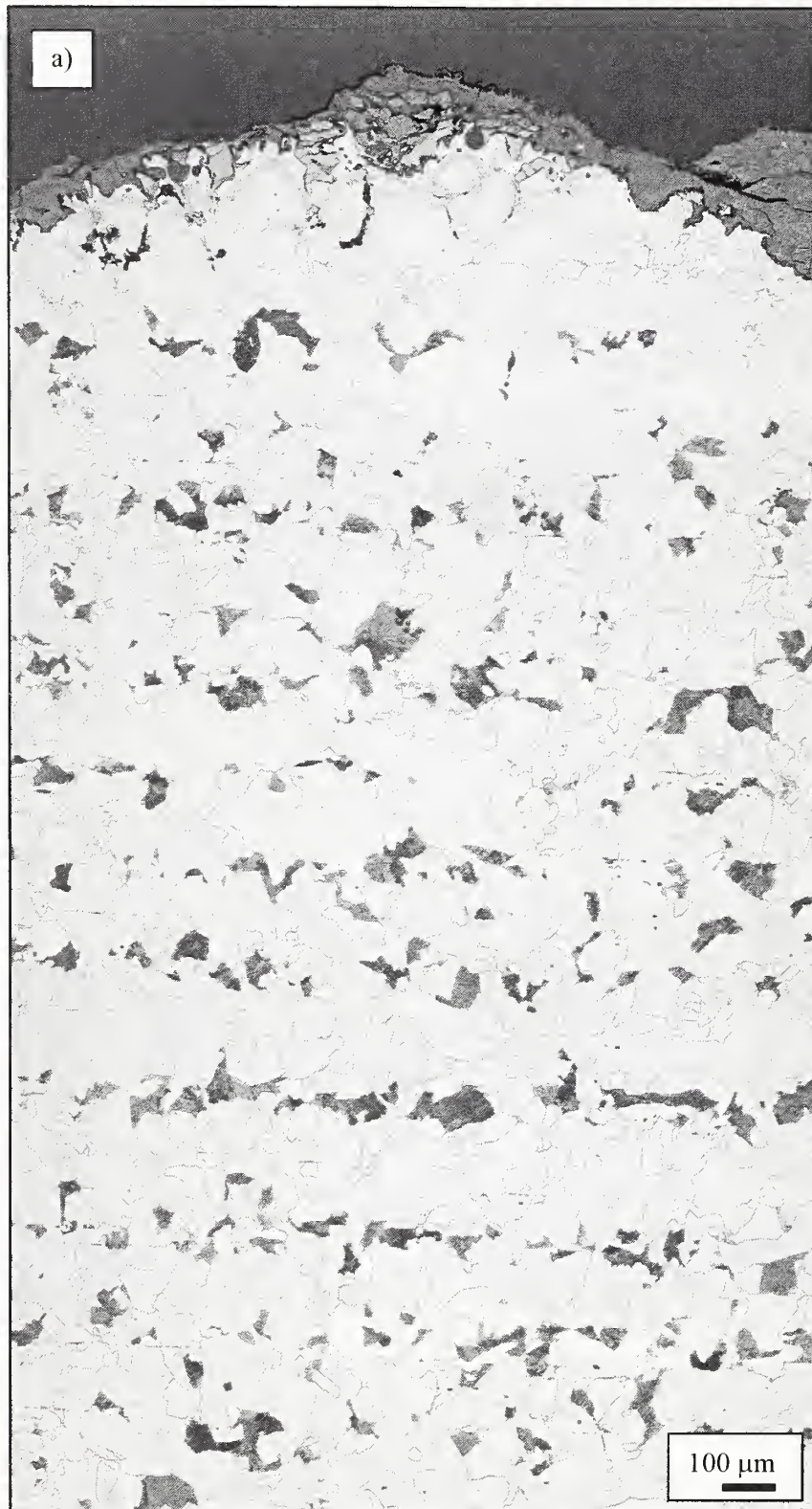
Figure 6–21. a) Light optical micrograph showing banded structure of the 50 ksi column labeled K-16 near where the extreme corrosion process occurred. As-built location was not known. Two percent nital and 4 percent picral etch.
