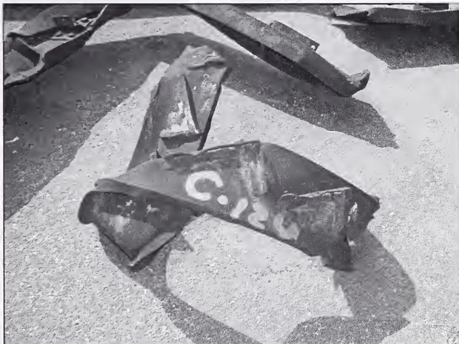
Figure 4–7. Sample C-124 from the core area, apparently used to support stairs as brackets for runs and riser were observable.
