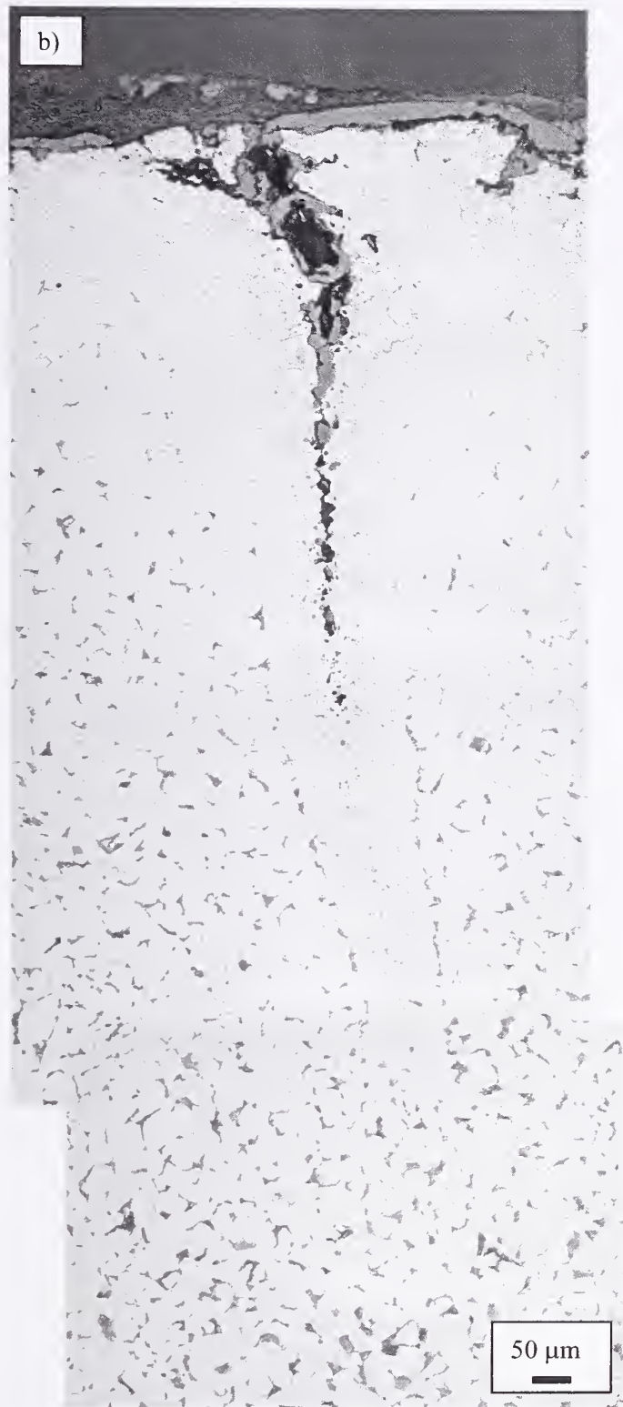
Figure 6–12. Light optical micrographs of the microstructure of a perimeter floor truss seat from the 99th floor of WTC 1, panel N-8 (A142: 97-100). b) penetration of the iron oxide phase with internal oxidation and decarburization fronts possibly due to elevated temperature exposure. Two percent nital and 4 percent picral etch (cont.).
