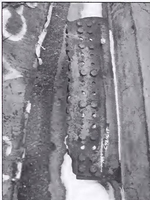
Figure 3–33. Photographic example of Type 2 failure mode for spandrel connections, bolt tear out in splice plate from C-46 (B157: 68-71). Orientation was from the outside of the building looking in. Damage of this type may be due to any one of the extreme loading events.
