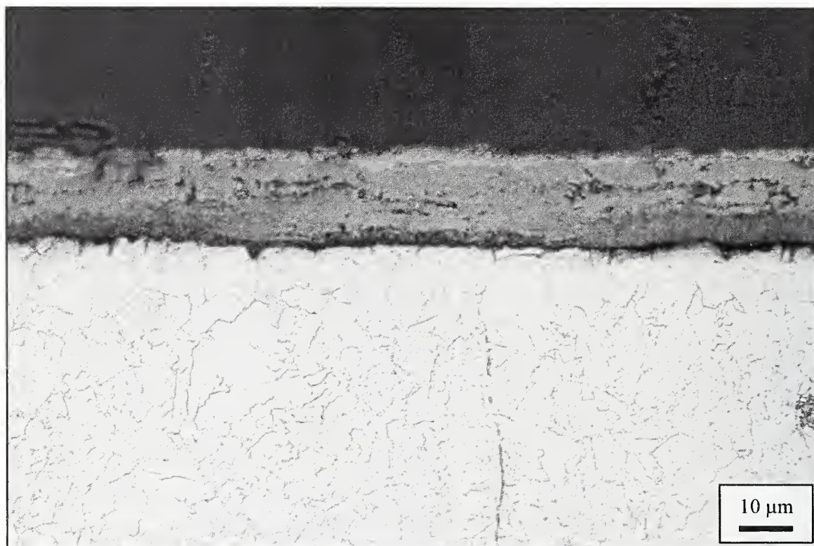
Figure 6–8. Iron oxide scale that developed on a 100 ksi quenched-and-tempered flange plate after isothermal exposure at 625 °C for 2 h. Sample was from panel C-10 (WTC 1, column 451, 88th floor). Two percent nital and 4 percent picral etch.
