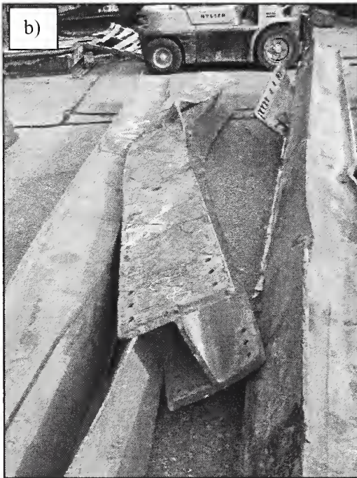
Figure 4–1. Core column C-80 (603A: 92-95) located in the impact zone for WTC 1. Damage believed to be due to collapse. a) Overall view of recovered column, b) view of connection in the 92nd floor region, failure as a result of bolt fracture, and c) torn end of column near the 94th floor region.
