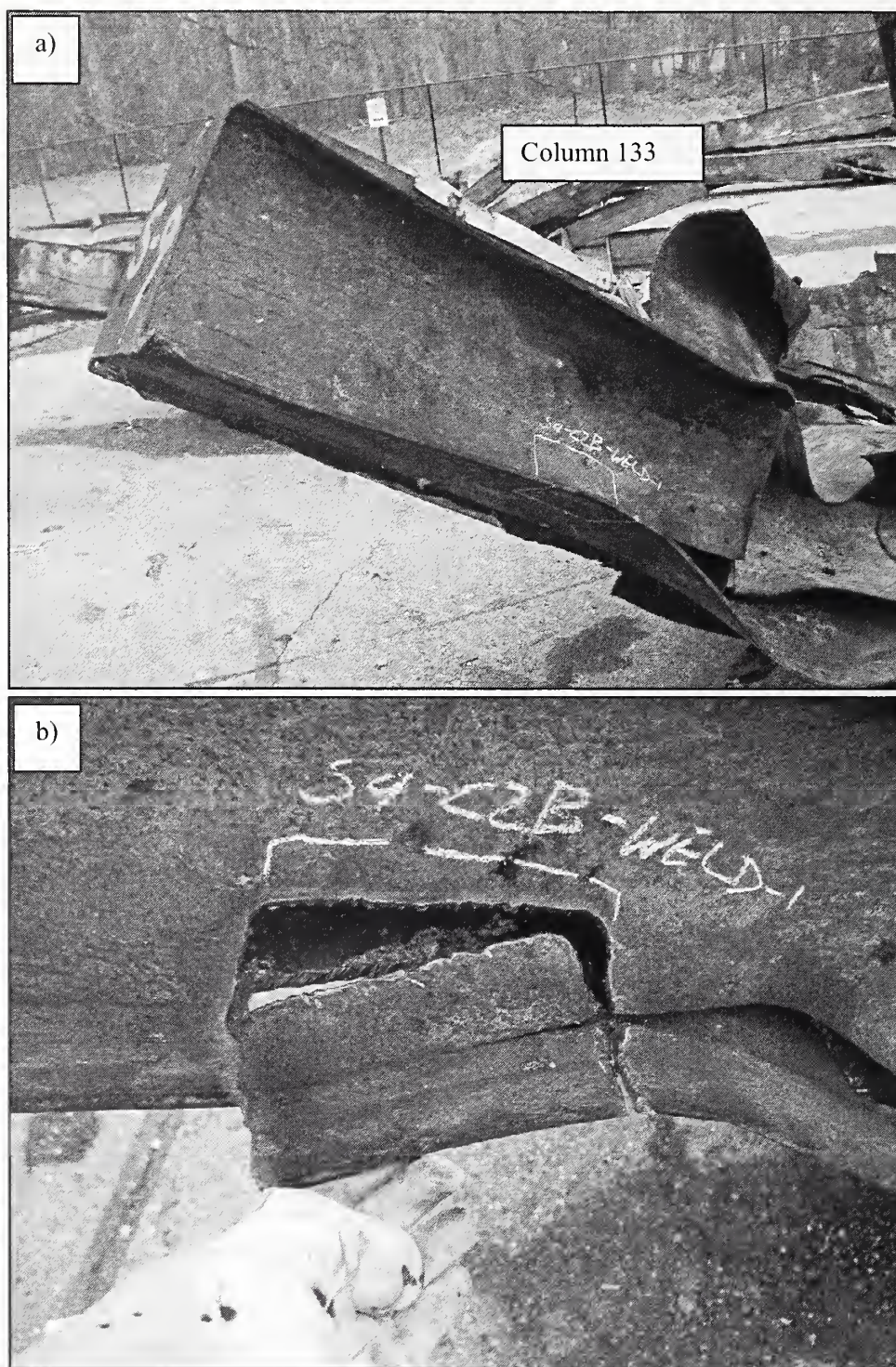
Figure 3–24. Weld fracture sample S9-C2B-Weld-1 (A133: 97-100, column 133), images taken a) prior to sample removal and b) after flame cutting. Panel S-9 was struck by the vertical tail assembly of the airplane.
