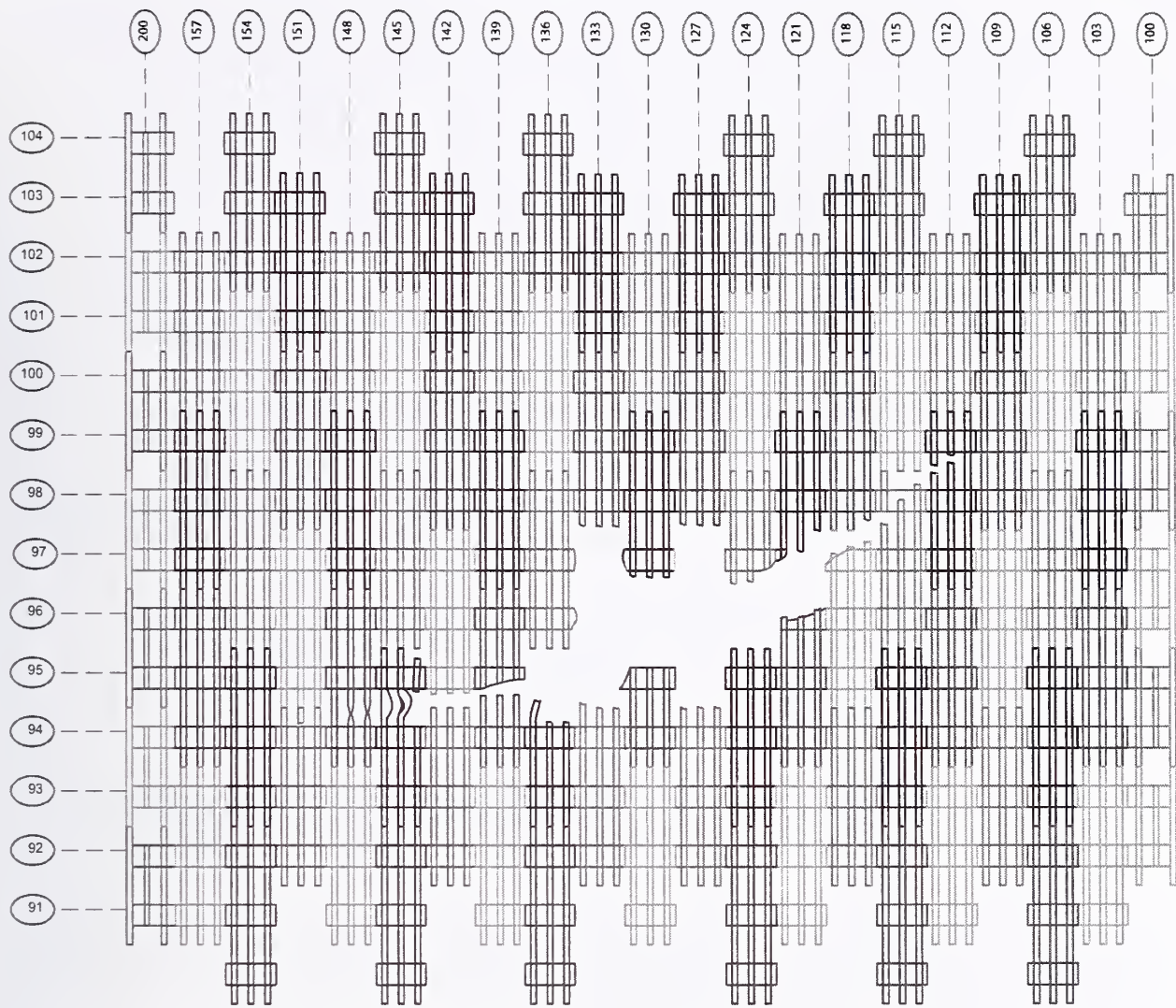
Figure 2–1. Estimated amount of damage to the north face of WTC 1, as determined by NIST.
