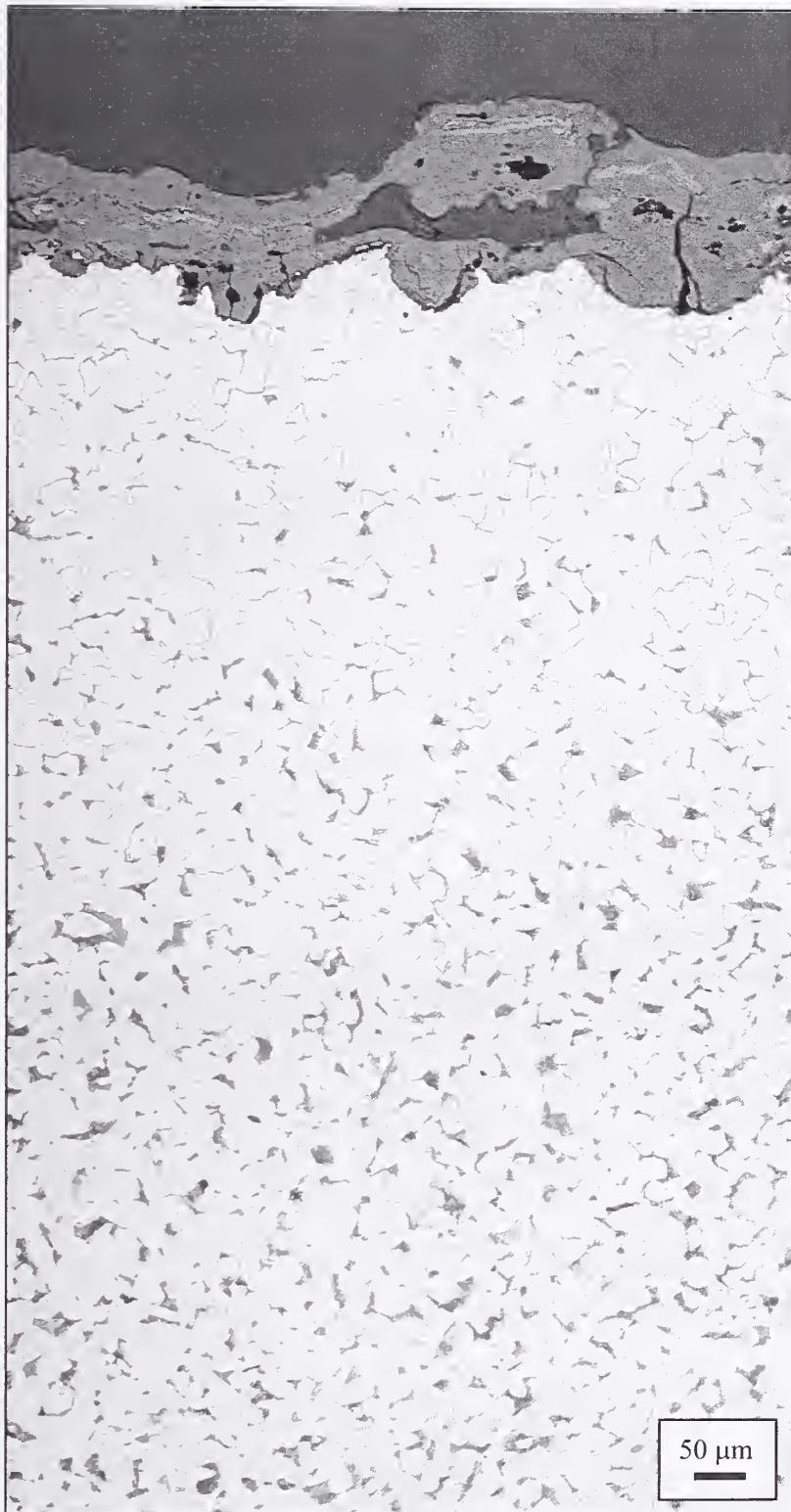
Figure 6–11. Light optical micrograph showing the partially decarburized zone found near the surface of a perimeter floor truss seat from directly above the airplane impact on the 99th floor of WTC 1, panel M-2 (A130: 96-99). Two percent nital and 4 percent picral etch.
