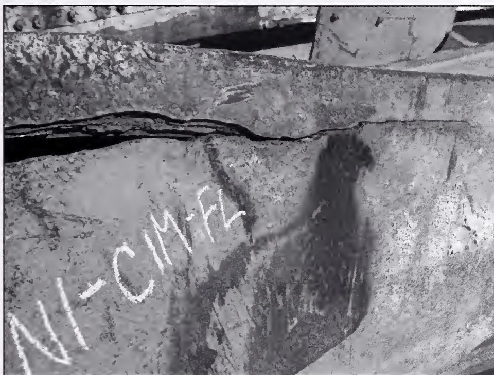
Figure 3–31. Most-likely scenario for fracture associated with weld if second crack of sample S9-C2B-Weld-1 had continued to propagate through the flange plate. Sample shown is from N-1 (A218: 82-85). Damage most likely occurred during the collapse of WTC 1.
