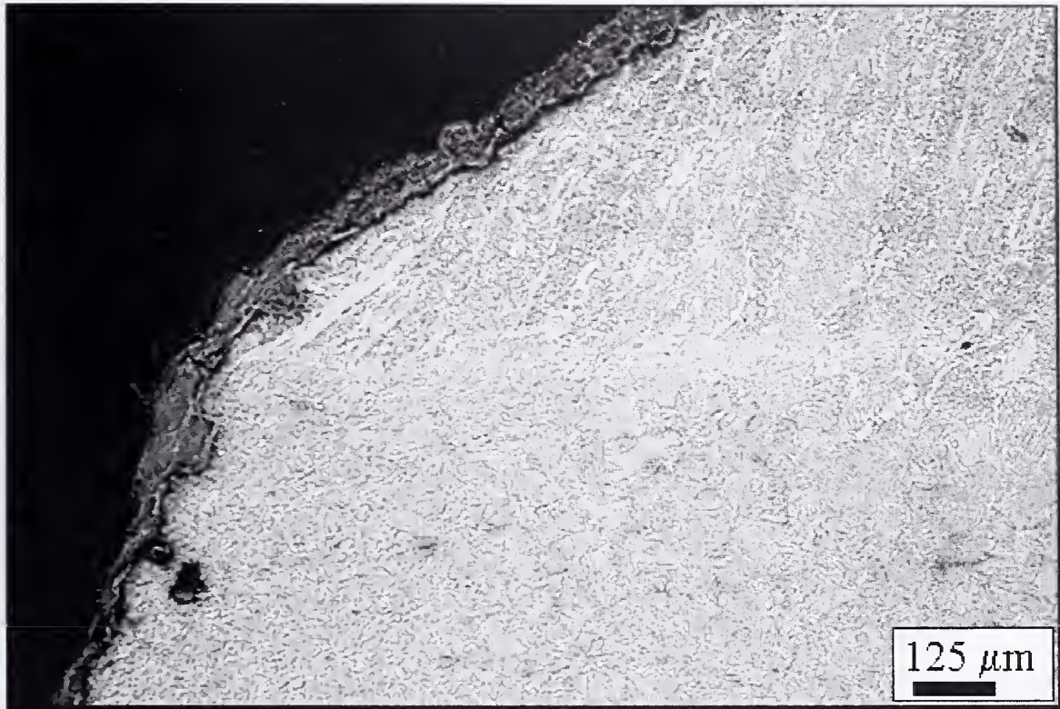
Figure 3–17. Light optical micrograph b) at higher magnification (red box in [a]) showing initiation of fracture at the toe of the weld and traveling through the HAZ of the plate. Two percent nital and 4 percent picral etch. (A130: 96-99, column 129)
