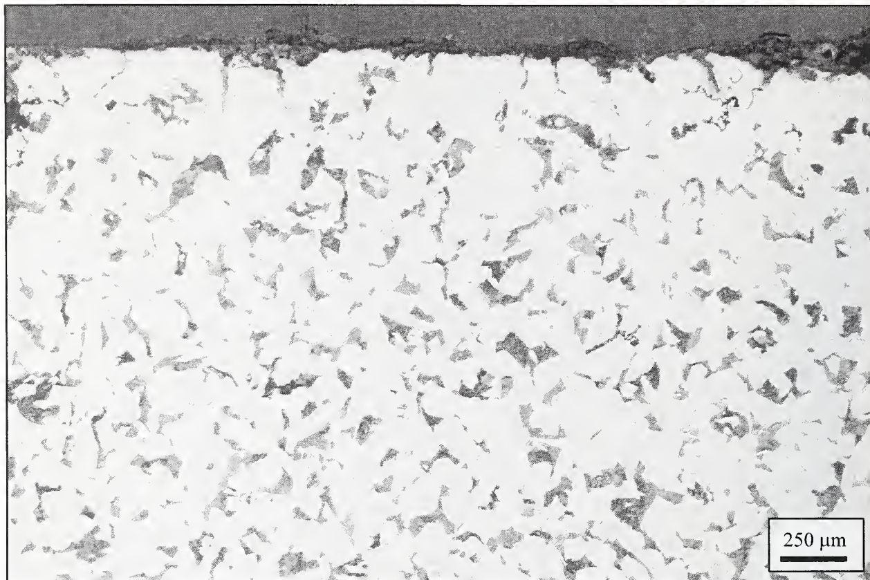
Figure 6–27. Light optical micrograph showing the structure of corrosion scale formed on sample C-115. A decarburization zone was not observed. Two percent nital and 4 percent picral etch.
