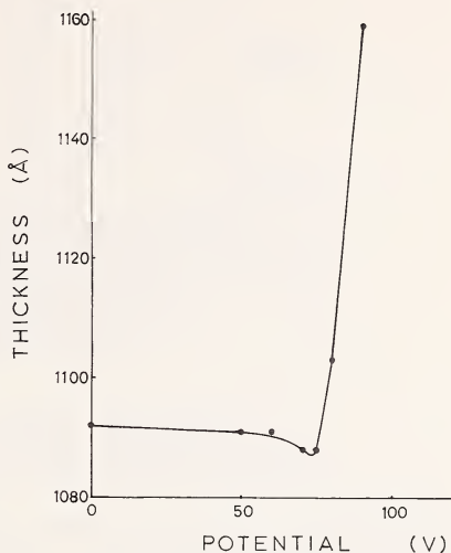
FIGURE 9. Thickness curve for the determination of the voltage for re-anodisation for aluminium anodized previously at 80 V.
