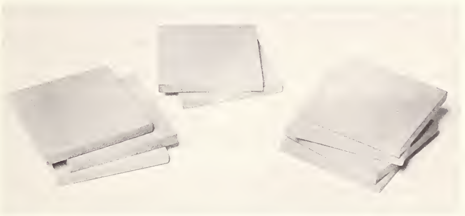
FIGURE 2. The meter-board can be disjointed and stacked up to make a liter-cube, or parts of one. The pieces are held together in the form of a board or cube by magnets or by dowel pins. Note: Each piece of the meter-board/liter cube has its mass adjusted to exactly 100 grams, so that the whole has a mass of one kilogram. It is packaged in a clear plastic container which is graduated at 100-milliliter intervals. It is a most instructive experiment to measure out a liter of water and discover that its mass is one kilogram.
