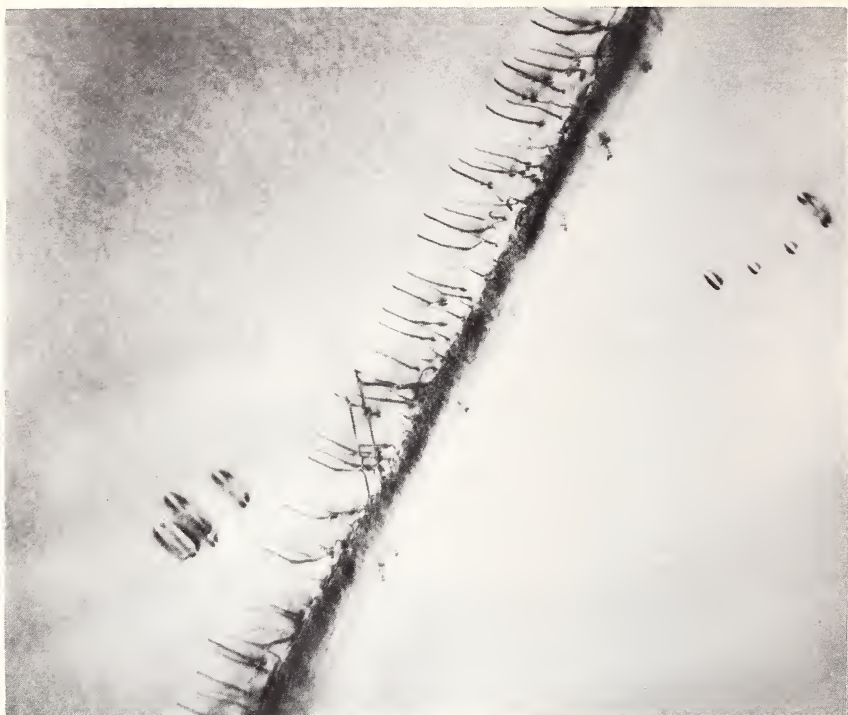
A transmission electron micrograph showing dislocations under a single scratch on the (0001) basal plane surface of an aluminum oxide single crystal. The scratch and its associated damage illustrated here is typical of that produced by mechanically polishing aluminum oxide with a fine ( \frac{1}{4} micrometer) diamond abrasive compound. Magnification = 37500 \times .
