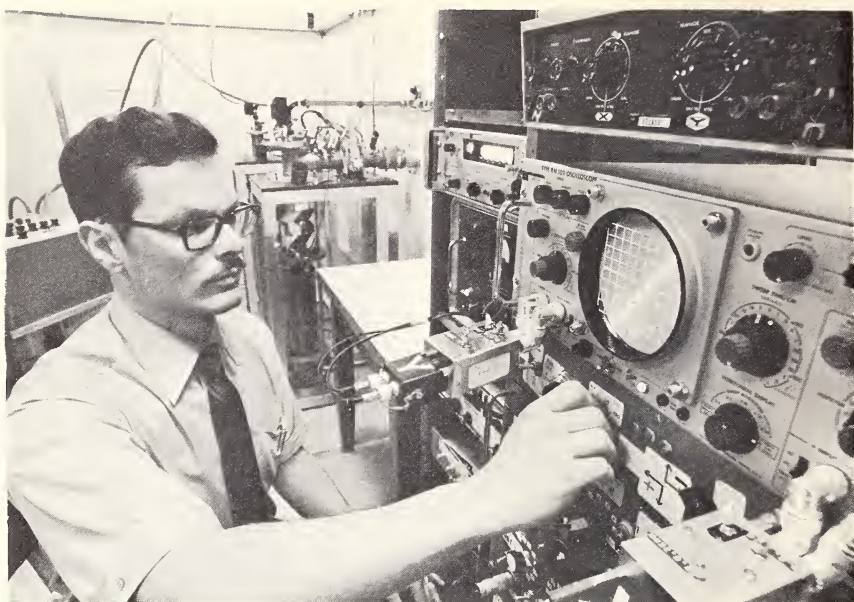
Comparing the voltage produced by a Josephson junction when exposed to microwave frequency to that of a standard cell.
