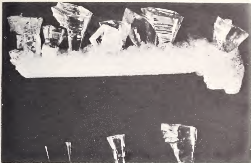
Single crystals of ultra-pure aluminum oxide. The crystals shown at the bottom illustrate the stages of growth beginning with a "whisker" seed weighing 0.002 gram at the left and ending with a crystal weighing 4.411 grams after approximately 40 hours of growth. At the top a group of crystals is shown attached to the aluminum oxide support used during the growth cycle.
