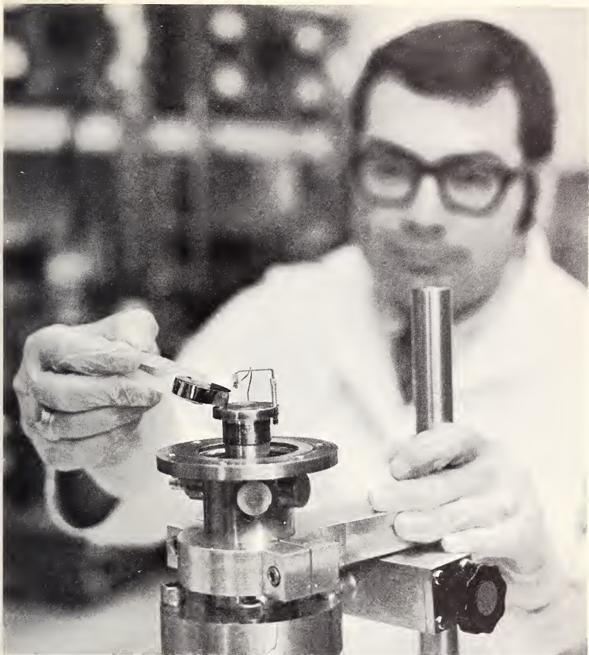
A wafer of germanium is mounted in a cryostat for measurement of its performance as a radiation detector.
