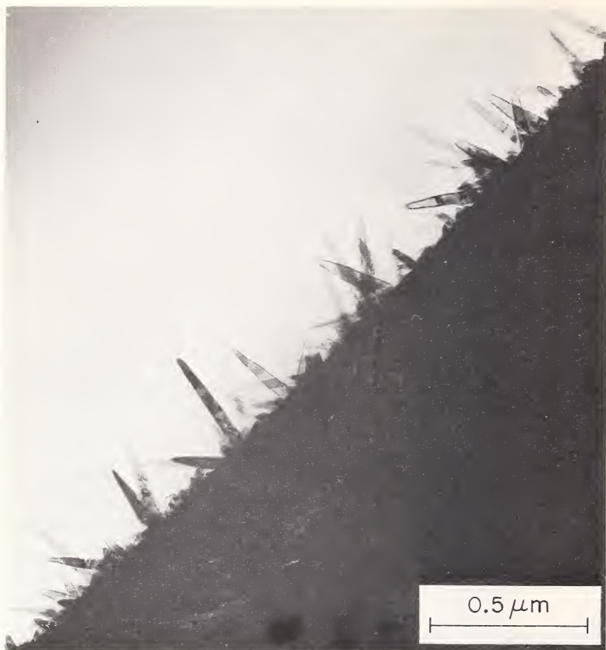
A transmission electron micrograph showing \text{TiO}_2 (anatase) crystals protruding from a titanium alloy after corrosion at 200 °C.
