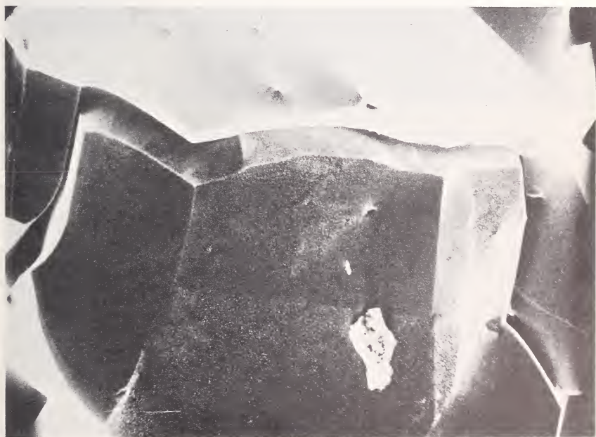
A scanning electron micrograph of intergranular fracture in a Cu 95/Pd 5 alloy. The alloy was exposed to a 3.5 percent sodium chloride solution at room temperature for several weeks.
