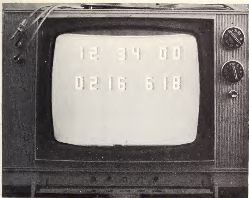
Conventional TV receiver and associated decoder displays time-of-day on picture-tube face in hours, minutes, seconds format on top line and time difference on the bottom line.
