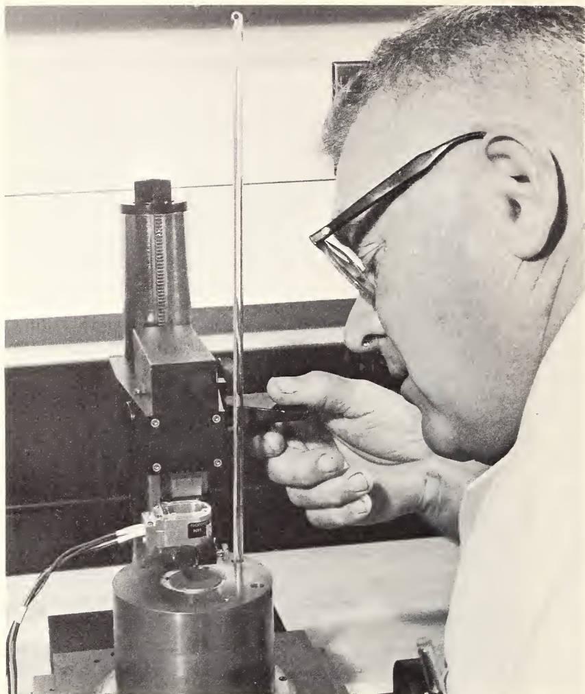
The four-point probe holder has greatly improved resistivity measurements and minimized damage to specimens.
