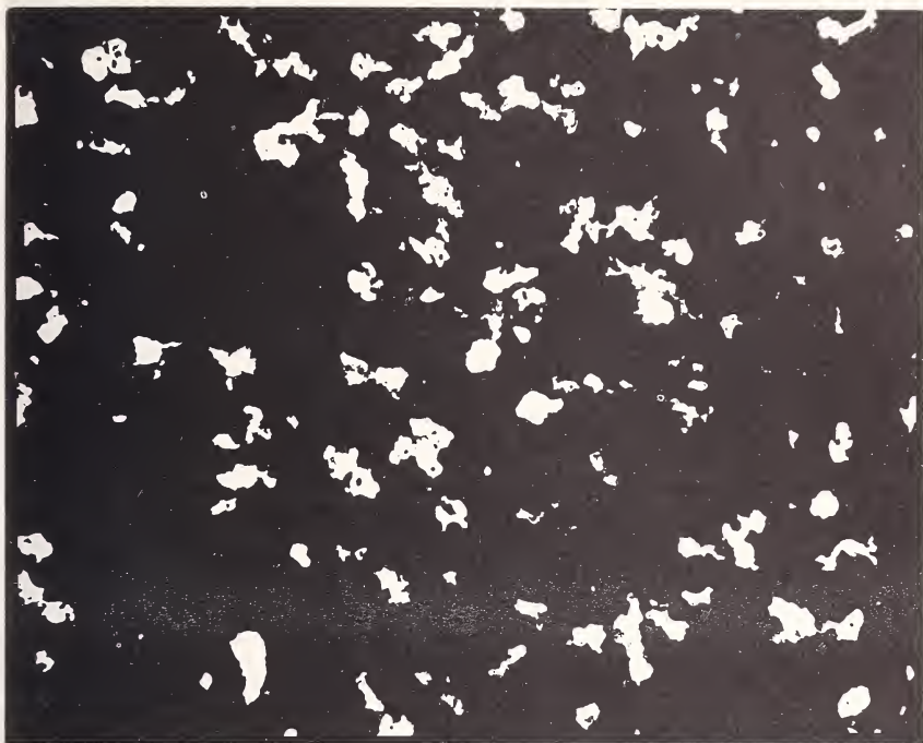
An optical micrograph of nominal 10 percent austenite in ferrite matrix. \times 25 . Measurement on the NBS scanner determined the austenite (white) phase area to be 9.96 \pm 0.03 percent.
