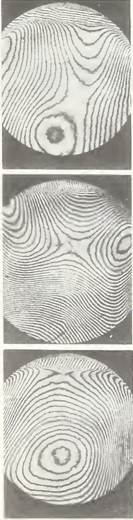
Figure 8. Typical topographs of silicon slices. On the right-hand side of the reference flat the aluminum support is visible, which also reflects.
