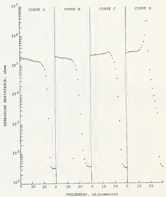
Figure 6. Effect of Time Delayed Dopant Injection on the Interface Between an N + Substrate and an N-type Epitaxial Layer.
