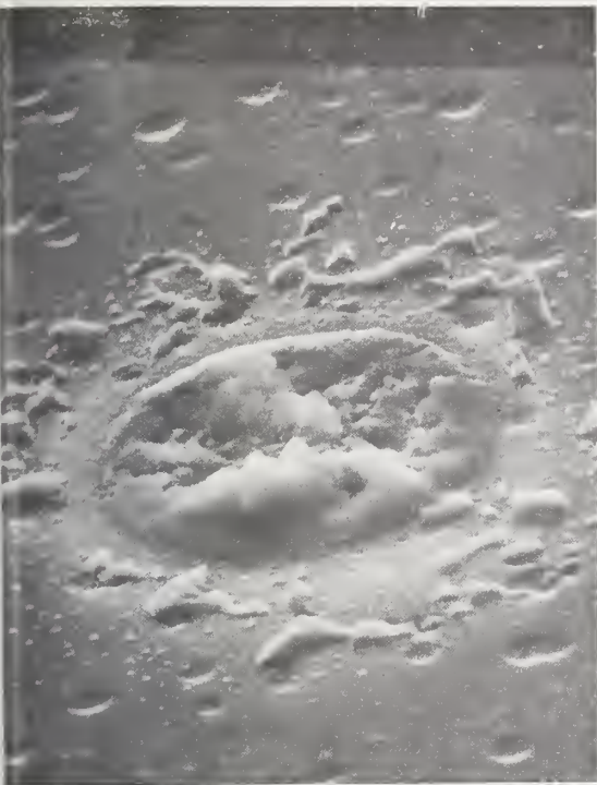
Figure 1. Scanning electron micrograph of a spreading resistance probe impact area on silicon. Magnification 10,000 X; 70° specimen tilt.
