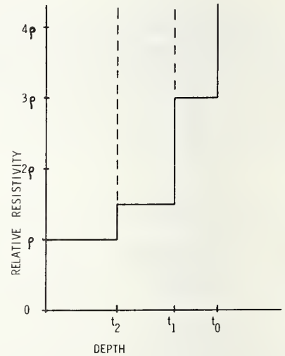
Figure 4. Resistivity profile resulting from the superposition of three layers of different thickness but uniform resistivity 3\rho .
