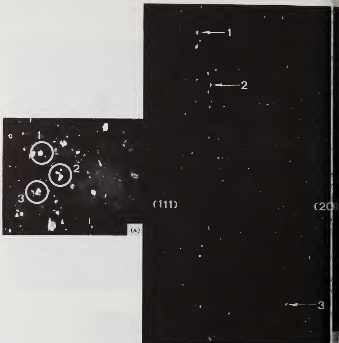
Figure 3. Outward tracing of reflection images of Fig. 2b. (a) 2.5 mm from specimen surface. (b) 27.5 mm from specimen surface.
