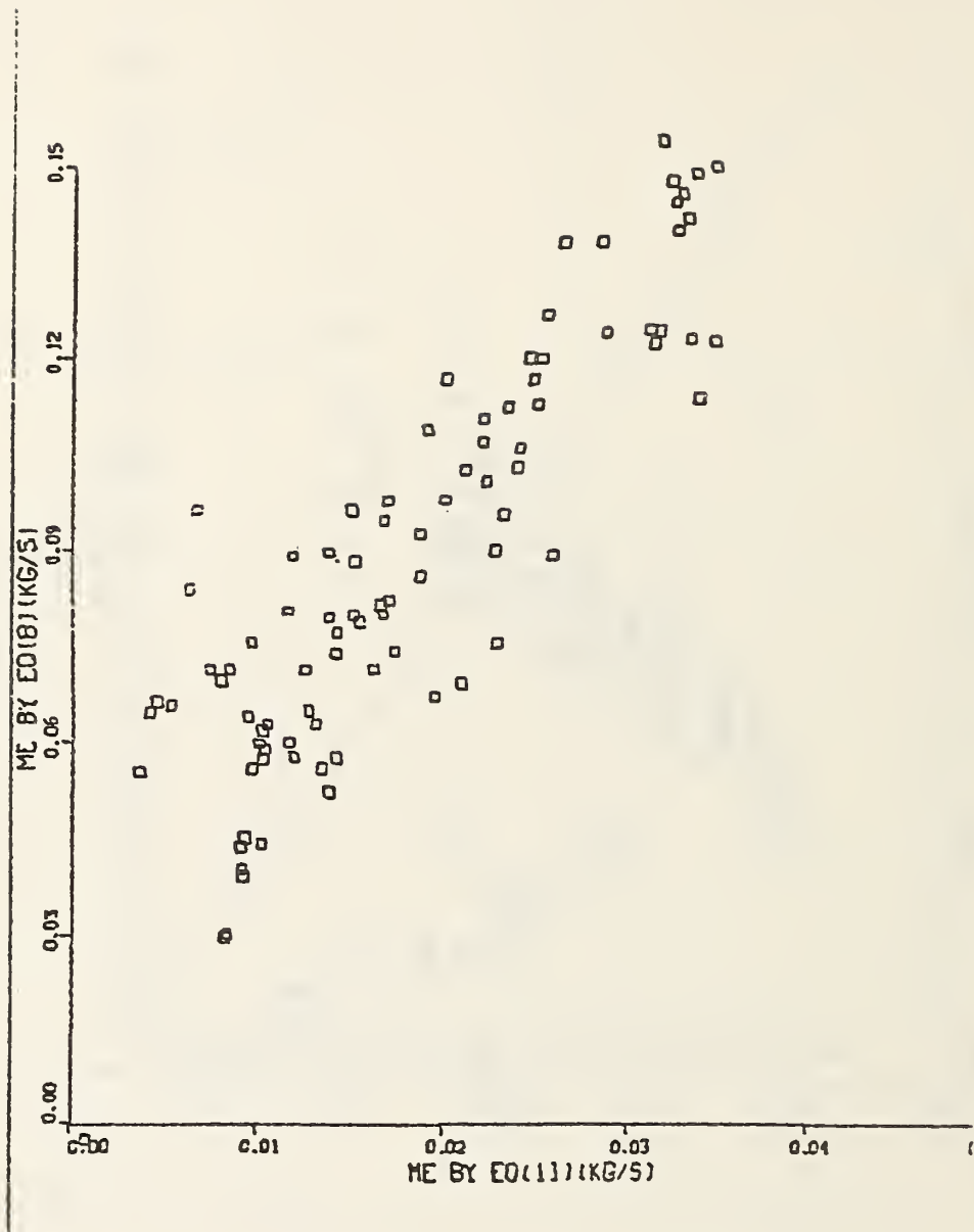
Figure 8. Comparison of vent mixing flow rates by two methods
