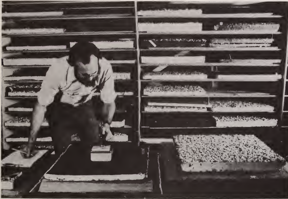
Evaluating equipment for detecting moisture in roofing insulation.
