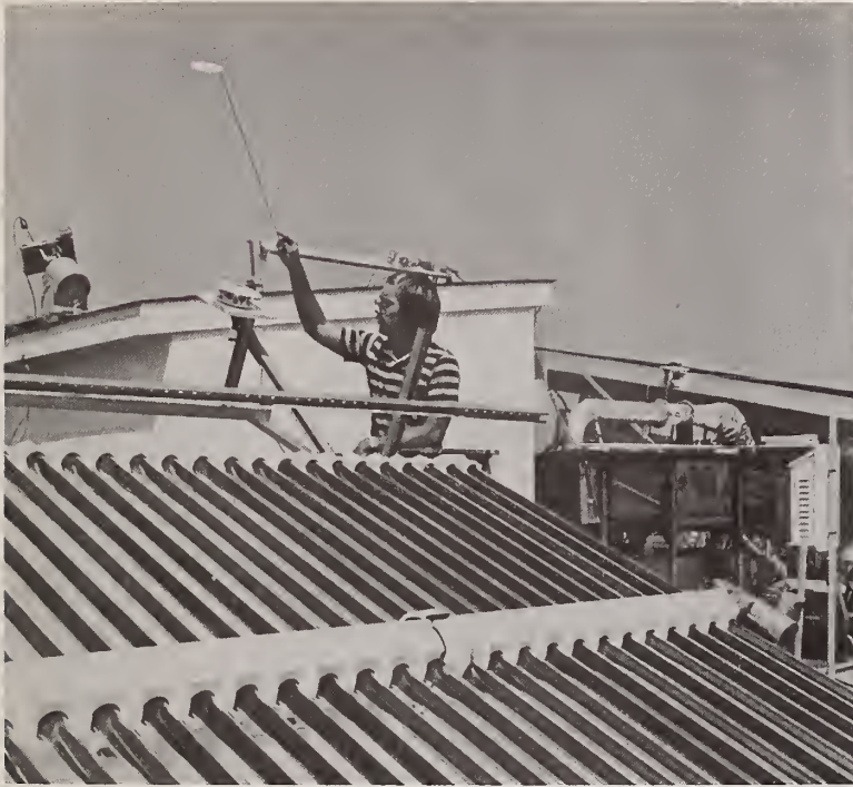
The performance of an evacuated tube collector is being monitored to develop test methods for solar collectors.
