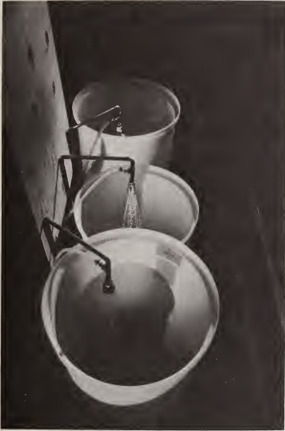
Shower heads are being tested to develop criteria and test methods to reduce water use.
