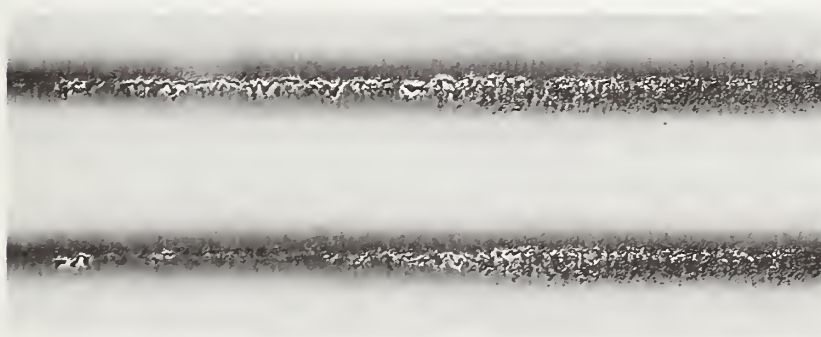
MOIRE FRINGE PATTERN USING 500 LINE/INCH RONCHI RULINGS
