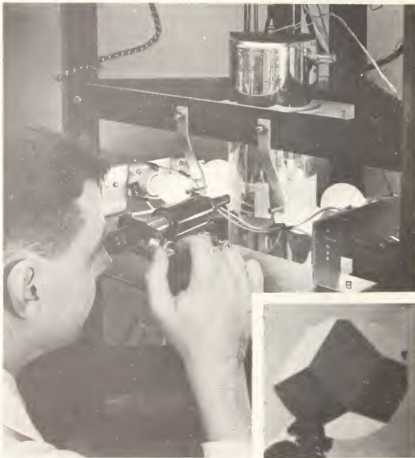
A measuring microscope is used to measure the distance between two faces on a potassium crystal growing from the vapor phase inside a dewar vessel. Inset shows potassium crystal about 0.9 mm in diameter. Studies of fundamental crystallization processes in metals provide a better understanding of the physical properties of the materials (page 92).
