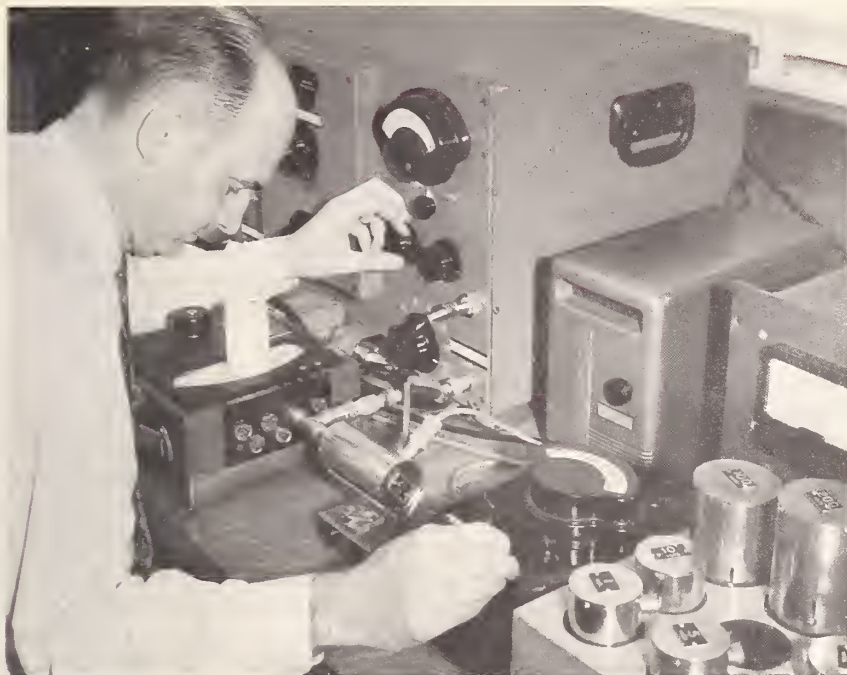
Finding the frequency response of a differential thermocouple voltmeter. This instrument is a recent contribution to the solution of the problem of transfer from d-c and a-c measurements at power and higher frequencies (page 38).
