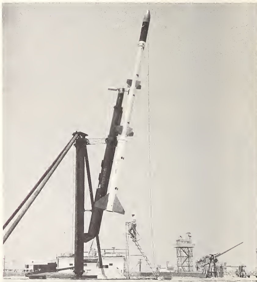
Javelin rocket which carried an ionosonde to an altitude of 1,000 kilometers. For thirteen minutes, the ionosonde made topside soundings of the ionosphere. The experiment was made to test the sounding system for the fixed-frequency satellite topside sounder to be orbited in 1962 (page 127).
