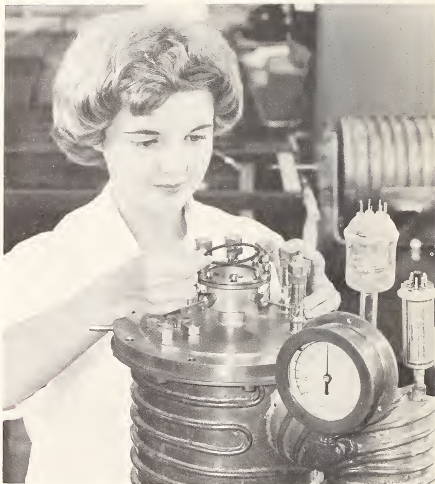
As part of an effort to extend the range and accuracy of temperature measurements, the thermoelectric properties of high-temperature thermocouples such as tungsten-rhenium and tungsten-iridium are studied in this experimental tantalum tube furnace. Operating temperatures of 2,000 °C and higher are obtained (page 51).
