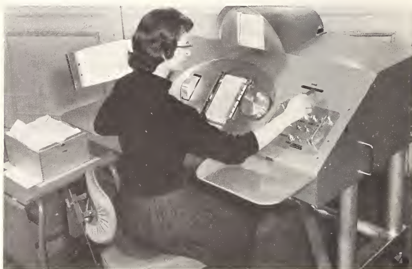
Microcite , a close-coupled searching machine developed for use with the NBS punched-card (peek-a-boo) instrumentation index. The operator can locate references, view abstracts on the screen at the top, and make copies of the selected abstract automatically (page 123).
