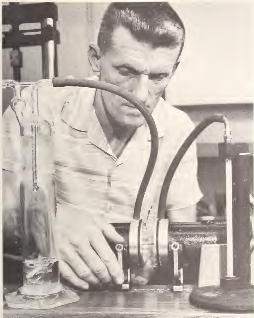
Rotating beam fatigue-testing equipment used to study the effect of various components of the atmosphere on the fatigue properties of metals. Studies in controlled atmospheres show that fatigue is profoundly affected by the environment at the surface of the metal (page 98).
