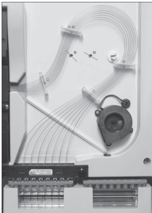
Sixteen capillaries enable high DNA throughput, allowing more samples to be simultaneously analyzed. © 2002 Robert Rathe
