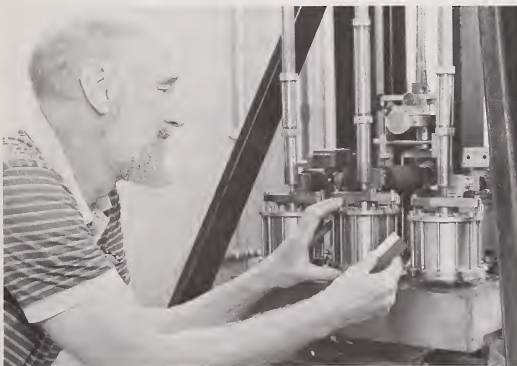
NBS physicist James Schooley prepares to place a gauge block to preset the manometer system of the NBS gas thermometer, the most accurate instrument of its type in the world.
