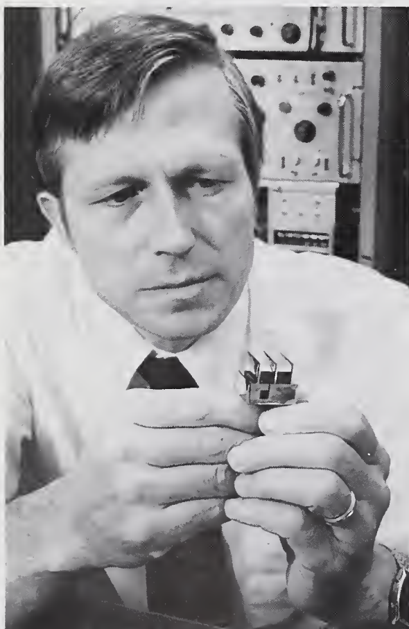
NBS physicist Albert Henins holds carefully cut silicon crystals used to precisely measure silicon-crystal lattice spacings.
