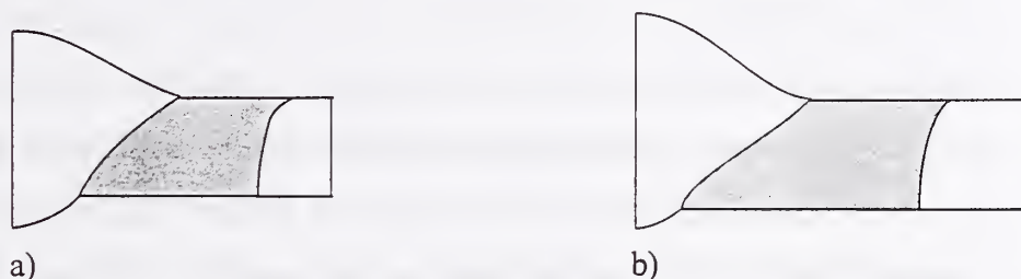
Figure 2: Comparison of welding experiment and its simulation for pulsed MAG welding, butt weld (thickness 2 mm), D_w = 1.2 mm, Z_K = 15 mm, I_G = 40 A, U_p = 35,5 V, CORGON 18 a) v_w = 7,1 m/min, f_p = 175 Hz, v_w = 1.31 m/min, b) v_w = 4.4 m/min, f_p = 100 Hz, v_w = 0.91 m/min
