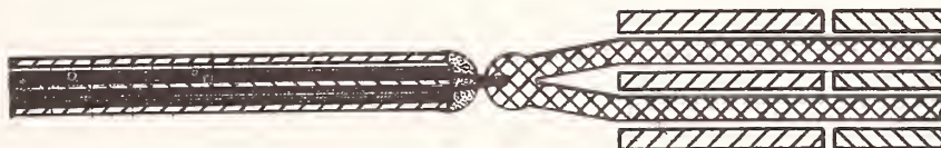
FIGURE 3. Arrangement to assure good thermal contact between the junction of a base-metal thermocouple and that of a protected platinum versus platinum-rhodium thermocouple.
